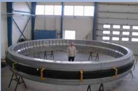
Developing fabric expansion joint solutions with a significantly longer life cycle and affordable replacement - here for a MHI 701F gas turbine.
