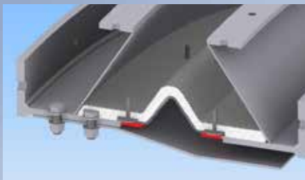
3. Fitting of KE-Pulse Barrier.
