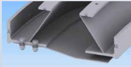
1. Removal of A-style expansion joint including external and internal insulation, wire mesh, back-up flanges and pre-bolster.
