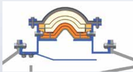
Ex. 1: Fabric EJ with gas side bolster and horizontal mounted flanges.
