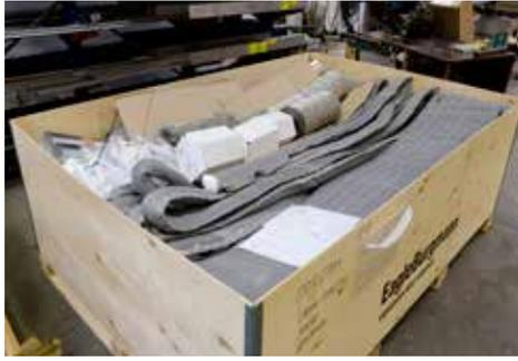
EagleBurgmann can replace fabric expansion joints, eg. EE-00, EE-01, EE-02, EE-03, EE-04 and IE-01 in exhaust systems behind all generations of M251, M501 and M701.
