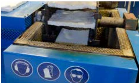
EagleBurgmann is testing a variety of fabric materials. Upgrading materials will improve life cycle. Low cycle fatigue (LCF) test rig.
