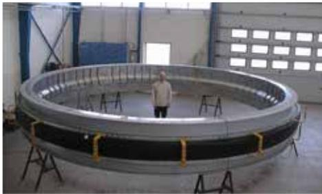
Large diameter expansion joint for a MHI 701F gas turbine.
