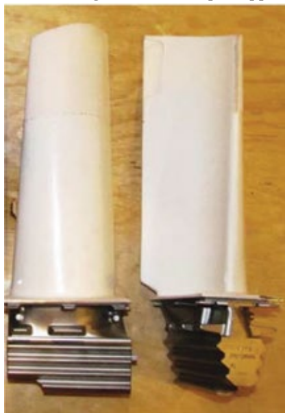
11. Extended coating protection made parts more durable, reduced fallout
