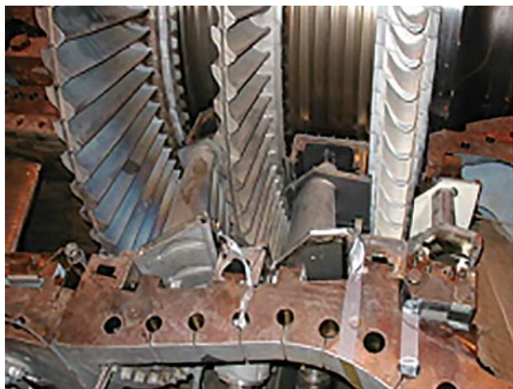
3. Turbine section of a Frame 6 illustrates three-stage arrangement (left). Arrow in photo of first stage at right points to where firing temperature is calculated (not measured)
