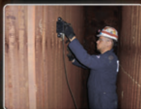
OD Scanning for Tube Wall Thickness
