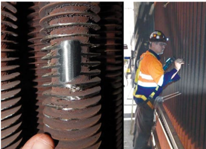
3. Superheater tube is prepped for ultrasonic NDE
