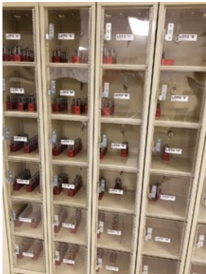
5. LOTO boxes hold keys associated with clearance isolation locks. Labeling matches up with notations on the job status board
