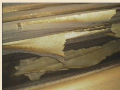
3, 4. Field turn insulation migration —end turn at left, slot turn at right—came into view in 2007
