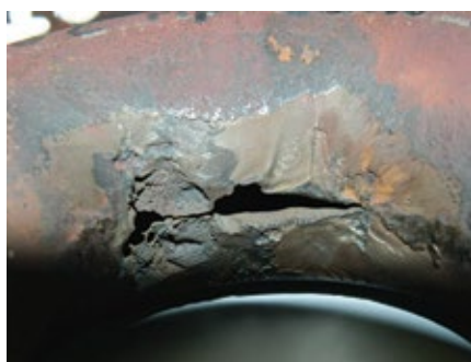
5. Failed return-bend economizer tube is at left, an active leak at right
