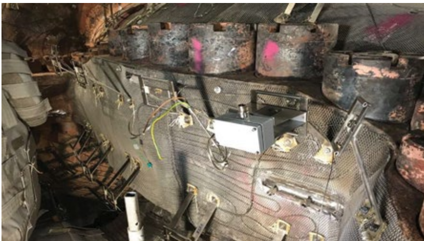
5. Removable heating blankets on the split line and above it facilitate maintenance and minimize insulation wear and tear
