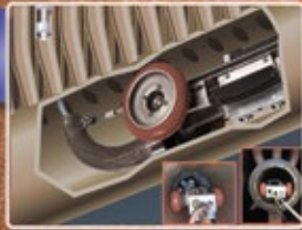
Internal Crawler for Visual and Tube Thickness from the Tube ID
