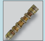
Varnish on valve spool
