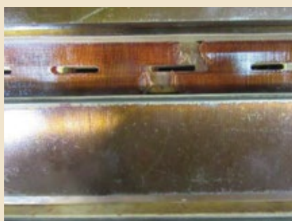
3, 4. Field turn insulation migration —end turn at left, slot turn at right—came into view in 2007
