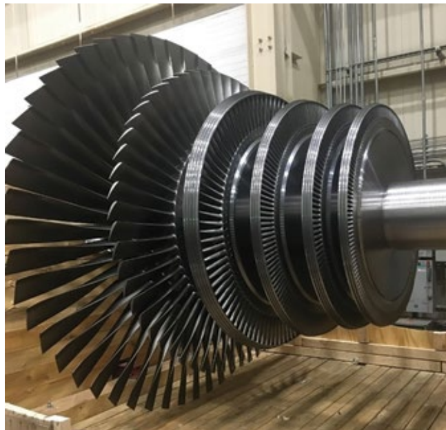
5, 6. New HP steam turbine rotor and barrel assembly is at left, new LP section at right
