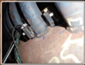
Internal Crawler for Visual and Tube Thickness from the Tube ID
