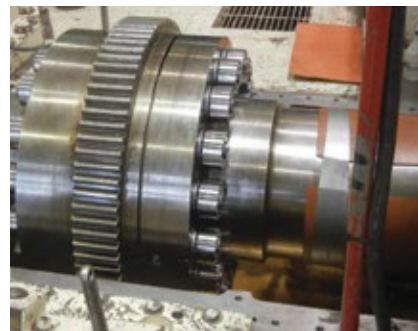
12, 13. EzFit coupling bolt avoids fitted-bolt seizure issues (left), eliminates slippage during operation (right)
