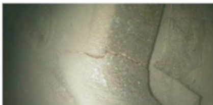
6-8. Inspection results: Field pole crossover cracking (left), phase-to-phase failure (center), bottom-bar insulation damage
