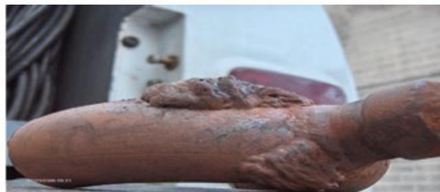
**4. Six different weld-repair styles** kicked off Bremco's tube-repair clinic, after the audience gasped at photos of the ugly, uglier (left), and ugliest (right) welds in service
