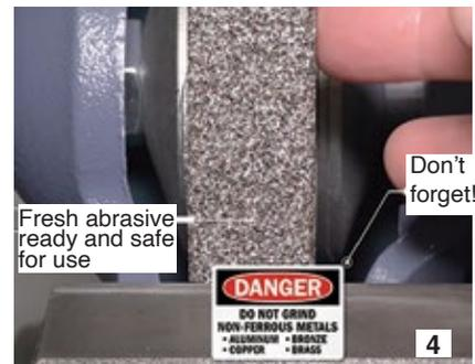
1 – 4. Non-ferrous metal fouling is observed on grinder wheel in Fig 1. Dressing is illustrated in Fig 2 and in close-up in Fig 3. Job is complete in Fig 4
