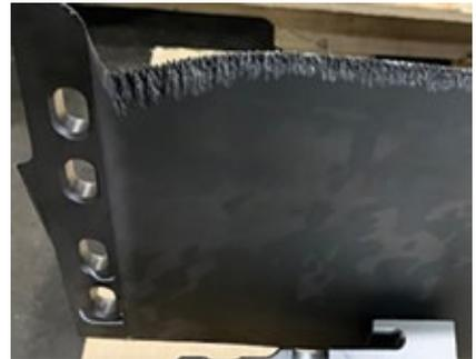
**11. Excessive leading-edge erosion** often is identified with 40-in. L-0 titanium blades installed in many steam turbines
