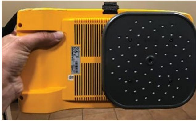
**1. Sonic leak detector** relies on an array of 64 digital mics to locate the source of the sound
