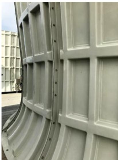
**2. New stacks** have hardware on the outside, making for easy maintenance access
