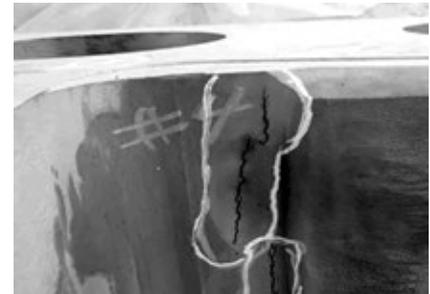
**2. Cracks of significant length and depth** at this turbine's HP inlet were ground out and weld-repaired
