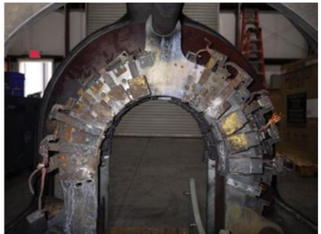
6. The outboard collector ring (at right in left photo) and associated brush-rigging components suffered severe arc damage. The outboard collector ring as viewed from the brush rigging is in the right-hand photo
