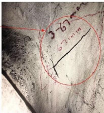
This 1980s-vintage unit for a 618-MW site had logged 220,000 hours and 328 starts. Material of manufacture is GS17CrMoV5-11 (1.7706). Operating conditions are 4.3 MPa at 330C to 430C.
