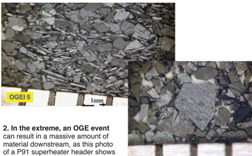
2. In the extreme, an OGE event can result in a massive amount of material downstream, as this photo of a P91 superheater header shows
