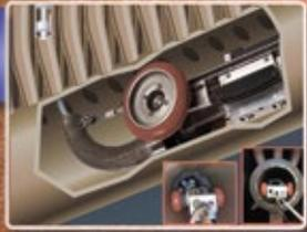
**Internal Crawler for Visual and Tube Thickness from the Tube ID**
