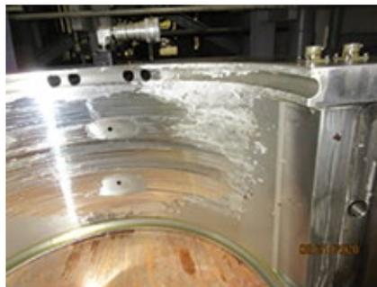
**5. Bearing electrolysis damage** and a broken shaft grounding brush were revealed during an inspection to determine the cause of high vibration
