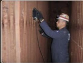
OD Scanning for Tube Wall Thickness
