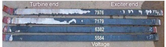
**8. Voltage is an integral factor for corona as the photo indicates.** Elevated temperature acts to further promote the phenomenon. The higher the voltage and the closer corona attack is to the turbine end of the generator, the greater the damage, as evidenced by the amount of "bleaching" in the photo
