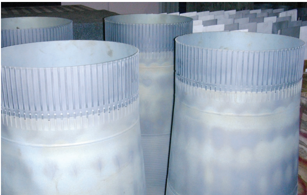
4-3. Heat tinting of liners should confirm that all coating has been stripped
