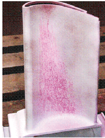
4-1. Dye-penetrant testing reveals coating cracks
