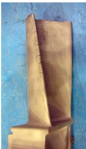
2-4. Visual inspection alone sometimes can identify parts that cannot be repaired—like this Frame 7 bucket (left)
