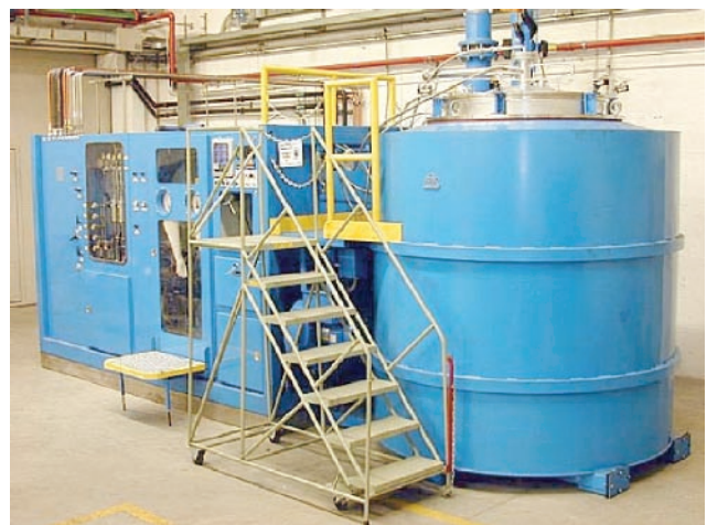
5-1. Fluor ion cleaning is one of the methods used to prepare components for brazing
