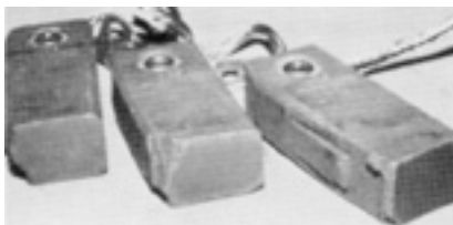
2. Brushes suffer excessive wear and breakage when the collector film does not adequately lubricate the contact surface between them and the collector ring
