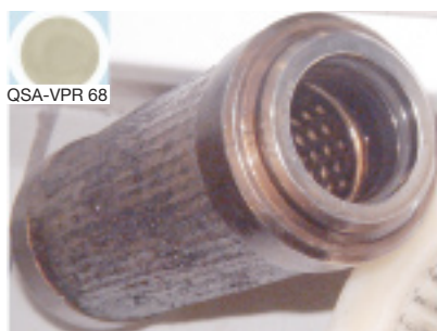
2, 3. The positive impact the CRV Plate has on varnish mitigation is easy to see by comparing the two photos of the filter for a fuel splitter valve. At the left, note the extensive fouling prior to installation of the CRV Plate. Replacement filter at right has 3000 hours of operation on the same oil after the CRV Plate was installed
