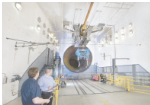
2. Engine test cell at Chromalloy's San Diego MRO shop can accommodate the LM2500
