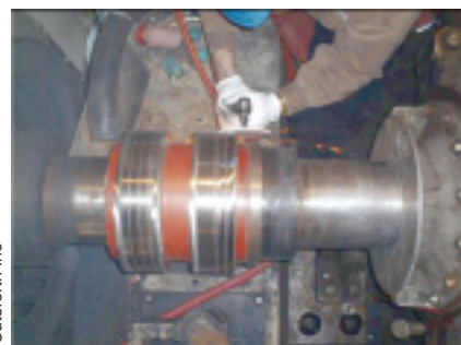
9. Spiral grooving is re-established when ring wear dictates. It can be done with the field in place
