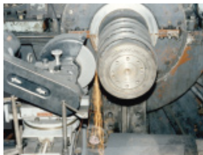
7. Objective of grinding collector rings on turning gear is to get the collector ring round
