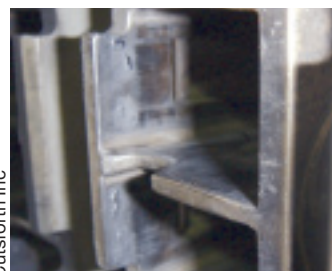
4. Buildup of carbon inside the brush box can restrict brush movement
