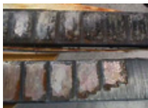
4. Stator bars , undamaged in the vent duct area, show the effects of spark erosion further into the machine
