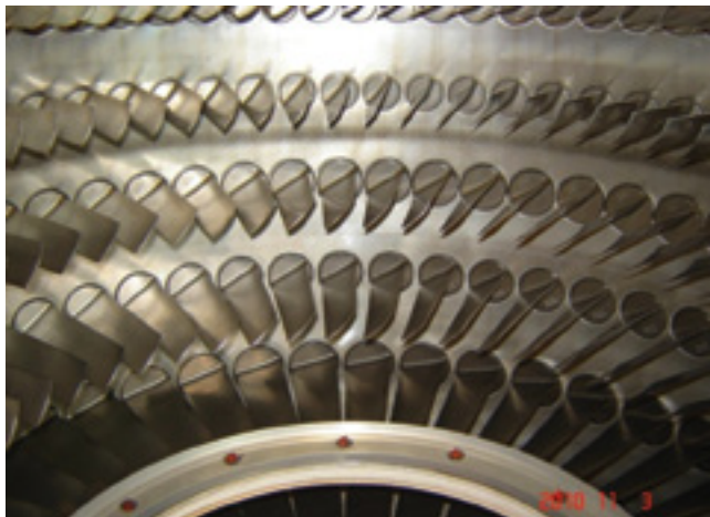
1, 2. After 4300 hours of operation with HEPA filters in the gas turbine inlet and no water washes, the airfoils in the upper stator case of the Kerrobert LM2500 (left) and the first four stages of its HP compressor (right) remained pristine
