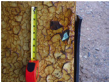
9. A test paper impregnated with potassium ferrocyanide placed on the exposed steel indicates with its blue color change that the contamination is from nonvisible soluble salts
