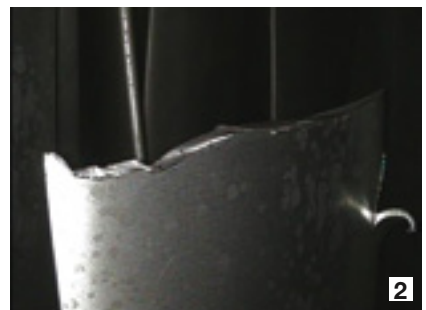
1, 2. S1 vane tip liberation at the 6 o'clock position caused extensive compressor damage in early March 2012
