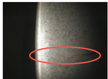
3. Crack in S1 stator vane was found in the lower half of the unit in early April 2012
