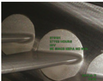
3, 4. A borescope inspection after one year of operation on HEPA filters, showed the bellmouth and visible stages of the HP compressor for the Windfall G4 were “like new”
