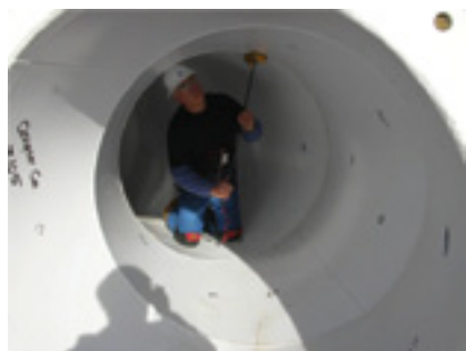
7. Inspecting a cooling-tower riser with a low-voltage holiday test is relatively easy inside pipes 54 in. and larger; more difficult in smaller pipes
