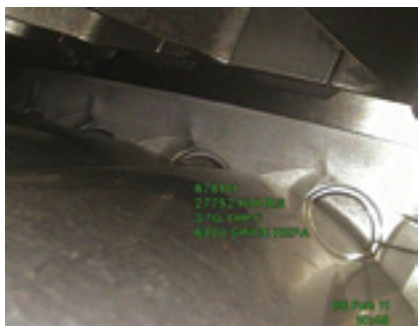
3, 4. A borescope inspection after one year of operation on HEPA filters, showed the bellmouth and visible stages of the HP compressor for the Windfall G4 were “like new”
