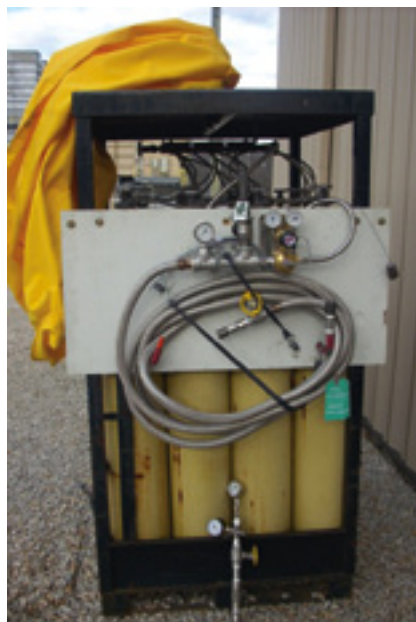
9. System for maintenance purging of natural gas is relatively simple
