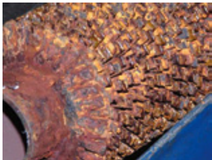
7, 8. HRSG tube condition before (left) and after (right) CO 2 blasting
