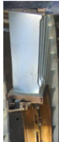
7, 8. Root spring forces the blade out into the running position and eliminates wear attributed to operation on turning gear
