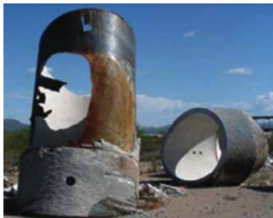
2. Trailing prestressing wires, the pipe displays hole blown by internal pressure (above)
