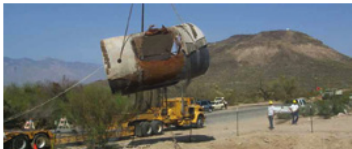
2. Trailing prestressing wires, the pipe displays hole blown by internal pressure (above)
