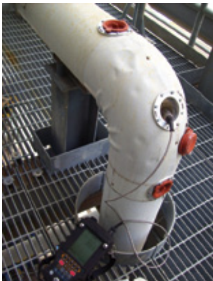
3. Elbow in boiler-feed pipe is UT-checked for wall thickness
