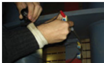
3. Vent duct allows access for inspection and testing. Here, contact coefficient probes are inserted into the back of the core
