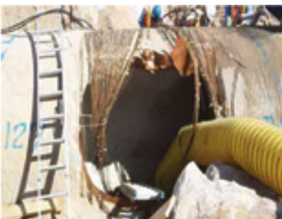
1. When prestressed concrete cylinder pipe fails, it often does so catastrophically
