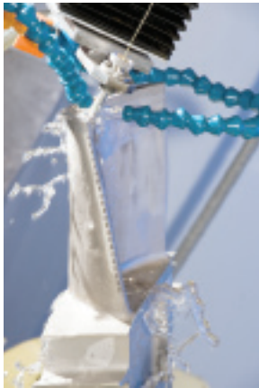
B6. Drilling cooling holes in 7FA first-stage bucket with EDM electrode (left)
