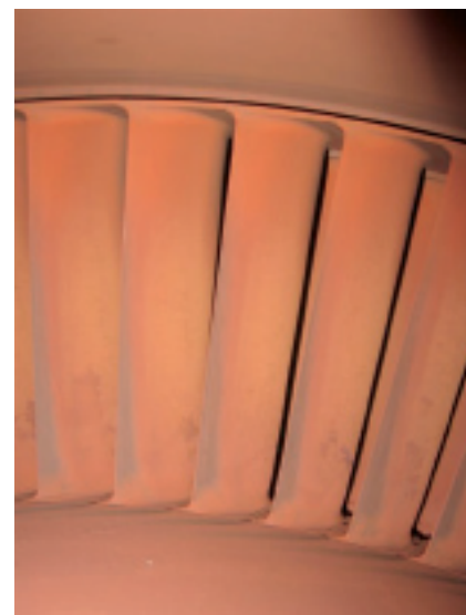
4. Corrosion products are transported throughout the condensate/feedwater circuit as evidenced by deposition on steam-turbine blades
