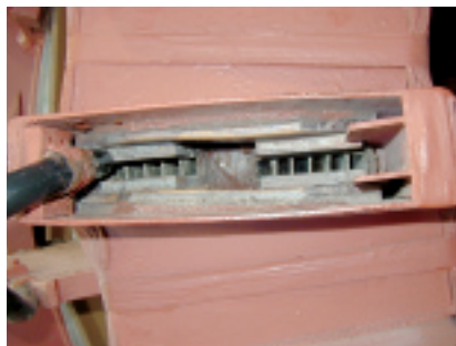
3. Stator winding RTDs and TCs can alert on significant change in winding copper temperature. Hose (arrow) picks up discharge air flow from stator bar and directs it to an RTD
