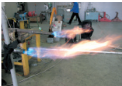
11. Ignition flame using orifice sizes recommended by CPS provides the thrust needed for successful starts
