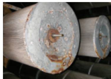
3. Galvanic corrosion from moisture ingress quickly chewed up metal portions of the original pulse-type filters
