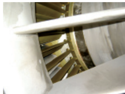
13. Unit 2 compressor inlet like new after 10,600 hours of operation with HEPA filters
