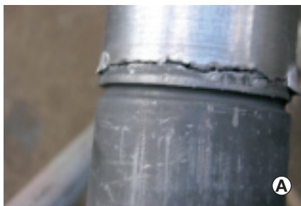
5. Desuperheaters take a beating in many combined-cycle plants. Note cracking of HP nozzle (A) and liner (B)
