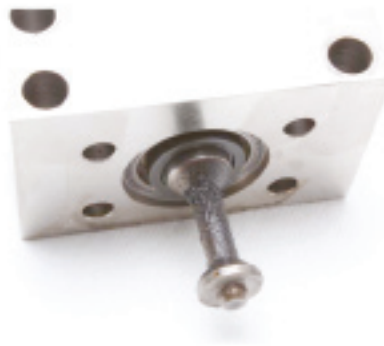
6. Cool means clean. After 80 hours in the oven, the spool for the water-cooled three-way purge valve looked almost new (left); that for the uncooled valve showed significant buildup of crud (right)
