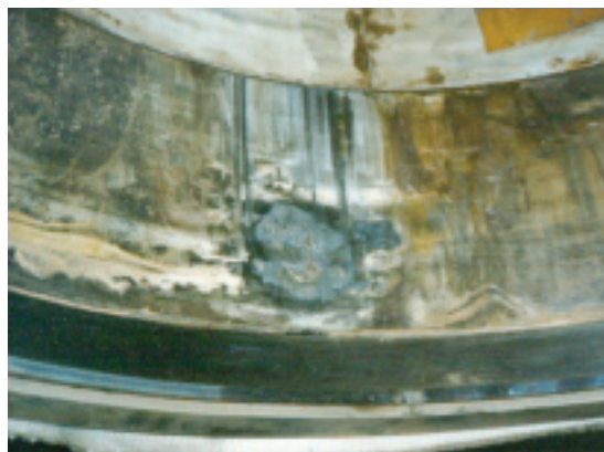
4. Severe burning on retaining-ring ID was caused by a single ground in the field winding
