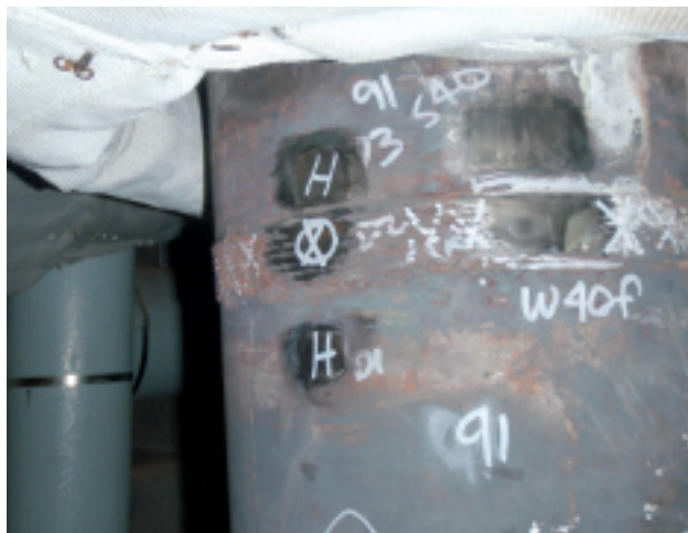
3. Weld joint was found with 1.25Chrome filler material instead of the required 9Chrome
