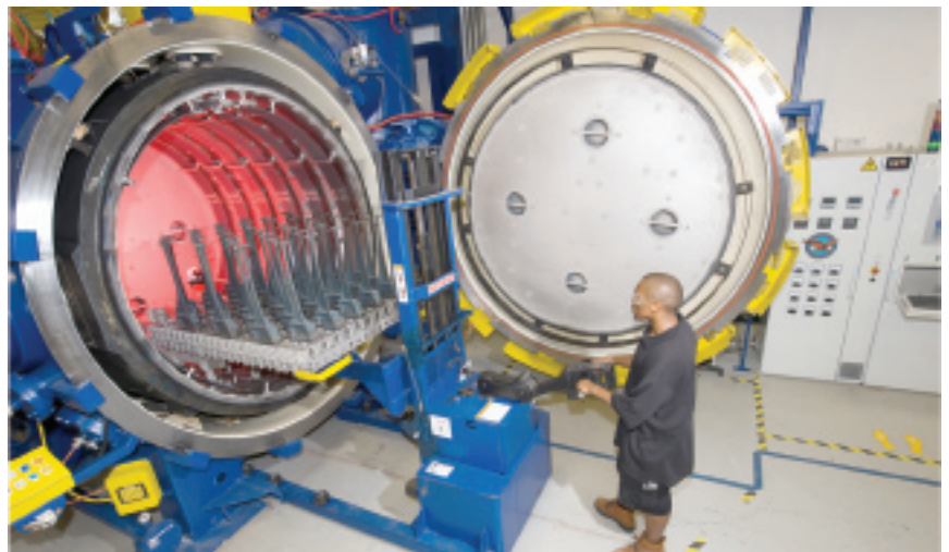
B2. Fred Miller loads one of the facility's new vacuum furnaces
