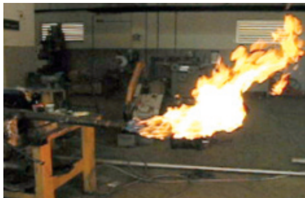
9. Ignition flame produced using the OEM's gas and air orifice settings is much too weak to achieve a high starting reliability on oil
