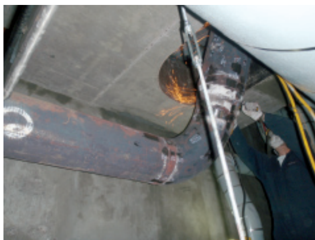
6. P91 pipe is prepped prior to taking hardness measurements
