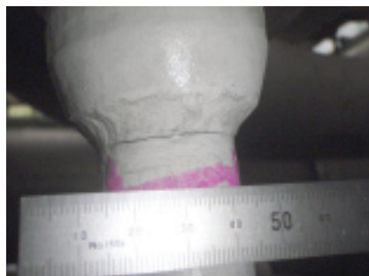
6. P91 components are not immune from cracking. HP drain line is one example
