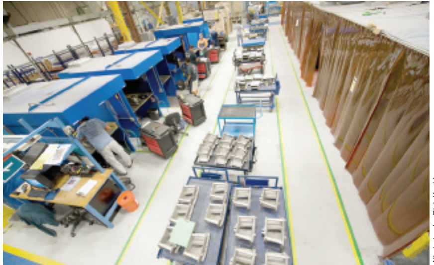
B1. Vane repair line extends from one side of the shop to the other
