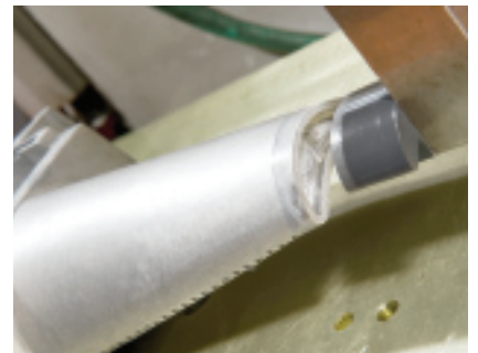
B5. Graphite-plunge EDM operating on a 7FA first-stage bucket
