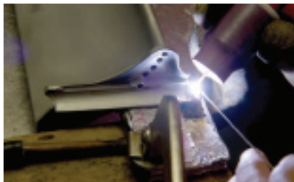
B11. Welding of Z notch on 7FA second-stage bucket
