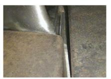
**1. Forward migration** of R0 compressor blades is conducive to leadingedge platform damage
