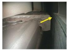
**13. Mounting hardware** fails on R17 stator vane and moves forward (direction of arrow), contacting the trailing edge of R17 airfoil
