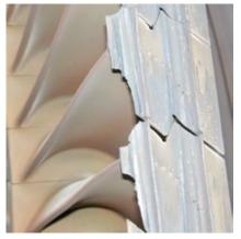
4. Close up of damage to the second-stage bucket shrouds
