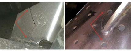
**14. Combustion inspection** shows cracks in the mounting bracket for original 12k transition piece (left). Cracking problem was transferred to the impingement sleeve in replacement 24k hardware (right)
