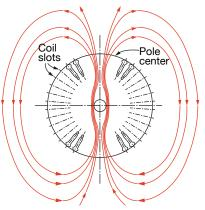
**1. Stator core** without the winding or other peripherals is at left, air-gap flux path for a 2-pole generator at right
