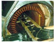
**13. High-flux test** typically is used today only when low-flux test results are questionable
