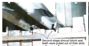
**2. Technicians from Advanced Turbine Support** also found material missing from the knife-edge seals on second-stage shroud blocks that had released from their slots
