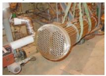
**12. Lube-oil-cooler** tube bundle should be removed periodically for condition assessment and cleaning
