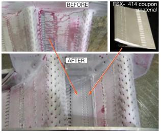
2. Weld repairs typically required on first-stage vanes are extensive, requiring bars and strongbacks to control distortion to the degree possible. Component shrinkage should be expected
