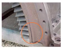
**6. Casing crack** like this generally is visible to a borescope technician looking inside the 10th-stage extraction cavity
