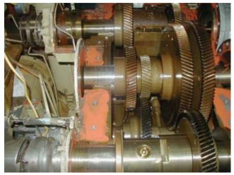
8. Components of a typical accessory gearbox are exposed with the cover off
