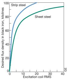
**26. Calculation of excitation** ampere-turns for high-flux testing is easy to do using curves in chart above. Not shown on the chart is the signature of author Clyde Maughan (Dec 4, 1952), then a GE employee, who developed the curves
