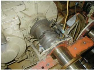
**9. Condition and alignment of a jaw clutch** must be checked; don't hesitate to replace when wear and tear is significant.
