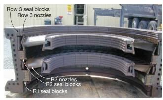
6. Position of turbine nozzles with respect to seal blocks is shown here
