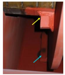
8. Core key bars are connected directly to the section plate via a bracket (yellow arrow) which, in turn, is connected rigidly to the frame (blue arrow)
