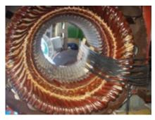
**11. Low-flux test** is performed using an excitation coil
