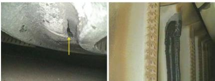
**18. Damage to first-stage bucket tip cap** (left, photo taken looking up at the bucket from below) must be found and addressed to prevent cooling-air starvation and damage at right
