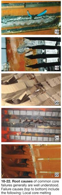
Failure causes (top to bottom) include the following: Local core melting probably caused by FOD (18), melting of core iron attributed to an over-flux incident (19), failing core caused by local looseness (20), core-iron melting attributed to a broken stator bar (21), and severe core impact damage caused by careless handling of the field during removal
