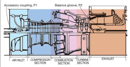
**2. Portable balance pickups** were installed on the output shaft of the accessory gearbox, the cold-end (P1) bearing, the hot-end (P2) bearing, the input side of the load gear, and the opposite side of the input high-speed pinion gear
