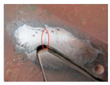
**12. Dovetail crack** is on the trailing edge of an R17 airfoil
