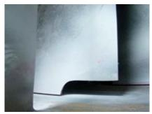
7. In-situ blending can eliminate cracks and avoid metal liberation and downstream damage
