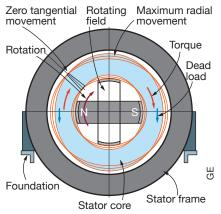
7. The large magnetic pull of the rotor air-gap flux on the core causes the latter to deform into an oval
