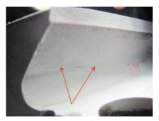
4. Crack in a R0 dovetail slot of the forward stub shaft is validated by red dye
