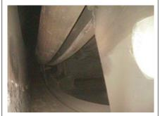
**20. Liberated flex-seal and ring pipe material** (above) damaged third-stage buckets (below)
