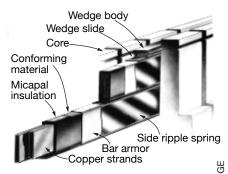
2. Core components and stator-bar support structure include core teeth, stator bars, wedges, packing, and side pressure springs
