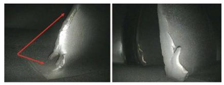
**11. Clashing damage** is in evidence on trailing edge of R3 rotor blade (left) and on the leading edge of an S3 stator vane (right)
