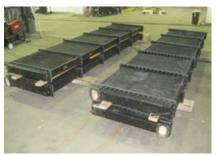
**13, 14. Radiators must be flushed** and pressure-tested regularly (left); clean radiators ready for installation are at right
