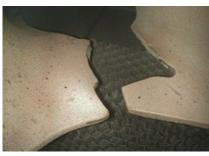
**19. Tip shroud liberation** from second-stage bucket is addressed by TILs 1858, 1859, and 1863
