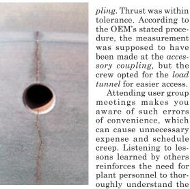
1. Crack at clearanceometer hole, Row-3 12 o'clock position
