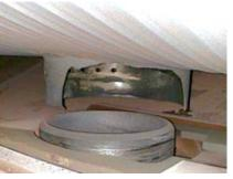
**16. Collar for crossfire tube** liberated and the tube dropped out. This also was found during a combustion inspection
