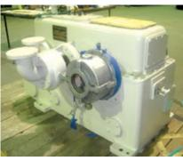
**10. SSS clutch** replaced original jaw clutch
