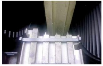
**12. Second-stage buckets and shroud blocks** were repaired successfully
