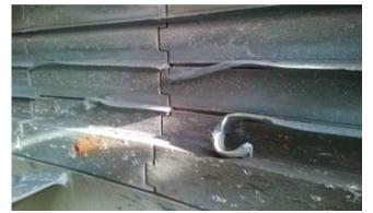
**7. Damage to second-stage shroud-block seal teeth** was extensive. Note that rotor rotation is from left to right, gas flow is from the bottom of the picture to the top
