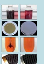
**Before** & **after** installation of a CJC™ Varnish Removal Unit VRU
