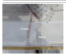
**3. Expert weld repairs** using the proper filler material can last a long time. Cracks develop elsewhere to relieve stresses in the component
