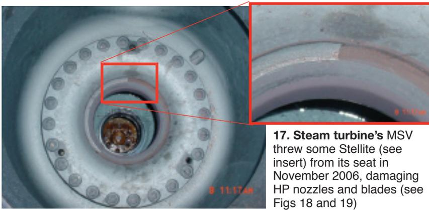
17. Steam turbine's MSV threw some Stellite (see insert) from its seat in November 2006, damaging HP nozzles and blades (see Figs 18 and 19)
