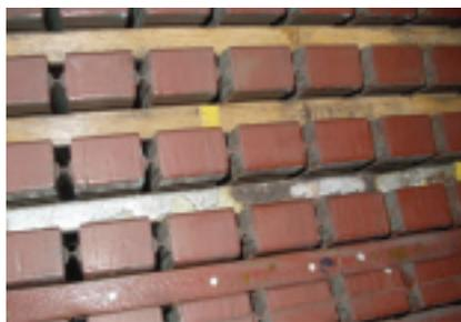
7. Advanced partial discharge activity is in evidence on bar surface
