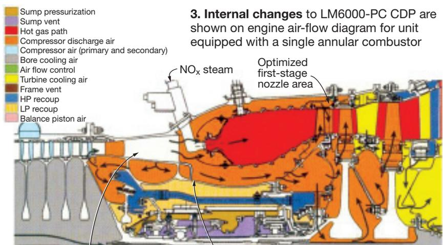
**3. Internal changes** to LM6000-PC CDP are shown on engine air-flow diagram for unit equipped with a single annular combustor
