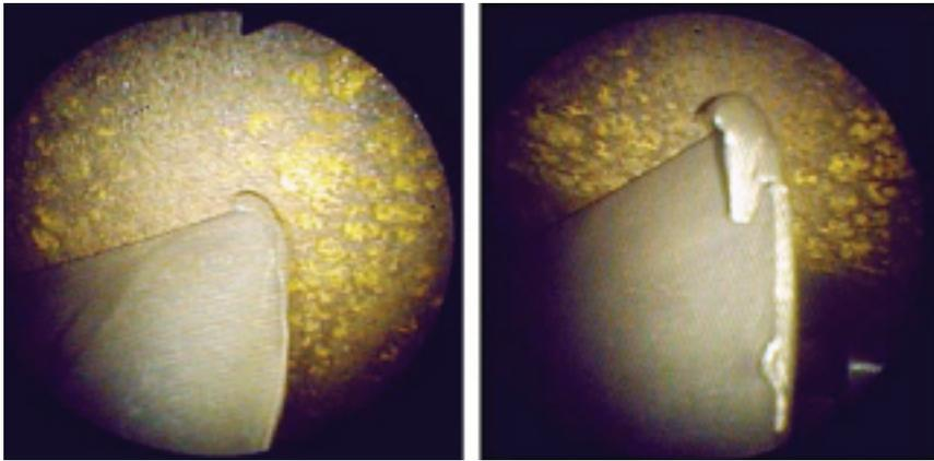
**8. Smeared and rolled metal** on adjacent stator vanes (damage area on vane at left, 1 × 0.25 in.; at right, 1 × 0.375 in.) proved clashing was increasing in severity since its discovery a year earlier
