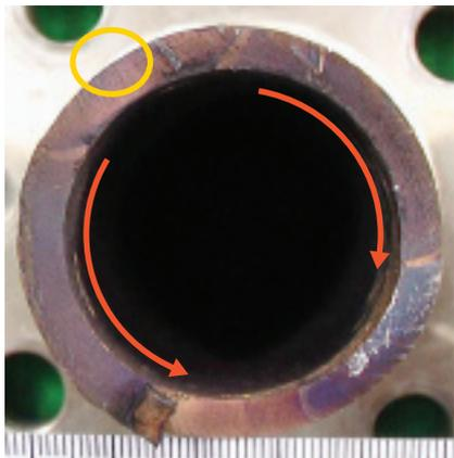
**20. Analysis of fracture surface** revealed striations characteristic of HCF along the red arrows. Starting point of the cracks appeared to be in the yellow circle at the back ends of the arrows (left)
