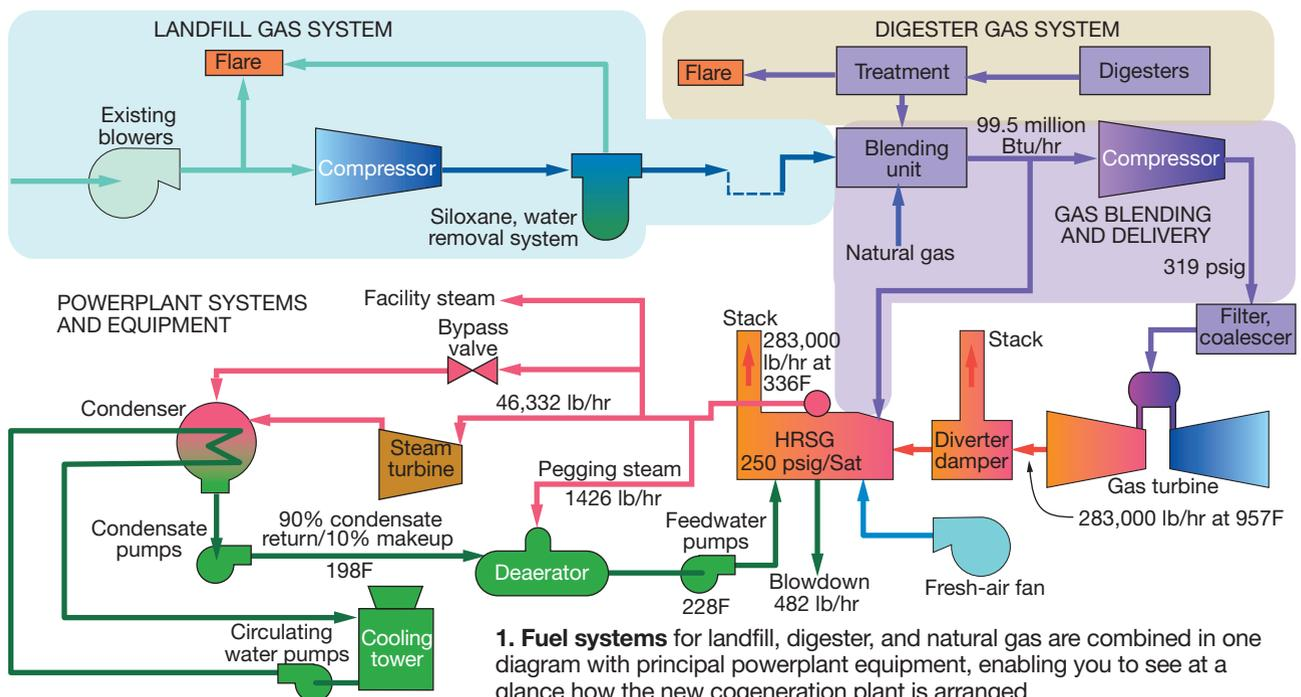
**1. Fuel systems** for landfill, digester, and natural gas are combined in one diagram with principal powerplant equipment, enabling you to see at a glance how the new cogeneration plant is arranged
