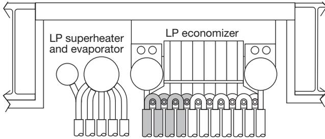
**7. Four rows of LP economizer tubes were removed (color), reducing backpressure by 3.7 in. H<sub>2</sub>O**
