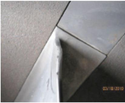
**3. Damage to trailing edge** of rotating blades. More specifically, deformation and some lift-up of material near the platform at the trailing edge
