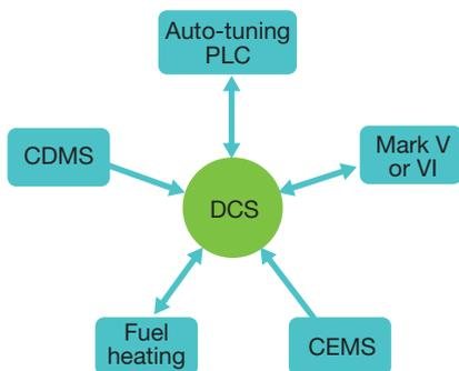
**31. CDM system** continuously monitors combustion dynamics and relays this information to the DCS, which monitors emissions and sends data to the auto-tuning PLC. The PLC determines when adjustments are necessary and automatically tunes the turbine to the operator's optimization goals.
