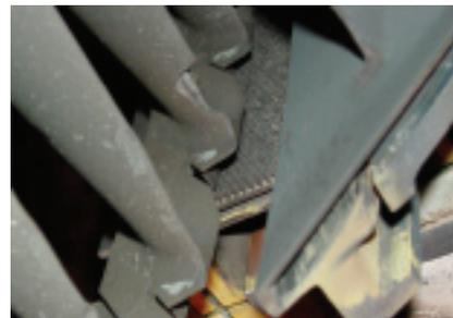
**2. Part of a UV detector tube liberated, traveled downstream, and damaged R3 blades and other components**
