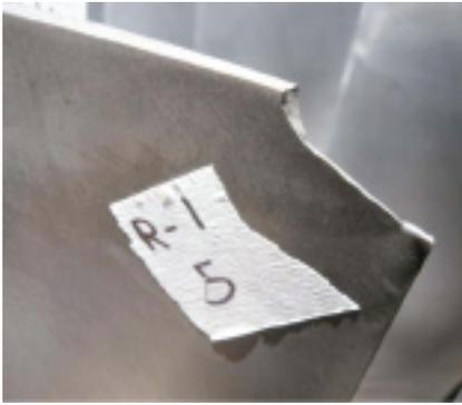
1. Classic tip crack is shown at the left with crack initiation about 2 in. from the leading edge. Impact caused the damage at the right
