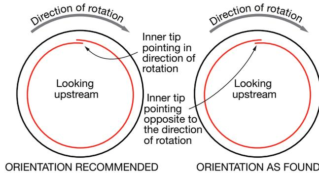
16. Inner tip of the lock wire should point in the direction of rotor rotation to help prevent the lock wire from moving
