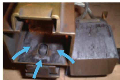
**22. Carbon deposits** inside the brush holder can restrict brush movement and prevent it from properly contacting the collector ring
