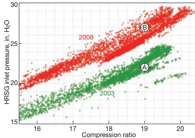
5. Historic data show a nominal increase in HRSG inlet pressure of 5 in. H<sub>2</sub>O (point A to point B) over a five-year period because of fouling
