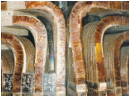
**16. Significant coil/turn distortion** is evident with the retaining rings removed
