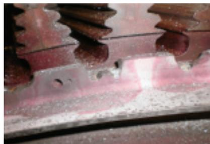
**5. Blend repair** reflects OEM's recommended procedures
