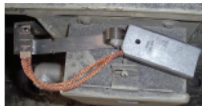
**23. Constant-pressure springs** cause side pressure that results in brush binding and scoring
