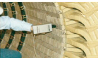
21. Hand-held taper checks tightness of stator wedges
