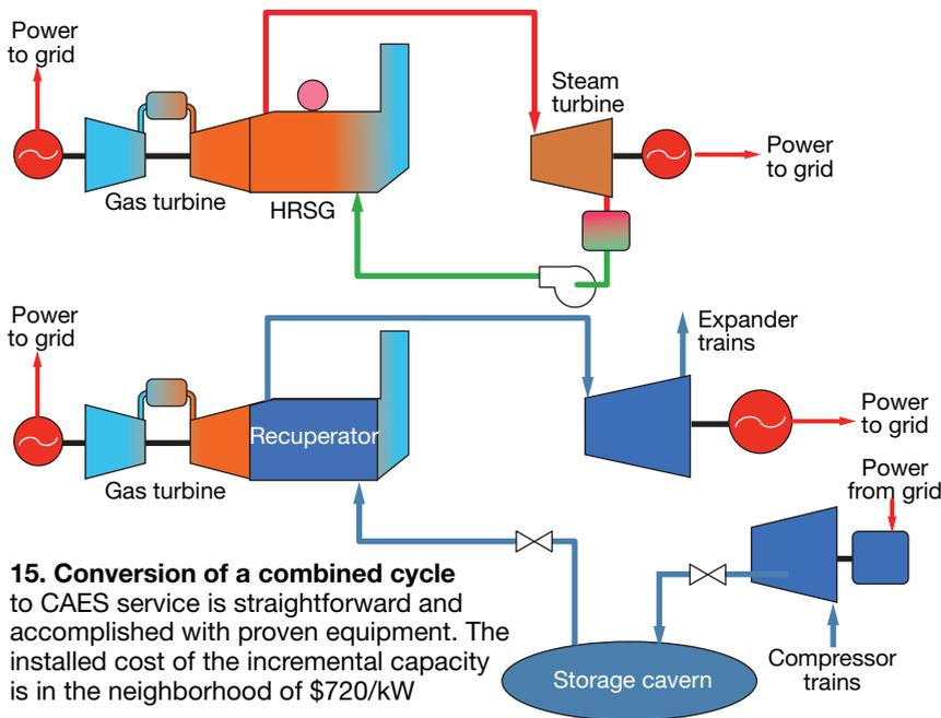
**15. Conversion of a combined cycle to CAES service is straightforward and accomplished with proven equipment. The installed cost of the incremental capacity is in the neighborhood of \$720/kW**
