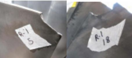
20 7F tip cracking
