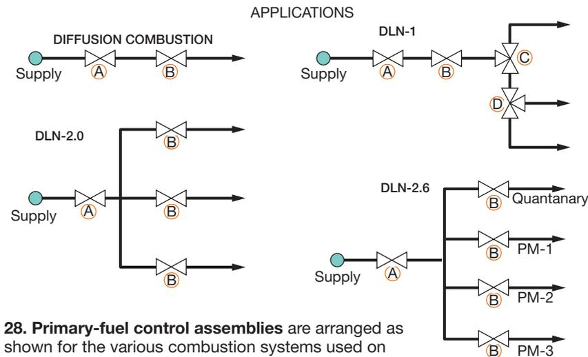
**28. Primary-fuel control assemblies** are arranged as shown for the various combustion systems used on large GE frames
