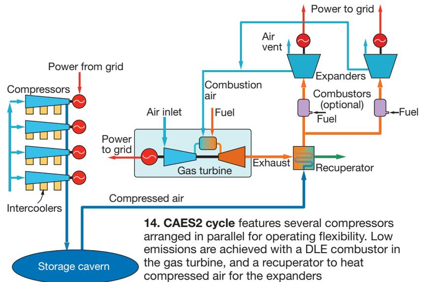
**14. CAES2 cycle** features several compressors arranged in parallel for operating flexibility. Low emissions are achieved with a DLE combustor in the gas turbine, and a recuperator to heat compressed air for the expanders
