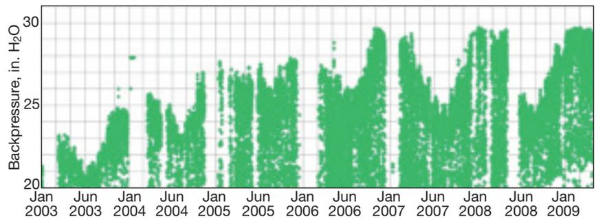
**6. HRSG backpressure** over time illustrates seasonal variations—valleys in summer, peaks in winter. Boiler limit is 30 in. H<sub>2</sub>O, forcing operators to manually limit gas flow through the HRSG on occasion by changing position of compressor inlet guide vanes
