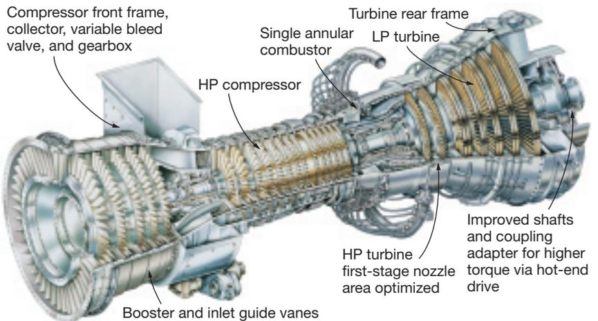
**1. STIG-equipped LM6000-PC**, designated the LM6000-PC CDP, shows some minor modifications from the baseline engine. The HPT first-stage nozzle area, shafts, and coupling adapter called out in the diagram have been modified; other parts are standard PC components
