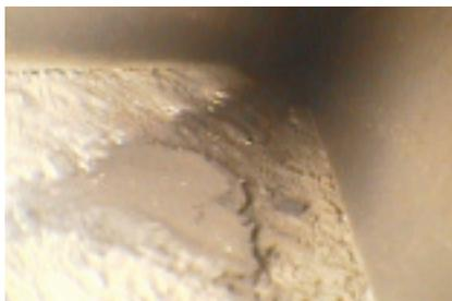
8. Spark damage caused by vibration is seen in ventilation duct through a borescope
