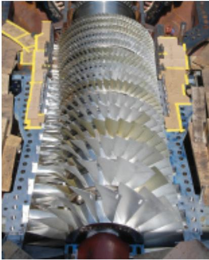
**1. Redesigned W501G compressor** incorporates features of Siemens' V-style machine to address wear issues (left)
