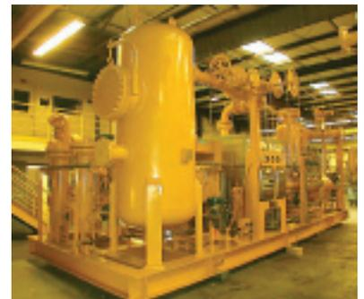
*Screw fuel gas boosting compressor
