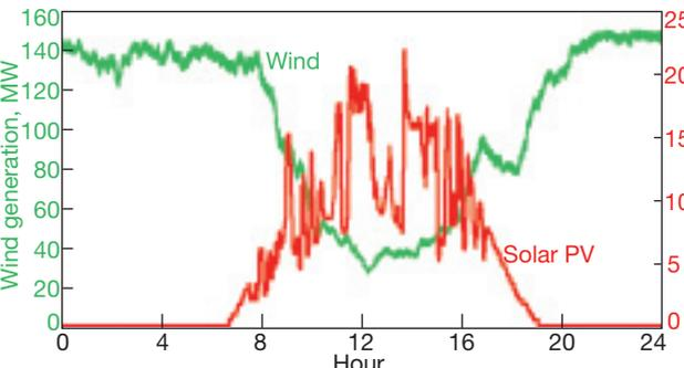
**8. Variability in wind and solar** generation are compared for a cloudy California day. The solar PV field is rated 24 MW, the wind farm 150 MW
