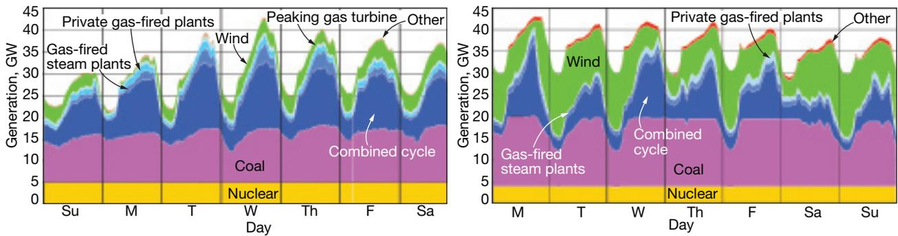
**12. Actual dispatch map for ERCOT generation assets** during a typical week in April 2009 (left) and how that would compare to a windy week in March 2013 (based on modeling results) when almost double today's wind generation is expected in operation
