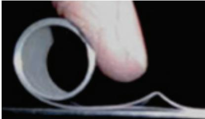
**24. Spring wear and tear** (note kink under finger) compromises proper brush-to-ring contact pressure
