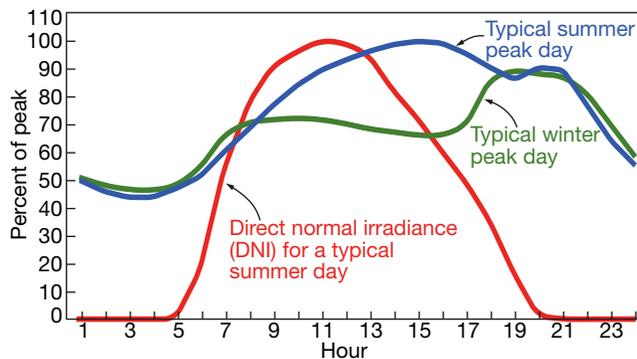
24. Solar power produced at maximum DNI is stored in a battery and released later in the day when demand is highest
