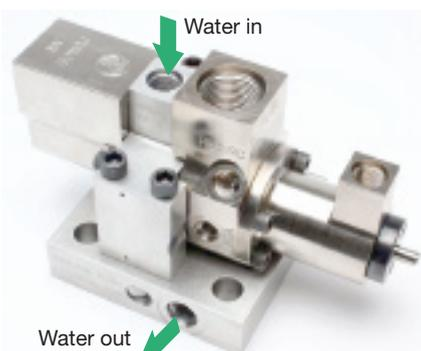
**27. The three-way purge valve** was a significant advancement in fluid handling technology because it combined the liquid-fuel and purge-air valves in one unit and improved system reliability (left). But coking remained an issue for many owner/operators. JASC’s solution was to incorporate a water-cooling circuit into the valve as it had successfully done for the standalone liquid-fuel check valve a few years ago (right)
