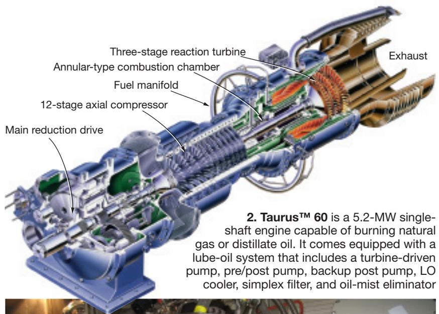
**2. Taurus™ 60** is a 5.2-MW single-shaft engine capable of burning natural gas or distillate oil. It comes equipped with a lube-oil system that includes a turbine-driven pump, pre/post pump, backup post pump, LO cooler, simplex filter, and oil-mist eliminator
