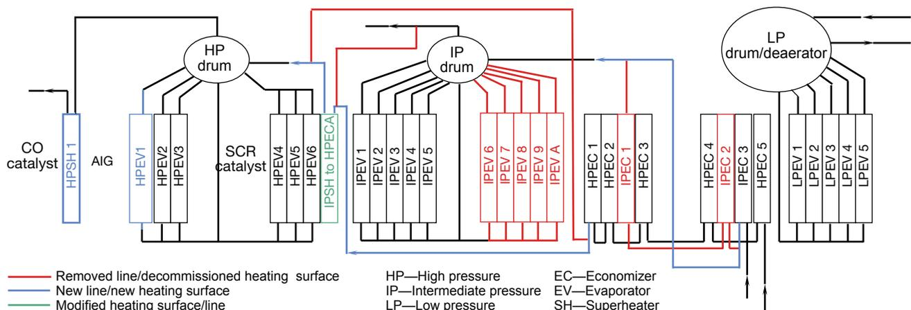
**4. Heat-recovery steam generator,** which supplies STIG and NO<sub>x</sub> steam to the gas turbine required a redesign effort, some new components, and modification of others to accommodate the change in engines from LM5000 STIG 120 to LM6000-PC CDP
