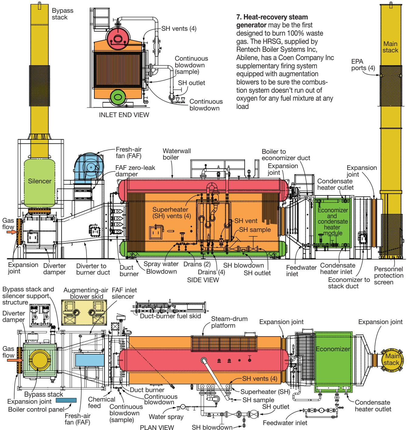
**7. Heat-recovery steam generator** may be the first designed to burn 100% waste gas. The HRSG, supplied by Rentech Boiler Systems Inc, Abilene, has a Coen Company Inc supplementary firing system equipped with augmentation blowers to be sure the combustion system doesn't run out of oxygen for any fuel mixture at any load
