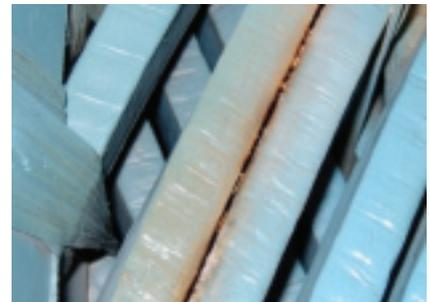
**11. Partial discharge attack** is in evidence at line-to-line phase break
