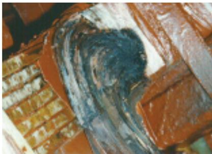
**9. Failing series connection** was identified on stator end windings
