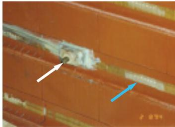
**4. Flux probe** (white arrow) is highly reliable and can determine the precise coil where a short exists. The green arrow points to seven holes in the wedge for measuring radial spring compression height, which is indicative of the wedging force on the stator bar
