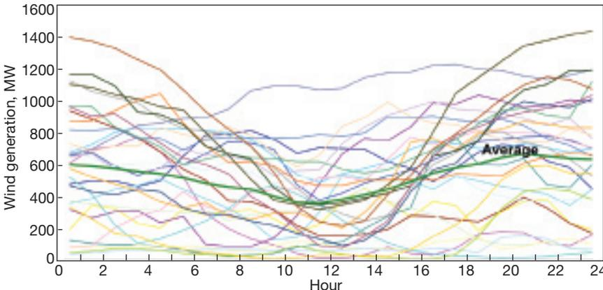
**7. Wind generation** can vary dramatically from day to day. Each curve above illustrates the wind generation profile for one day in April 2009. Knowing what to expect from wind when lining up resources a day ahead is challenging for grid operators like the CalISO, which developed this chart based on its system data
