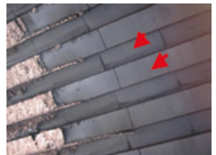
10. Tapered inserts correct tooth tip looseness
