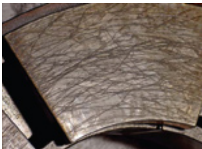
1. Stray shaft currents caused arcing that damaged this thrust-bearing shoe
