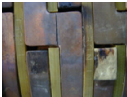
22. Broken coil-to-coil connection produced limited arc damage
