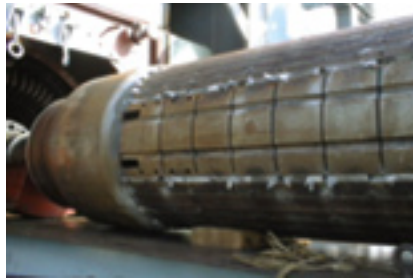
28. Extreme overheating of field forging during a negative-sequence field current event makes this component scrap
