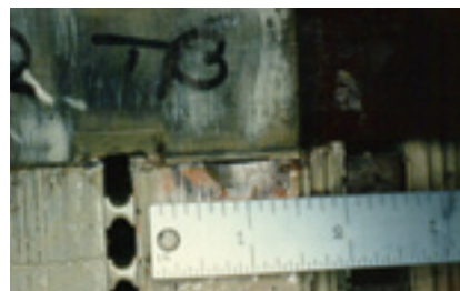
1, 2. Local core overheating was caused by damage to the insulation of a few laminations (left). Section of damaged laminations was safely removed by careful grinding (right)
