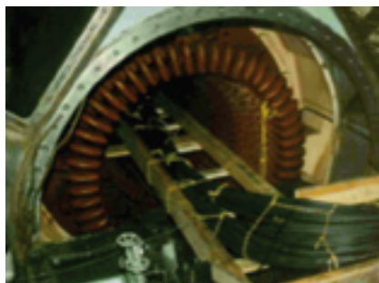
13. Heavy excitation coil is required for a high-flux test
