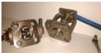
1. Manual ball valve has removable top for maintenance and inspection. The copper-coated ring is the body-to-bonnet seal
