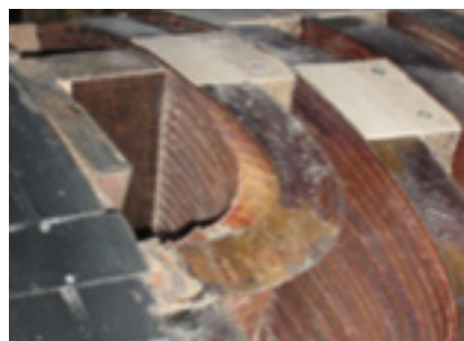
16. Top turn of the smallest coil is distorted
