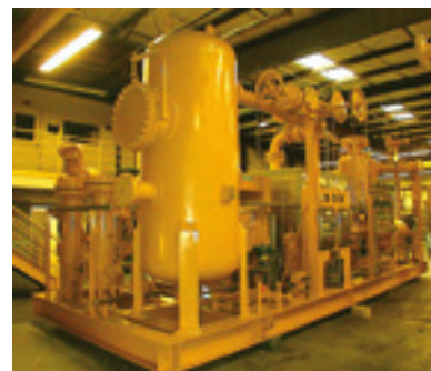
Screw fuel gas boosting compressor used with aeroderivative gas turbine (output: 50 MW)
