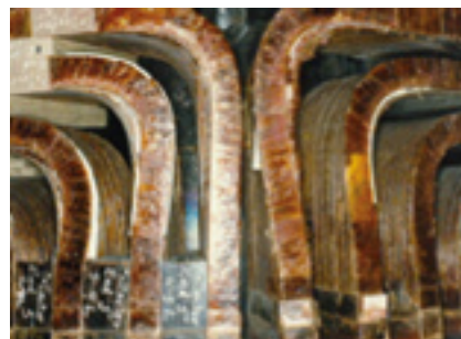
18. Coil/turn distortion shown here is serious and widespread
