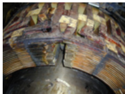
17. Severe distortion of top turns on several coils is in evidence
