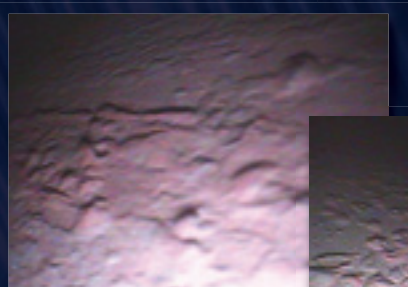
Pitting inside boiler tubes can be avoided if water is degassed
