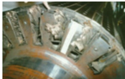
32, 33. Fractured 18/5 retaining ring failed after exposure to raw water while in service (left) ; field winding after the ring failure is at right
