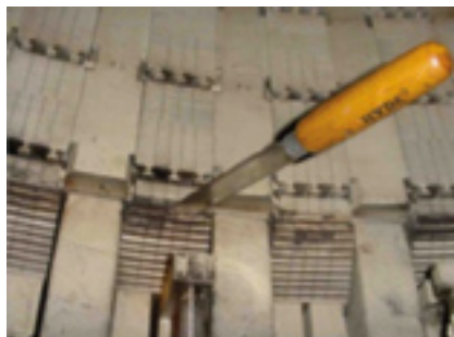
11. Ability to insert a knife into the core confirms loose tooth iron
