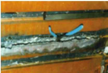
4. Severe melting caused failure of the entire tooth
