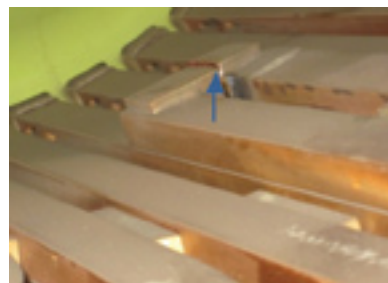
24. Pole-to-pole connection at the bottom of the coils is fractured (arrow)
