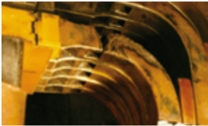
19. Top turn in field winding is broken
