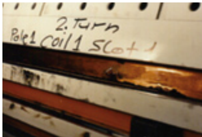
20. Burning between winding and forging occurs because field current continues to flow after a turn break
