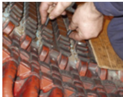
12. Step iron at the end of the core is tested manually
