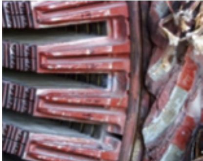
6, 7. Slight discoloration of iron was considered minor (left), but melting at that spot after a few hours of operation with a new winding (right) proved that diagnosis incorrect
