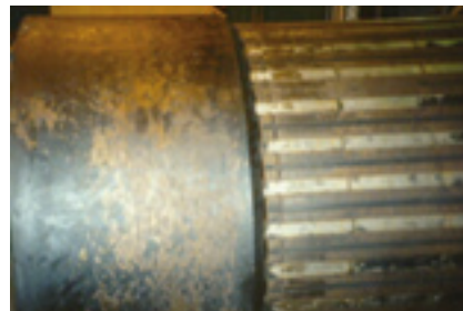
15. Rust condition can damage forgings. Resulting conductive materials can contaminate the extensive electrical creepage surfaces
