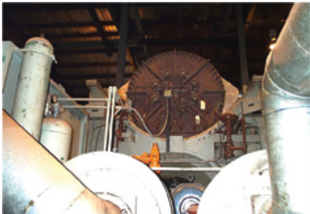
2. Combustion system has eight burners. Combustion chamber is 4 ft in diameter
