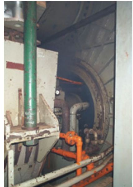
8. Blue smoke started spewing from the bearing tunnel although the expansion-joint repair was successful
