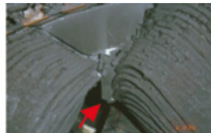
34, 35. Failure of a single bolt initiated the cascading failure of the remaining bolts for this salient pole field
