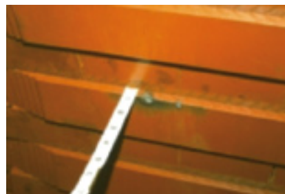
1, 2. Local core overheating was caused by damage to the insulation of a few laminations (left). Section of damaged laminations was safely removed by careful grinding (right)
