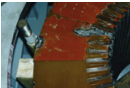
8. Core melting caused by over-fluxing is very severe
