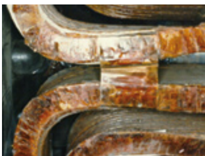
23. Top-to-top connection will lose flexibility if excessive braze material is applied
