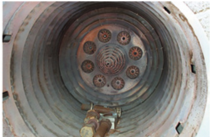
2. Combustion system has eight burners. Combustion chamber is 4 ft in diameter
