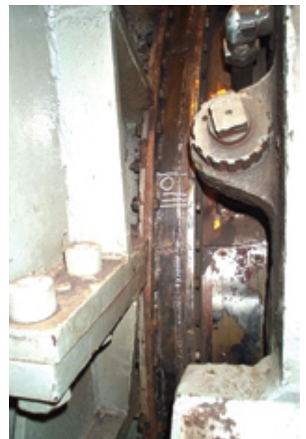
6. Overlay strap avoided a costly complete disassembly and replacement joint
