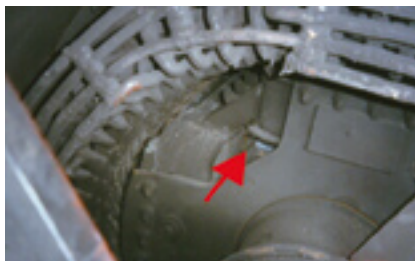
34, 35. Failure of a single bolt initiated the cascading failure of the remaining bolts for this salient pole field
