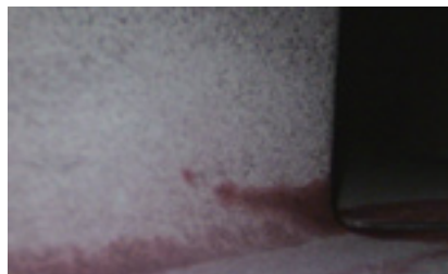
2. Trailing-edge platform crack on S0 vane identified with visible dye penetrant
