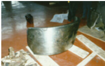
32, 33. Fractured 18/5 retaining ring failed after exposure to raw water while in service (left) ; field winding after the ring failure is at right
