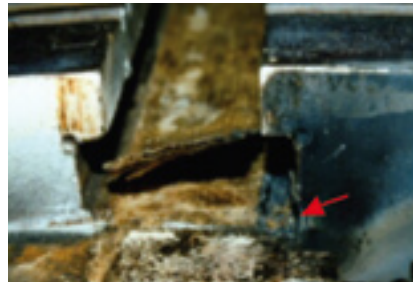
31. Double field-winding ground damaged field forging tooth
