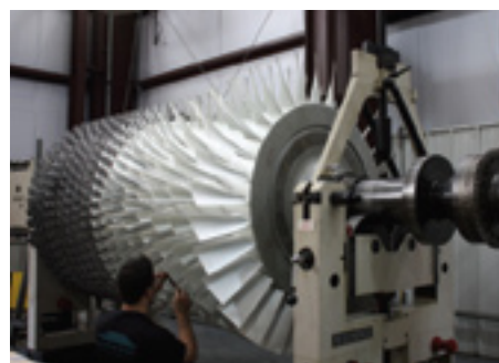
D. Balancing and run-out checks are final steps in the rotor overhaul process
