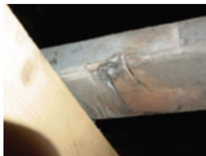
9. Stator-bar insulation damage was caused by lamination looseness
