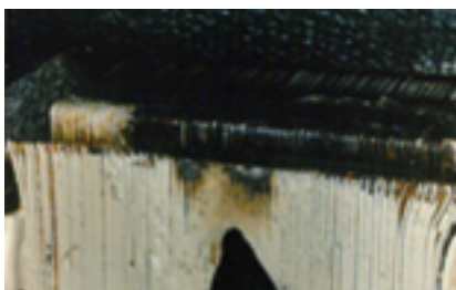
1, 2. Local core overheating was caused by damage to the insulation of a few laminations (left). Section of damaged laminations was safely removed by careful grinding (right)
