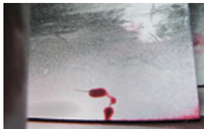
1. Radial tip crack on R1 blade identified with visible dye penetrant
