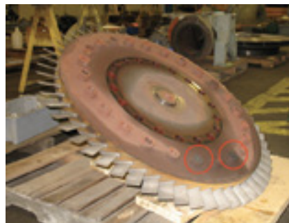
13, 14. A couple of marriage bolts sheared off during the unbolting process (left). Optimal solution was to swap out the affected 16 th compressor stage on the replacement unit with that from the original Ascutney machine (right)
