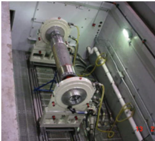
8. High-speed balancing, seasoning, and overspeed testing greatly reduce the potential for rotor-related issues during startup
