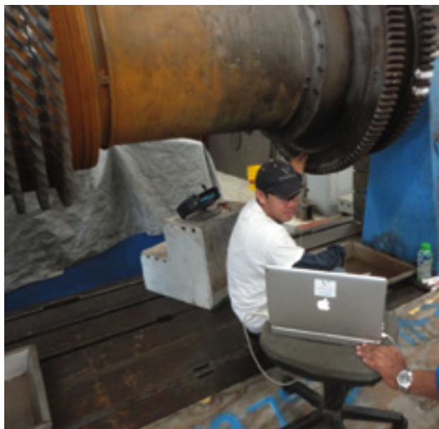
45. Ultrasonic inspection is conducted of the turbine first stage without disassembling the rotor
