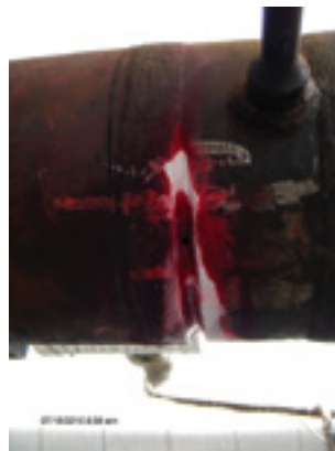
16. Failure of this dissimilar weld was spotted before any collateral damage occurred
