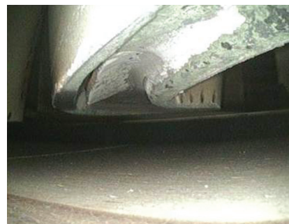
8. Bulging and material separation on the suction side
