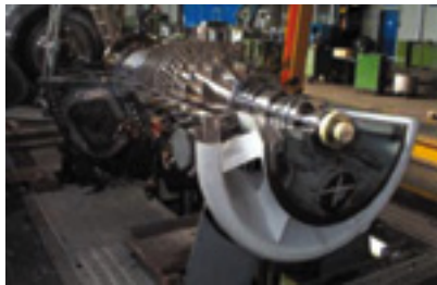
HP rotor assembly for the MS5002E is in the left-hand photo, the engine proper is at the right
