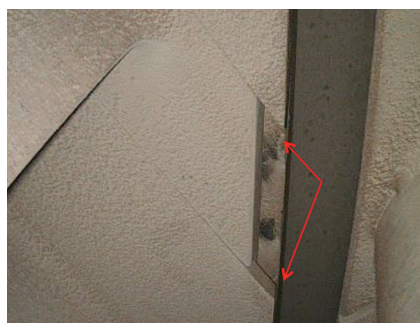
12. Upstream movement of compressor S17 rotor blade
