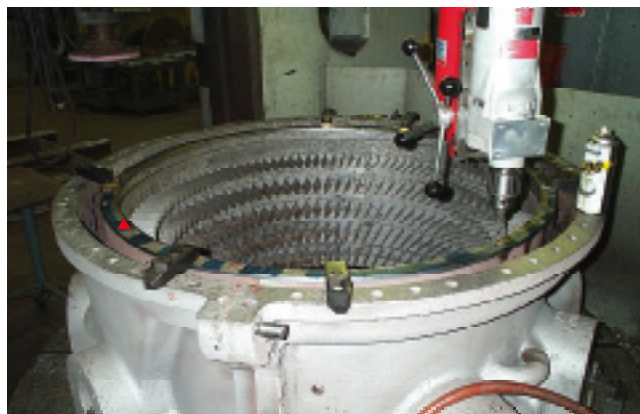
34. Mid compressor case is bolted together in the shop where two 180-deg patch rings are installed and fastened to the casing with counter-sunk flat-head bolts to form a new hook for the ninth stage
