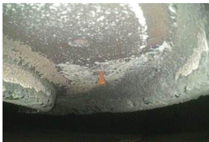
4. Blocked cooling hole at leading edge of tip cap
