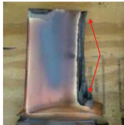
3. Leading-edge cap loss occurs after the protection provided by the coating is gone
