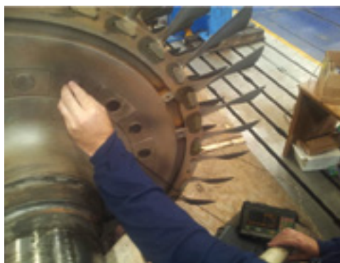
46. Compressor through-bolts are ultrasonically checked to determine their condition.
