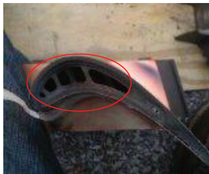
1. Complete loss of bucket tip cap is rare
