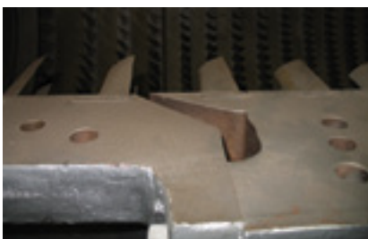
18. Ninth-stage hookfit area , prone to cracking as Frame 5s age, was in good condition
