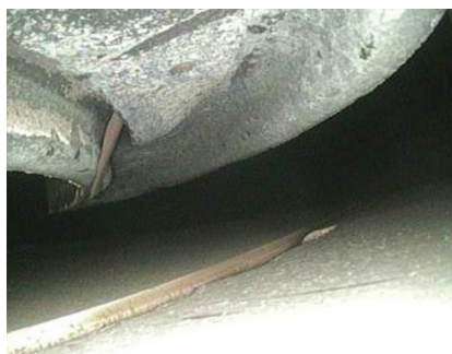
5. Bulging and material separation at leading edge of tip cap. Note debris protruding through opening where the material has separated
