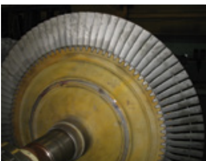
15, 16. Fir trees in the first-stage turbine wheel were grit blasted after buckets were removed (left); second-stage wheel was cleaned with buckets in place (right)
