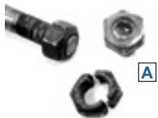
1. Failure of bolts (A) allowed combustion can cover to blow off (B), causing collapse of liner and flow sleeve (C)
