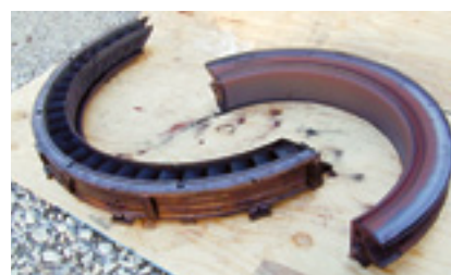
36. Half of each nozzle ring has five segments with five airfoils per segment (left); support ring is at right
