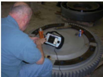
13. End-of-life inspections require an array of specialty NDE tools and knowledgeable technicians
