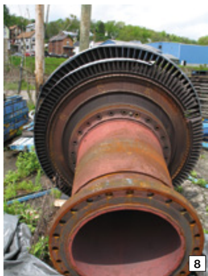
8-10. Original Ascutney distance piece and turbine section were scrapped (8). R1 fir trees were no longer fit for duty as close-up image reveals (9); the second-stage wheel also shows the wear and tear of a tough life (10)
