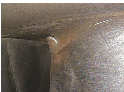
20. First-stage stator vane tear on trailing edge (suction side)
