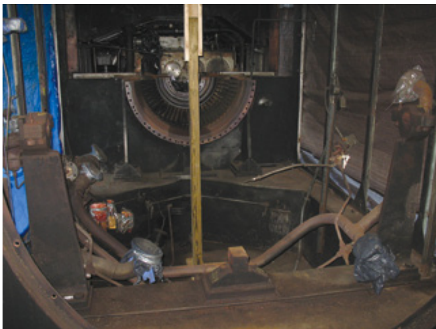
7. Engine removed, connection to the auxiliaries compartment is visible along with lube-oil piping
