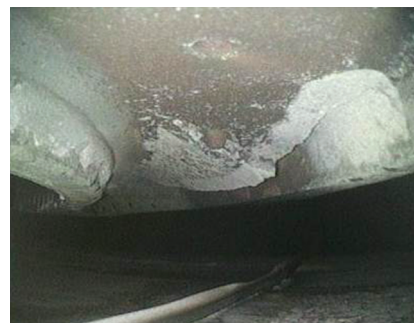
7. Another view of bulging and material separation at the tip-cap leading edge
