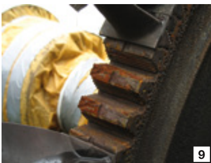
8-10. Original Ascutney distance piece and turbine section were scrapped (8). R1 fir trees were no longer fit for duty as close-up image reveals (9); the second-stage wheel also shows the wear and tear of a tough life (10)
