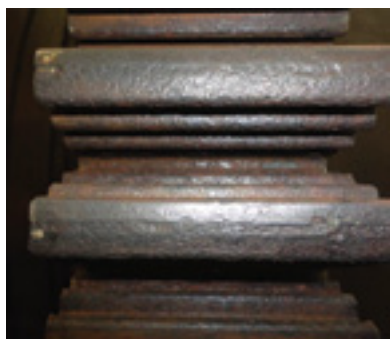
43. Closer examination revealed flaw in Fig 42 was a cluster of indications (above)
