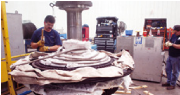
Induction heating coil is installed to expand the turbine wheel and facilitate removal of rusted-in buckets
