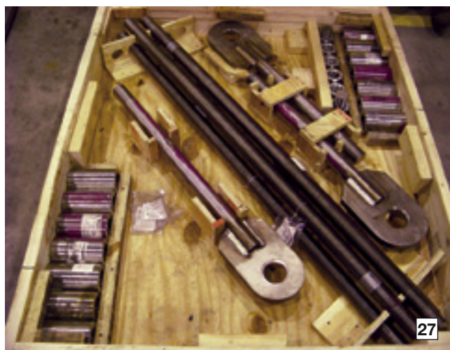
25-28. Replacing fixed supports on the upper headers for Reheater 1 with spring cans is expected to reduce significantly the number of tube failures in the years ahead. Lugs supports are added in Fig 25, spring cans and associated hardware are shown in Figs 26 and 27; the installed cans are in Fig 28
