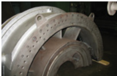
19, 20. Condition of the exhaust end of the lower casing half was fair (left), as was the upper half of the exhaust casing (right)
