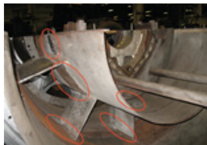
21, 22. Exhaust-end patch repairs were sufficient as there was no major damage (left). Even the diffuser, which was missing a couple of pieces of metal, could be repaired adequately by scavenging parts from the original GT (right)
