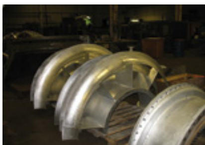
21, 22. Exhaust-end patch repairs were sufficient as there was no major damage (left). Even the diffuser, which was missing a couple of pieces of metal, could be repaired adequately by scavenging parts from the original GT (right)
