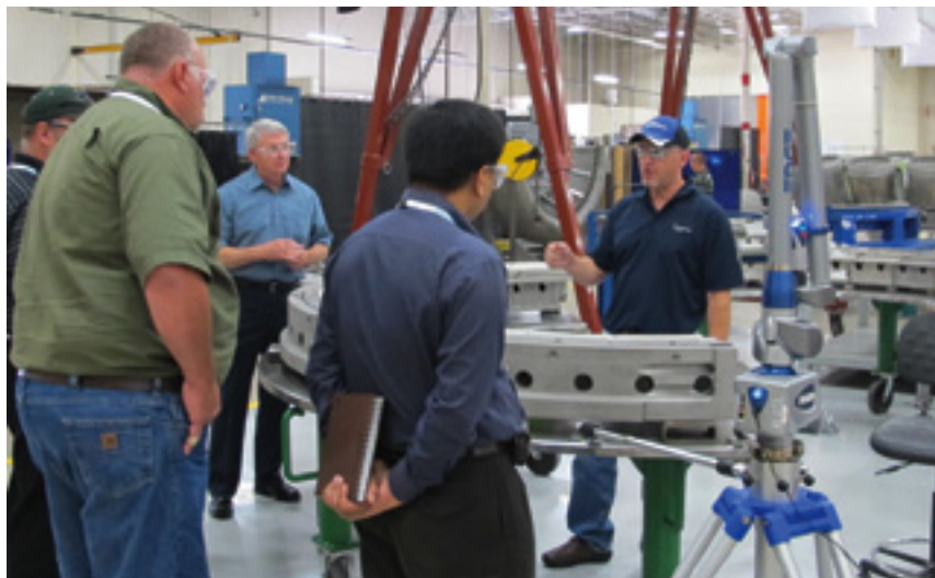
3. Liburdi's Rob Rowland explains the use of inspection arms for dimensional measurement (of a vane ring here) and model formation. Fit-up of transition pieces is verified in jig behind and to the right of Rowland
