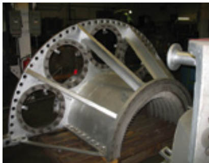
11, 12. The replacement MS5001D was in reasonably good condition as indicated by tight, unscathed compressor vanes (left) and the top compressor case for Rows 10-16 (right)
