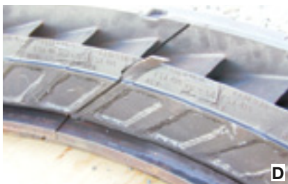
35. Seal between adjacent nozzle blocks looks almost normal in A, except for the cracked weld. Seal has migrated downstream about an inch in B. Downstream side of seal, seen with borescope before machine disassembly, is approaching the first-stage rotating buckets in C. Seal migration is more pronounced in D after nozzle blocks have been removed from the unit
