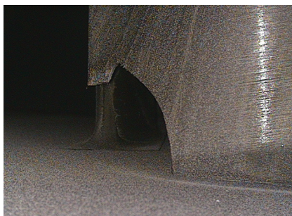
18. Second-stage rotor blade tip liberation (trailing edge)
