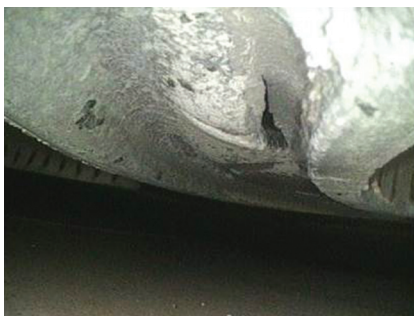
6. Bulging and material separation viewed from the trailing edge
