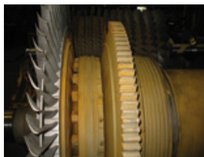
15, 16. Fir trees in the first-stage turbine wheel were grit blasted after buckets were removed (left); second-stage wheel was cleaned with buckets in place (right)
