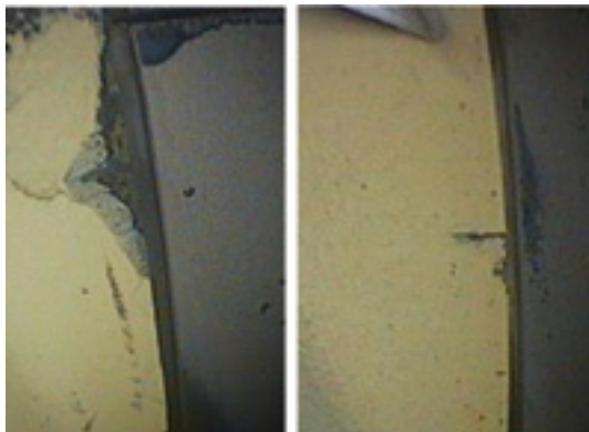
13. Erosion of the S2 nozzle's outer platform trailing edge starts as a crack in the parent metal (right) and moves forward exposing the shroud's leading edge
