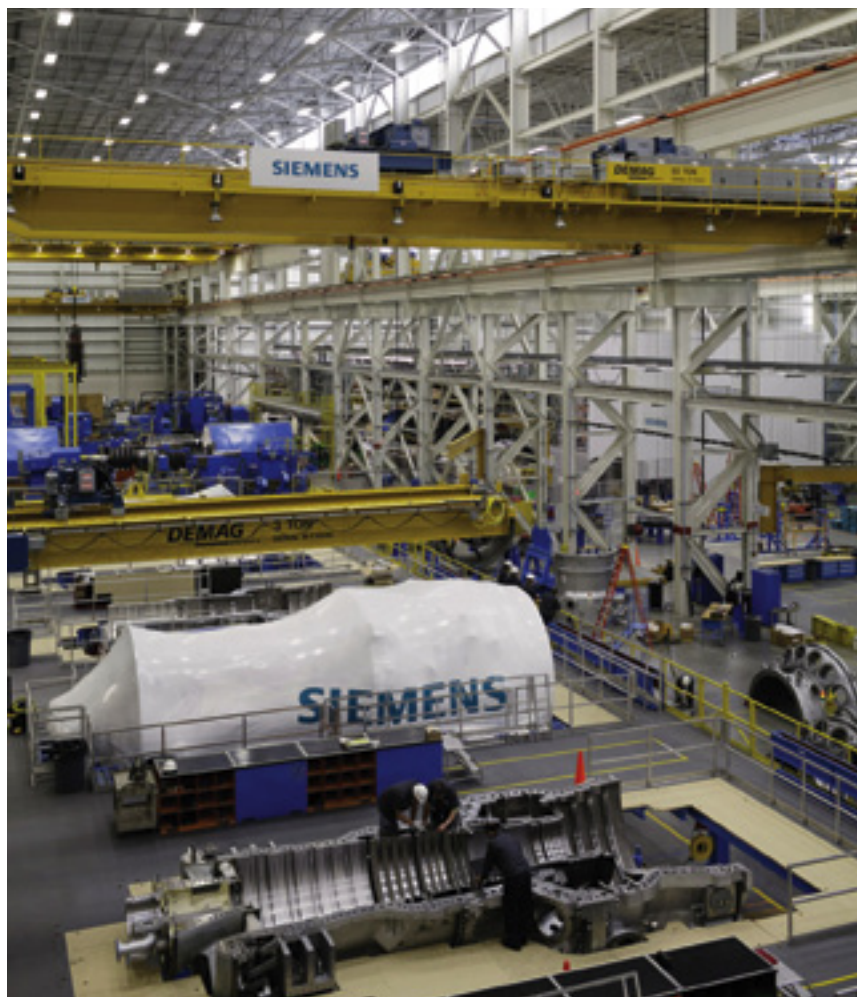
1. Gas-turbine assembly area at the Siemens manufacturing facility can accommodate seven engines
