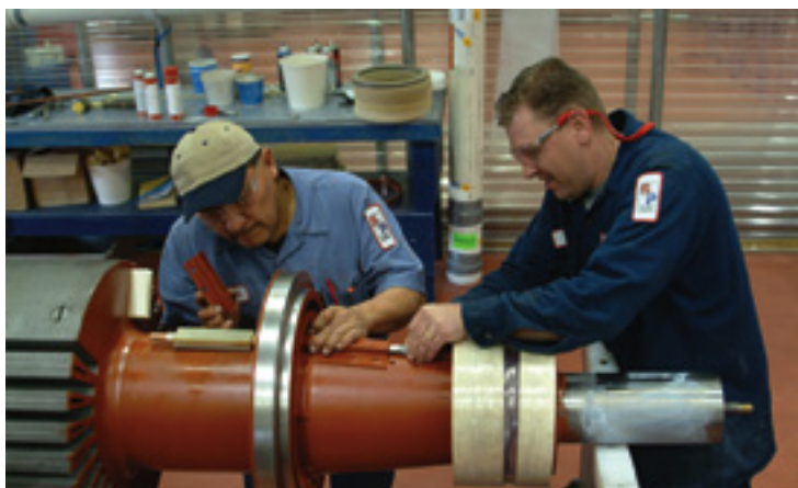
4. Generator rotor rewind rejuvenates the rotating element. An increase in the temperature class of the associated insulation system from Class 130 (B) to Class 155 (F) benefits the user by extending service life and uprate potential
