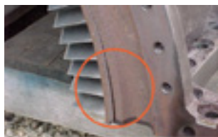
25. Casing crack generally is visible to borescope technician looking inside the 10 th -stage extraction cavity (below)
