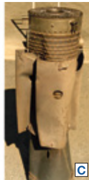
2. Portions of failed ductwork bolts were sucked into the inlet air stream and carried into the compressor, damaging airfoils. Note that the compressor shown is for a 7B. Shuman said he used pictures from Frame 5s, 6s, and 7B-EAs in his presentation, but that the damage illustrated has affected virtually all GE frames
