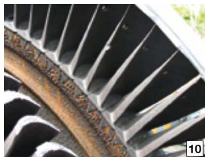
8-10. Original Ascutney distance piece and turbine section were scrapped (8). R1 fir trees were no longer fit for duty as close-up image reveals (9); the second-stage wheel also shows the wear and tear of a tough life (10)
