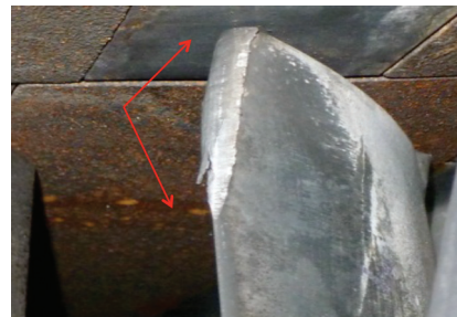
10. Tip damage on the leading edge of this S1 stator vane was caused by clashing
