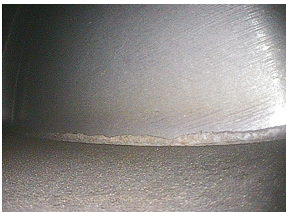
19. Second-stage rotor blade with rolled metal
