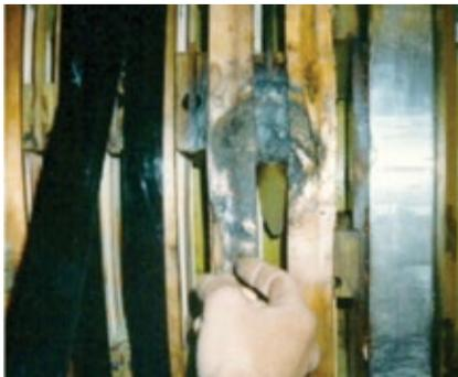
**4-4. Arc damage from shorting** between two coils (left) effectively removed the coils from the excitation circuit. The single ground lasted for a significant period of time because the detection circuit was connected incorrectly. Result: Near-fatal burn damage to the retaining ring (inside diameter)
