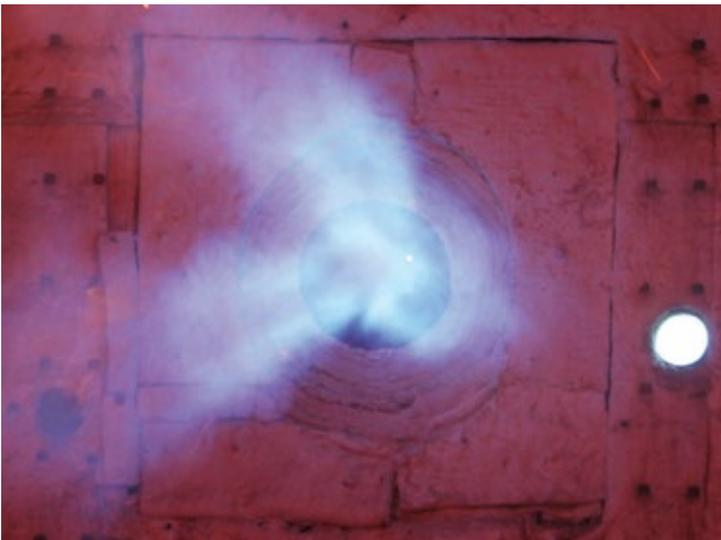
The ZEECO® GB low-NOx power burner fires a variety of gas or liquid fuels and supports multi-fuel applications without major combustion control or burner management system modifications.
