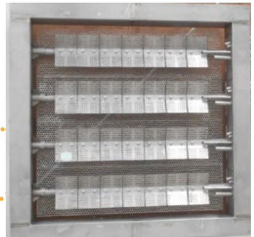
ZEECO DB-LN Duct Burner
