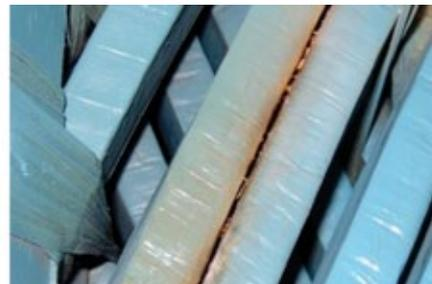
**2-6. Inadequate spacing** between bars in the end windings contributes to partial-discharge attack
