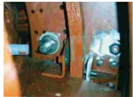
**1-15. Key-bar currents** want to connect through three parallel paths: core flange, core laminations, and frame components. OEMs have tried to bridge these currents via shunting straps and silver plating as shown
