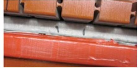
2-2. End-winding and slot partial-discharge indications are evident in this series of photos
