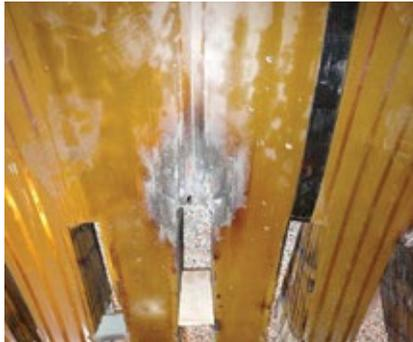
**1-2. With core iron removed**, the extent of heat penetration at the core melting locations is easy to see
