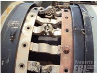
**B. Expansion and contraction of shunts** can lead to cracking and failure
