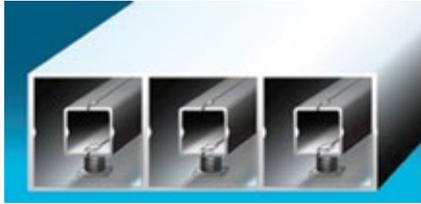
**3. In segregated-phase bus**, conductors for each phase are housed in a common metal enclosure but separated by metal barriers between the phases
