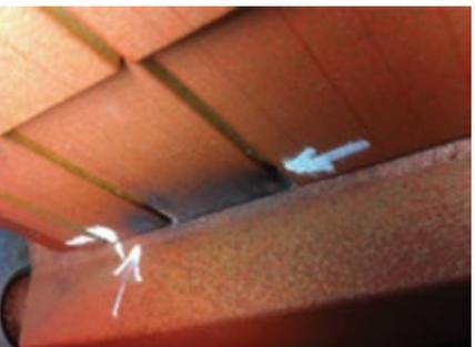
In either case, the key-bar currents want to connect through three parallel paths: core flange, core laminations, and frame components. OEMs have tried to bridge these key-bar currents via shunting straps and silver plating (Fig 1-15). But regardless of shunting attempts, the voltage is robust and will want to flow current in all three paths. This leads to the local burning between key bars and core iron shown in Fig 1-16.
