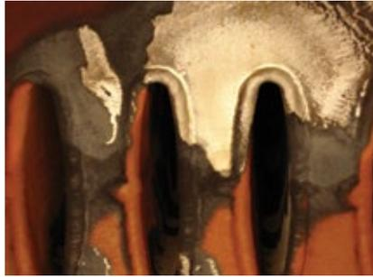
11. DHACI rating 4, serious corrosion at inlets to cooling tubes
