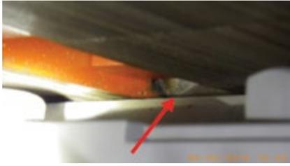
**1-17. Arc heating** occurred at the end of the core
