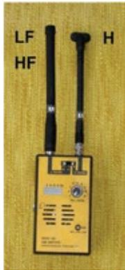
2-3. "Sniffer" is a special AM radio used to measure radio-frequency energy. Ear phones are necessary to hear an identify an EMI signal in high-noise environments
