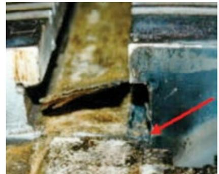
**4-5. Minor rotor-forging burn** damage in an area of low mechanical stress is relatively easy to correct by light grinding of field iron
