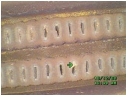
**2-7. Effects of restricted flow** caused by oxide formation are in evidence here
