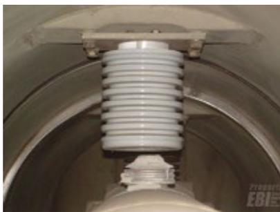
**A. Insulator failure.** Note that the ceramic insert is completely out of the insulator
