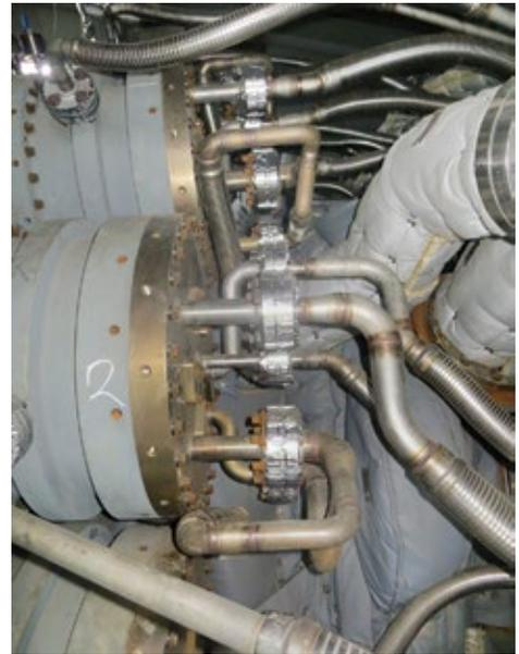
**3, 4. Field performance tests** showed the 7FA.05 combustion section exceeded expectations on output and heat rate, while meeting 9-ppm NO<sub>x</sub> emissions down to approximately 40% of the full-load rating
