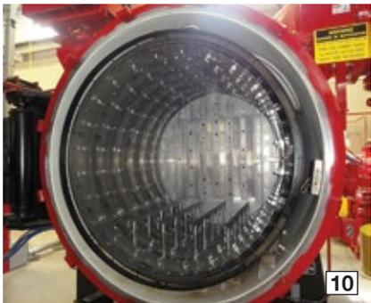
**7-10. Shop tour.** Metallic coating is applied robotically with high-velocity oxygen fuel (7); engineered rack (8) is constructed of Haynes® 230 material for high-temperature vacuum heat treatment without risk of airfoil positional movement on long turbine buckets/ blades; vacuum furnaces (9), internals in Fig 10, consist of all moly hot-zone construction rather than graphite. This provides the lowest oxygen content (ppm) during elevated temperature cycles
