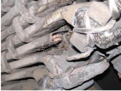
**1-6. Stator-bar fracture** caused a single phase-to-ground failure. Winding immediately tripped on ground relay, but current continued to flow through the arc as field current decayed causing substantial damage (left)
