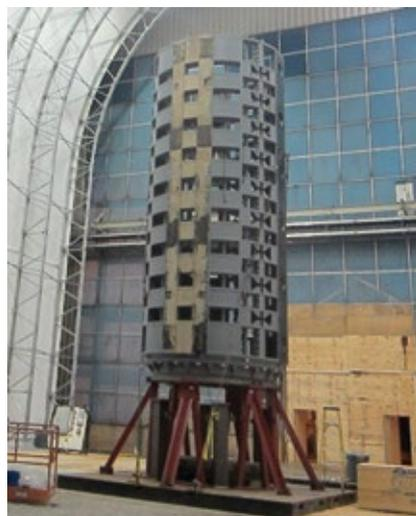
**1-5. Inner frame was upended** to install new a core in a “cage” machine—a long, complicated process
