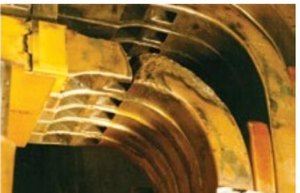
**4-6. Generator condition monitor** is very sensitive and will pinpoint the location of minor core overheating (left and center) and will easily detect at a very early stage any major damage (right)
