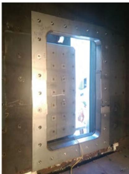
it. Obviously, at about 600 lb, it is too heavy for workers to remove by hand so a trolley system was installed to carry the weight. Jack bolts were installed to pull the door out of the hole and guide rails on the top ensure that the door comes out straight, minimizing the possibility of damage to the mounting studs.
