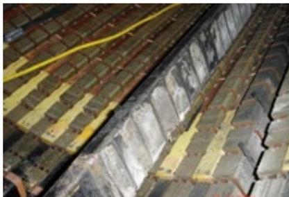
**2-4. Winding deterioration** was caused by bar vibration in the slot (vibration sparking)
