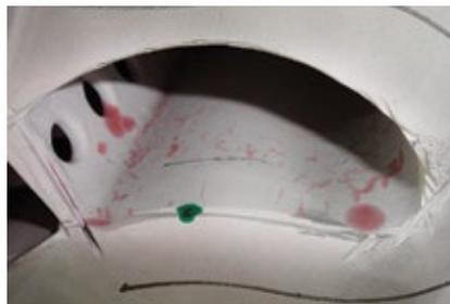
**5. Nozzles begin to fail** “from the inside out” after significant operating hours as red-dye crazing on the internal surface of this first-stage nozzle reveals
