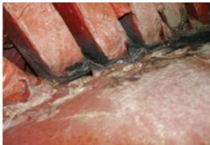
**2-5. Insulation delamination and tracking** in contaminants is shown here
