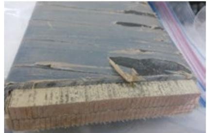
**1-9. Investigators identified severe internal and external partial-discharge damage on high-voltage bars.** Note damage to surface tapes and grounding paint
