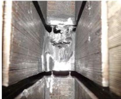
**1-1. Winding failure** was near the end of the core in slot 18. Some core grinding had been done before this photo was taken
