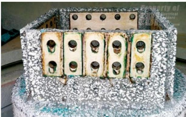
**11. Cracks in expansion joints** allow moisture ingress and severe corrosion can occur when excessive ground currents are present
