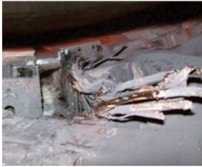
**4-2. Failure to ground** caused by the fracture of a stator conductor is not rare. Winding and core damage attributed to a burned open bar in a slot is shown at left and right, respectively
