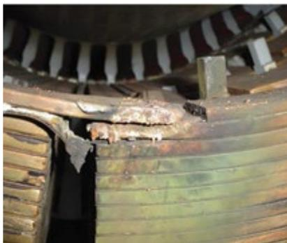
**3-1. Failure modes** discussed by Moore included the pole-to-pole crossover failure shown here
