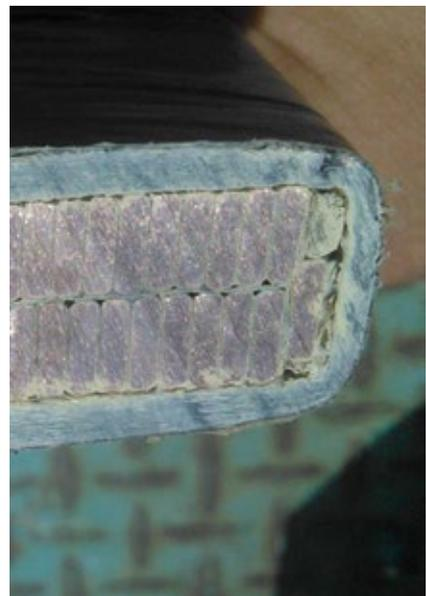
**1-11. Voids visible at the bottom of the bare bar** were caused by internal PD
