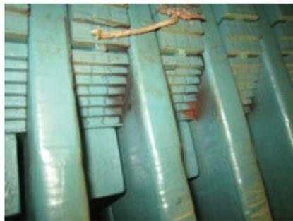
**1-14. There is a concern** relative to the top strands of the top bars at the core ends in generators of recent design that rely on large core-iron stepdown at the core ends
