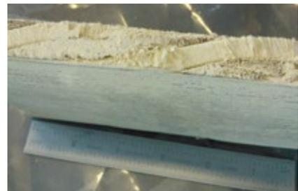
**1-10. Total destruction of internal insulating materials** is in evidence: Cross-over putty is completely eaten away and the strand insulation has been attacked
