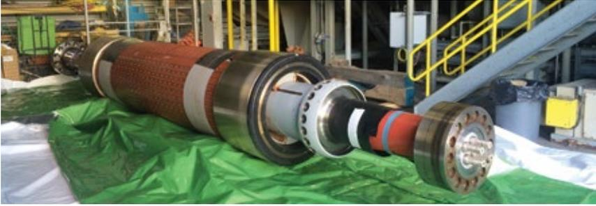
4. New generator rotor for the steam turbine replaced the existing one, which suffered a saltwater intrusion event and other issues
