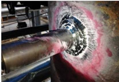
**4. Insertion-type thermowells** in SA106B carbon-steel piping rely on an Inconel weld filler
