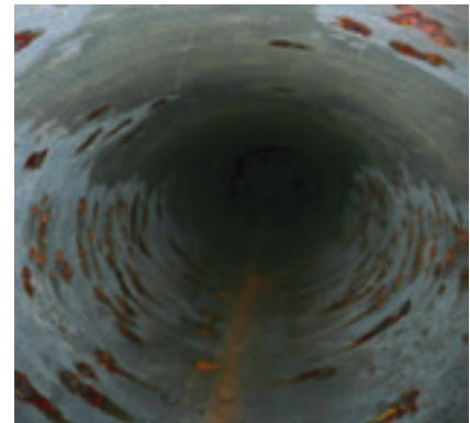
4. Breakdown of the passive oxide layer in an HP steam line that stood for six months without preservation treatment
