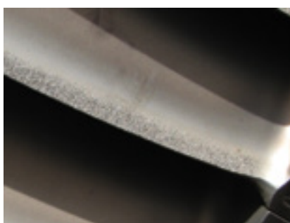
5. Trailing edge erosion of last-stage blades occurs at low loads
