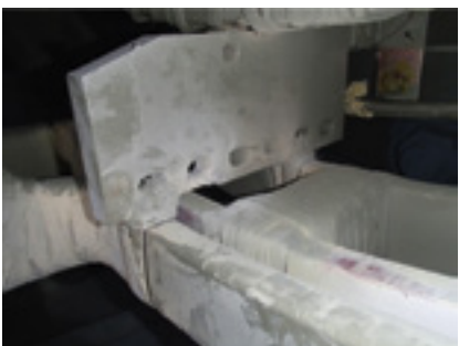
7. Dusting of ties and movement of the dummy ring and the A-phase jumper ties to the gunstock was clearly evident in Unit 2
