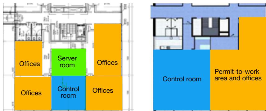
2. Control-room design concept proposed by company architects (left) was significantly different from the one proposed by the plant task force (right)—and accepted
