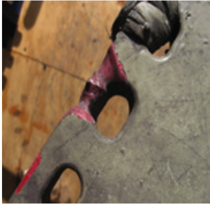
4. Broken tie and hole erosion in one of the gunstocks
