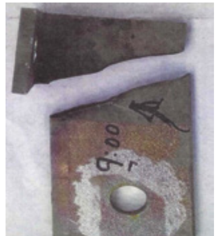
8. High-cycle fatigue cracks were found in Unit 2's axial support brackets
