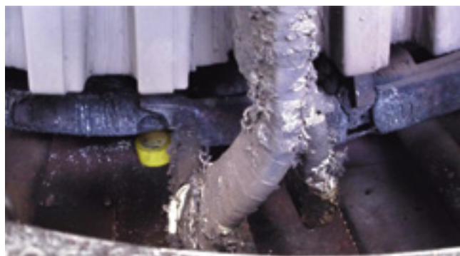
2, 3. Primary fault zone in Unit 1 was at the C- and A-phase jumpers to the connection rings, as shown from two angles
