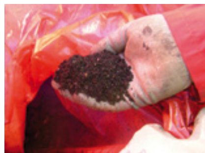
9. The sticky material on economizer gas-side surfaces was reduced to an easily handled waste product acceptable for environmentally safe disposal
