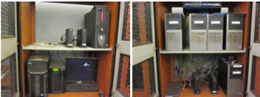
1. Virtualization enabled plant to remove significant hardware from behind the control-room workstations
