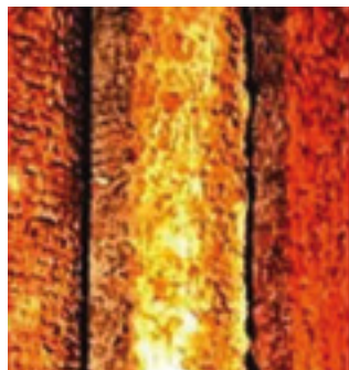
4, 5. Typical fouling and bridging of tubes before cleaning is shown at left. At right, the same tubes have been restored to “new and clean” condition by blasting with CO 2 pellets
