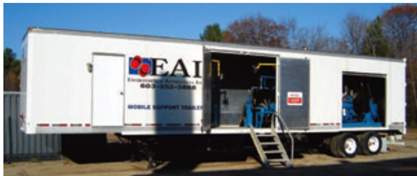
6. Mobile support trailer houses all the CO 2 blast cleaning equipment, produces the high-density pellets as needed, and carries support tools
