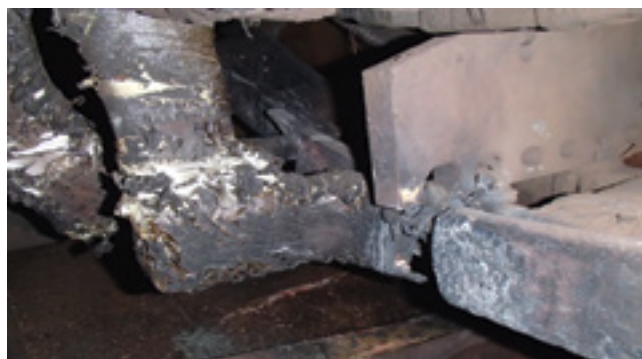
2, 3. Primary fault zone in Unit 1 was at the C- and A-phase jumpers to the connection rings, as shown from two angles
