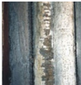
4, 5. Typical fouling and bridging of tubes before cleaning is shown at left. At right, the same tubes have been restored to “new and clean” condition by blasting with CO 2 pellets
