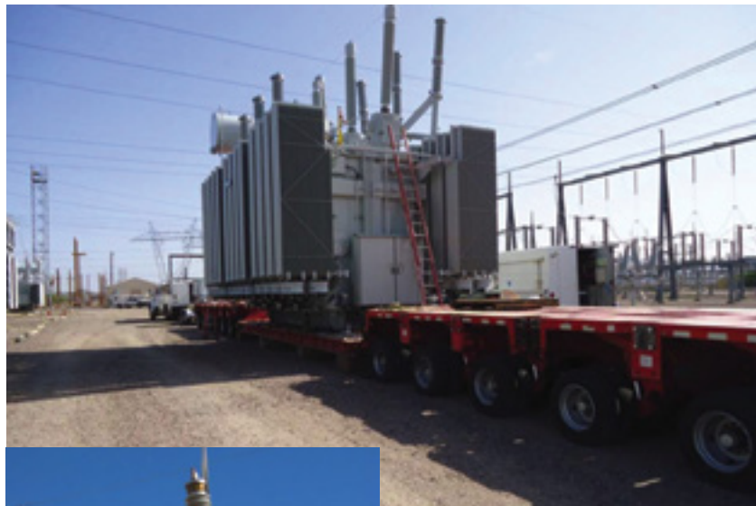
A. Transport of large transformers can be challenging. While many units can be shipped by rail car, some must be trucked to the site
