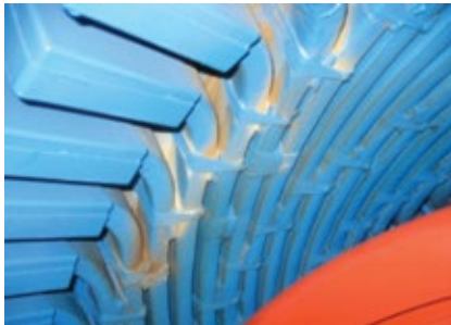
1, 2, 3. Dusting is indicative of early-stage vibration in endwinding
