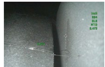
4. Measurement of blade clearances is possible only with 3D PM
