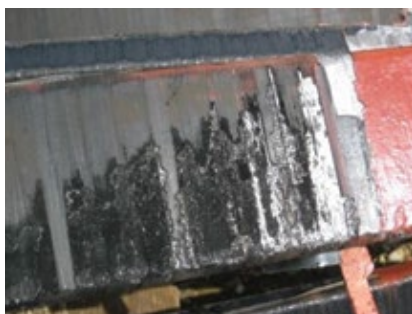
3, 4. Vibration sparking is a fast-acting destructive phenomenon as evidenced by bar damage at left and side-packing damage at right
