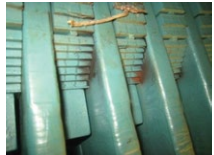
14. Side forces on the top bar likely caused the vibration that led to dusting
