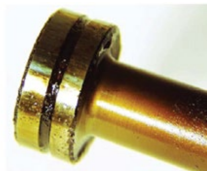
1. Varnish is shown here in its insoluble form
