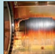
Varnish on journal bearing, gas turbine
