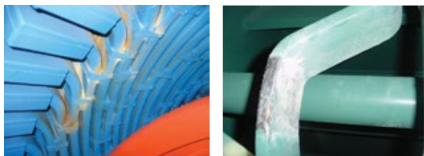
5, 6. Dry ties generally have not performed well in endwinding support systems. At left is dust generated where ties have failed; at right, bare copper is exposed from wear associated with dry ties
