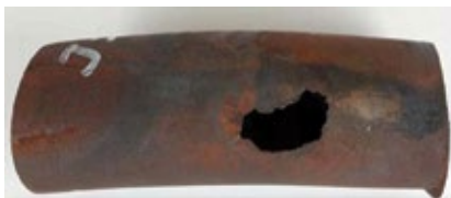
3. Two-phase flow at bend in LP evaporator tube caused this failure
