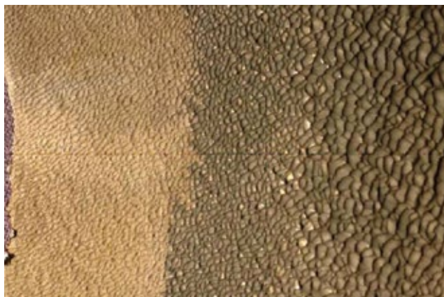
2. Worn belly plate was removed from an LP drum exposed to two-phase flow
