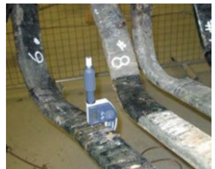
18. Small coil-wound generators made with inappropriate asphalt material post-1970 reintroduced the failure mechanism illustrated in Fig 17. In photo, the remaining groundwall measured 20% of original thickness
