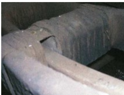
9. Questionable blocking of connection rings was in evidence on a winding that failed in service
