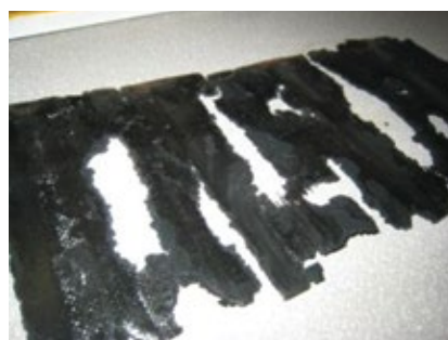
3, 4. Vibration sparking is a fast-acting destructive phenomenon as evidenced by bar damage at left and side-packing damage at right
