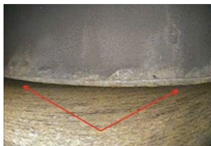
8. Compressor rotor blade exhibits rolled metal
