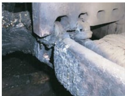
8. Arc damage was caused by failure of connection-ring insulation
