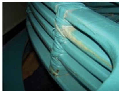
4, 5. Early-stage vibration of connection rings is identified by dusting
