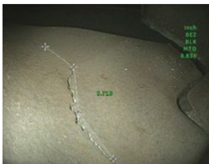
11. Extent of damage to a second-stage bucket tip shroud is measured
