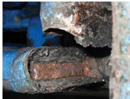
12. Arc damage resulted from copper fatigue failure of a connection ring
