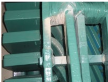
4, 5. Early-stage vibration of connection rings is identified by dusting
