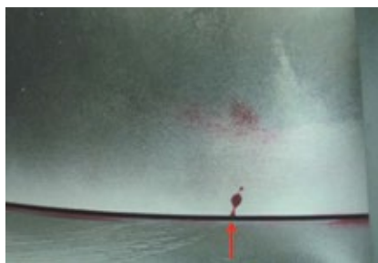
9. Rotor-blade tip cracks are easy to spot with dye penetrant
