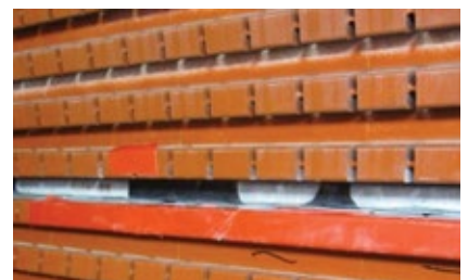
19. Slot partial-discharge activity is in evidence on this modern air-cooled generator
