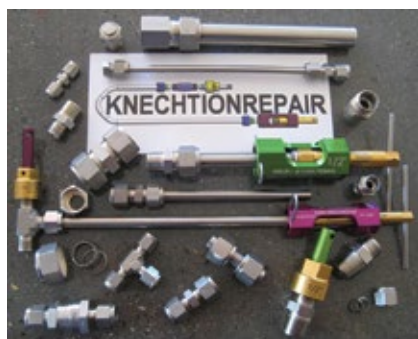
2. Tool set for repairing cross-threaded compression fittings quick!
