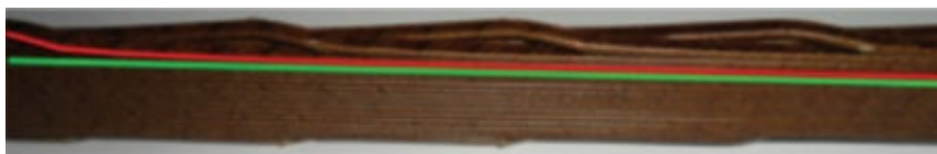
1. Copper strands are Roebelized together to form modern mica ground-wall generator bars
