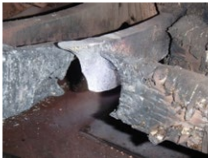
10. Arc damage was found at the joint between the stator bar and connection ring
