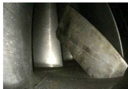
10. Protruding stator vane shim should be machined flush with the platform or removed
