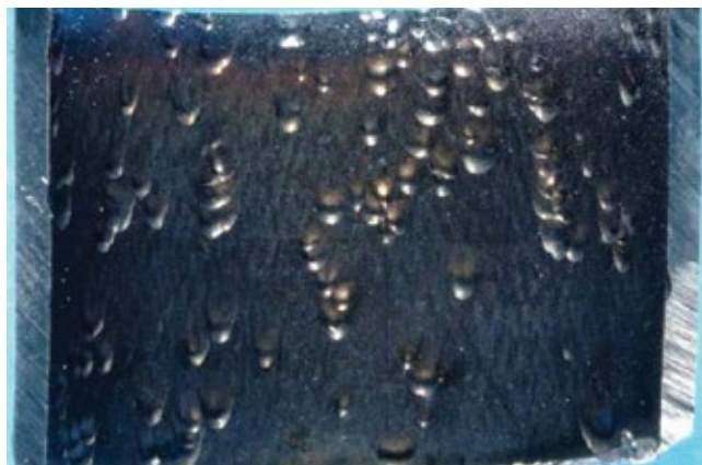
1. Single-phase FAC as seen in an HRSG tube
