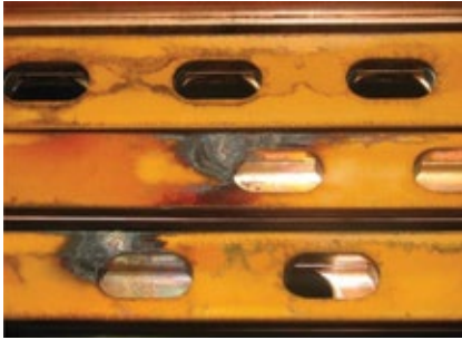
20. Strand shorts in a direct-cooled field are caused by contaminants entrained in cooling air
