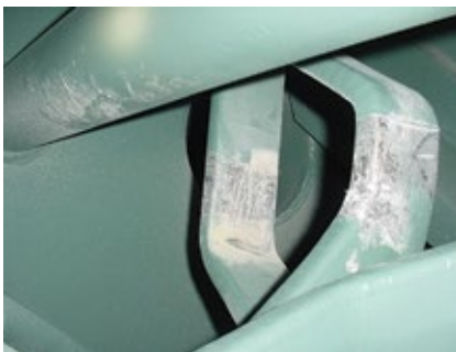
6, 7. Insulation wear on two rings in different phases is clearly problematic
