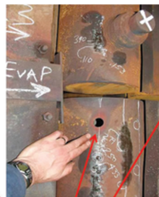
3. Hole in evap header (center) occurred directly above tube end (right). Header location in HRSG is at the left
