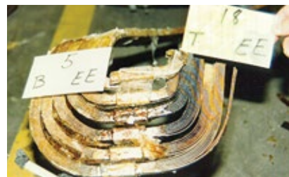
C. Major winding failure occurred from shorted strand groupings
