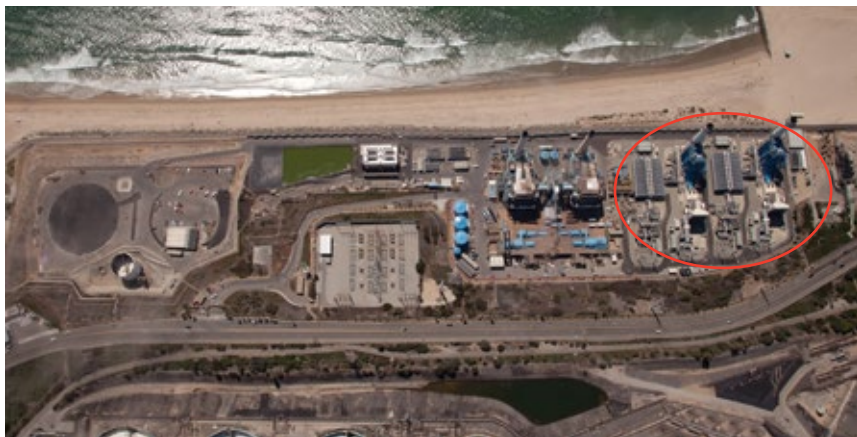
1. El Segundo's two new 1 × 1 gas-fired combined cycles (circle) are installed where an oil/gas-fired thermal unit once stood. Two more old units slated for removal are to the left of the new ones. The access drive from the coastal highway snakes around the substation; a massive petrochemical complex is on the other side of the highway (foreground). Diagram illustrates arrangement of key components in El Segundo's single-pressure non-reheat steam cycle
