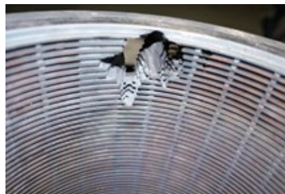
8. Bypass-valve disc-stack damage occurred on all three units at Darling Downs
