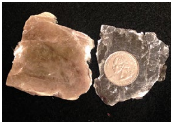
1. Raw mica is processed, and applied to tape or paper with resin, for use as an insulator
