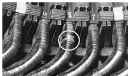
A. Tape separation of 0.75 in. (circle) was caused by migration of groundwall insulation
