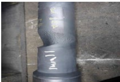
7. Stop-valve stem damage was attributed to plastic deformation, erosion, and/or corrosion
