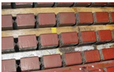
B. Significant surface partial discharge is in evidence in the slot
