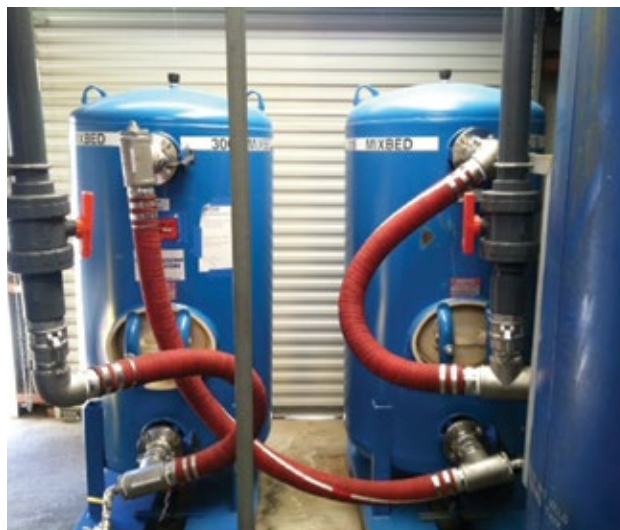
2. Original arrangement of 16 mixed-bed bottles jammed in a stationary truck trailer (left)
