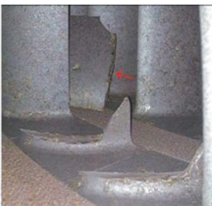
2, 3. S17 stator-vane (left) and exit-guide-vane liberations (right) were easy to identify during borescope examinations
