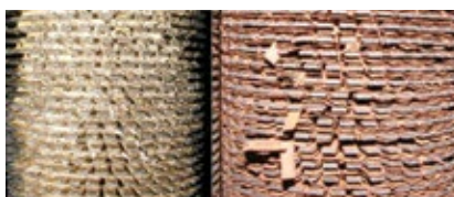
5. Long layup for repairs contributed to fouling of finned tubes—salt deposits at left, rust at right
