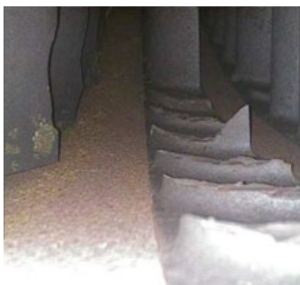
2, 3. S17 stator-vane (left) and exit-guide-vane liberations (right) were easy to identify during borescope examinations
