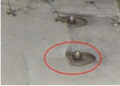
**7. Engine vibration** and the use of flat washers for attaching insulation to the exhaust casing limit insulation lifetime
