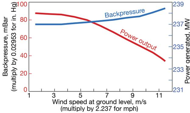
**7. ACC performance** falls off as wind speed increases. Results are for a 750-MW combined cycle operating at 50F ambient
