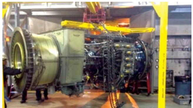
6. When rolling out the engine, the speaker's experience suggests having a person at each corner. The challenge at this site was the reduced clearance between grade and maximum engine height because the package was installed below grade
