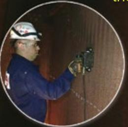
OD Scanning for Tube Wall Thickness
