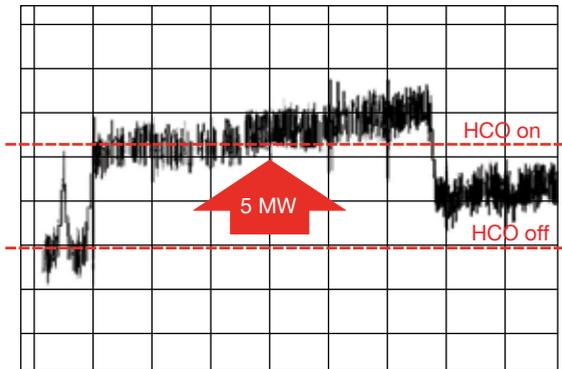
**5. Hydraulic clearance optimization** feature available on some Siemens gas turbines controls blade-tip clearances automatically by way of hydraulic pistons located behind the compressor thrust bearing
