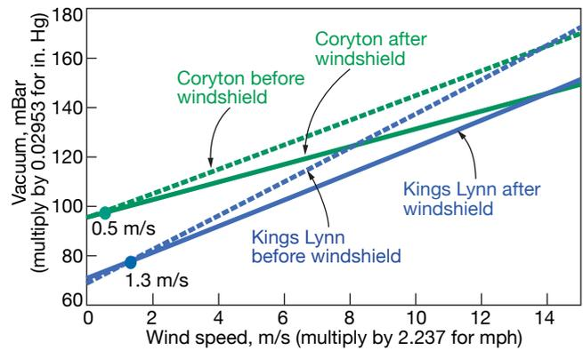
**8. Impact of wind speed** on vacuum at two ACC-equipped UK generating plants
