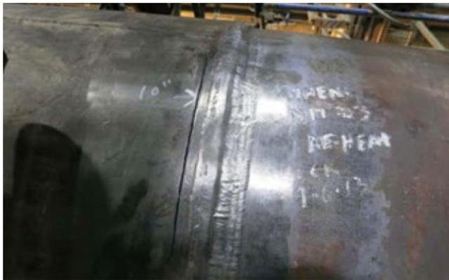
**1. Desuperheater weld crack** developed about 1 ft downstream of spray nozzles
