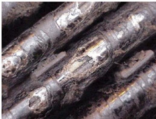
**12. Cleaning of generator stator insulation requires care. Photo illustrates what can happen when blast pressure is too high**
