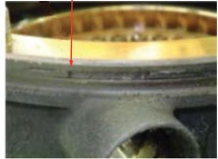
**1. Arrangement of the frame, sump, and pressurizing air passage at the back end of an LM6000 shows where O-ring seal damage has been found**
