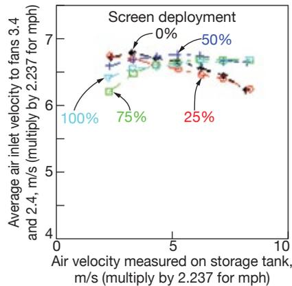
**15. Effects of wind speed** and wind-screen deployment on the average air inlet velocity to fans 3.4 and 2.4 are illustrated in the chart. Note the positive effect of the screen at higher wind speeds and its negative effect at lower wind speeds. Breakeven is about 9 mph (4 m/s). Best results are achieved with 50% screen deployment (up to a wind velocity of 18 mph)
