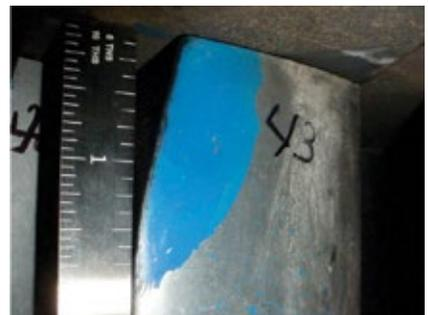
**3. Leading edge of stationary vane** was removed by contact with rotating blades
