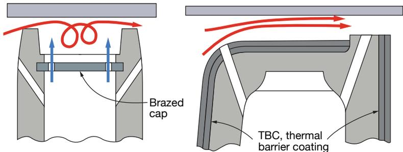
**4. Computer modeling** of tip leakage for turbine blade with conventional squealer tip is at left. Squealer tip design for original 501F first-stage turbine blade (center) caused turbulence conducive to cap cracking and oxidation. Elimination of the squealer tip on one side of the 501F blade (right) smoothed out the flow, contributing to fewer repairs, longer life
