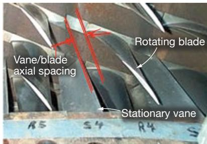
**1, 2. Clashing occurs** when the tip of a stationary vane moves forward more than half an inch and contacts passing rotating blades near their platforms
