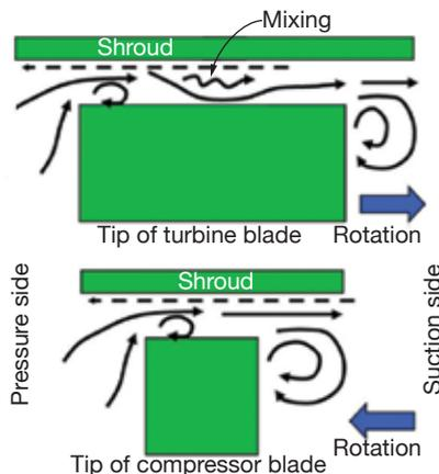
2. General leakage flow over the tips of turbine and compressor blades is basically the same
