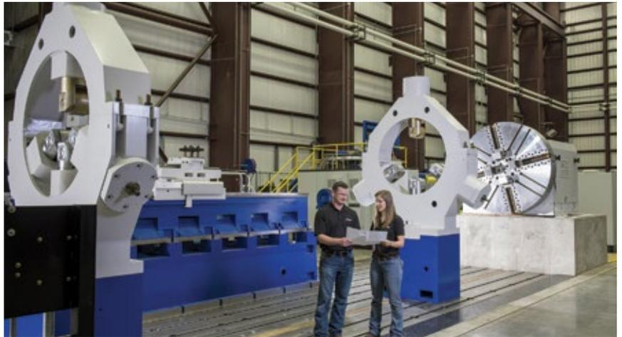
**Sulzer expands its machining capabilities** with a state-of-the-art lathe specifically designed for versatility and to accommodate rotors from the latest gas turbines. Capacity is 100 tons, length is 76 ft over bedway, swing is 14 ft
