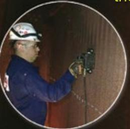
OD Scanning for Tube Wall Thickness
