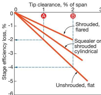
3. Effect of clearance on turbine efficiency is defined for various blade-tip designs
