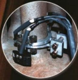
Claw Tool for Tube to Header Weld Cracking
