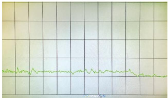
**3, 4. ACC vacuum swings were dramatic** prior desuperheater replacement (left). After replacement, vacuum stability improved dramatically, restoring steam-turbine output to the design spec (right)
