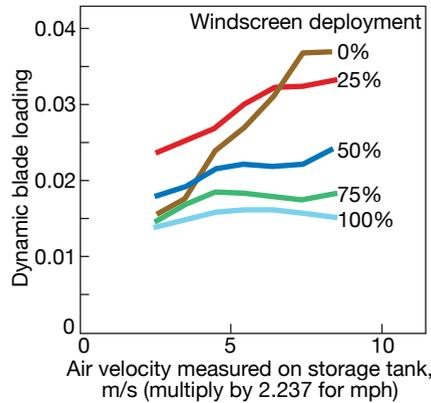
**16. Effect of wind speed** and wind-screen deployment on the dynamic blade loading of fan 3.4 reflects highest loading at highest wind speeds. Screen deployment reduced dynamic blade loading by a factor of from two to three
