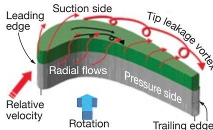
1. Behavior of leakage flow over a turbine blade with a flat tip
