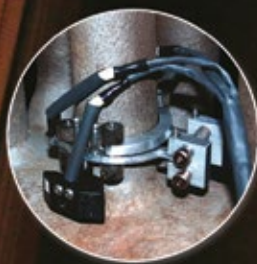
Internal Crawler for Visual and Tube Thickness from the Tube ID
