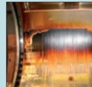
Varnish on journal bearing, gas turbine
