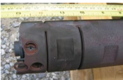
2. Probe-type desuperheaters in cycling units are prone to fatigue failure
