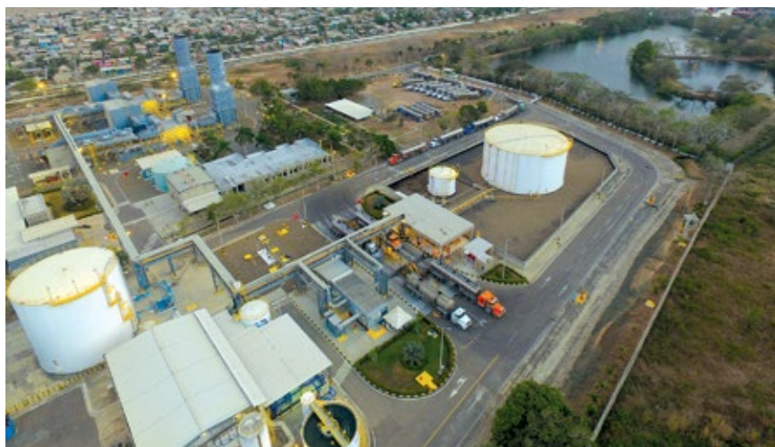
1. Delivering fuel oil to Termocandelaria at full capability reveals four trucks at the unloading station, several others in the queue to the left of the large oil tank, and several others in the parking lot at the top center of the photo
