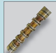
Varnish on valve spool
