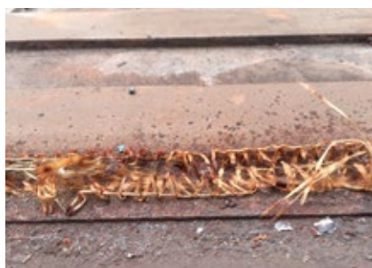
5. Gasket material around the roof of this SCR unit was found in a completely degraded condition
