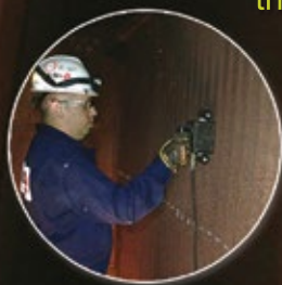
Internal Crawler for Visual and Tube Thickness from the Tube ID
