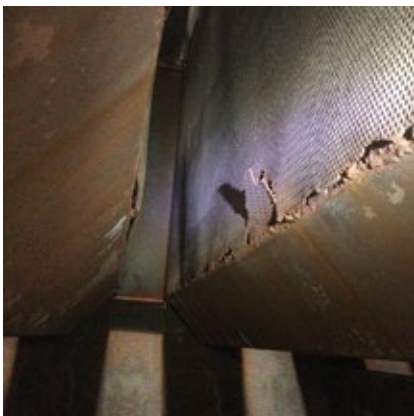
5. Baffles tearing away from frame/damaged
