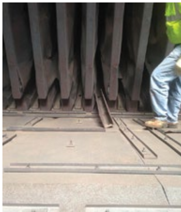
4. Internal liners and channel guides: poor
