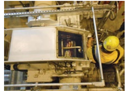
HP steam-turbine module (left) is geared to 3600 rpm (above)
