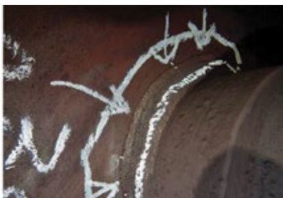
4. Cracks are discovered with greater frequency in such drum penetration welds as the cracked riser nozzle weld (top) and the blowdown nozzle
