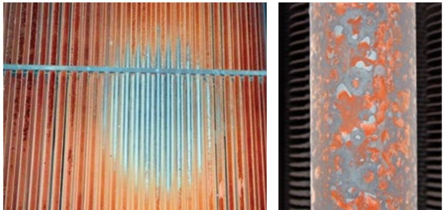
**5. Overheat zone** is clearly visible on panel at left; impact of overheat on tube internal surface is at right
