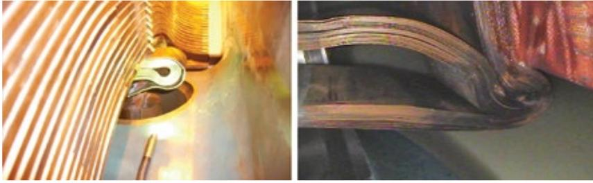
**31. Broken J-straps:** Complete J-strap separation from main terminal stud is at left; a deformed, collapsed J-strap is at right
