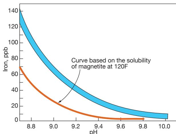
**1. Dooley/Aspden relationship, important to ACC operation, graphs the relationship between pH and total iron.** Note that ammonia was used exclusively for pH control in this case; iron levels were measured at the condensate-pump discharge. Data for iron solubility are attributed to Piero Sturla of ENEL's Piacenza Laboratory (1973)
