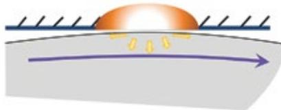
**38. Rubbing between stationary and rotating parts causes frictional heating. Heat flows inward as illustrated**
