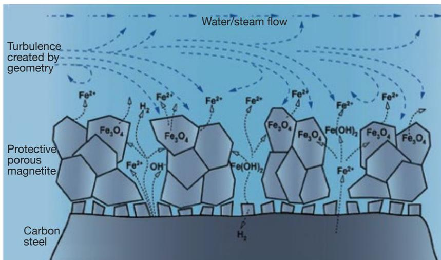
**2. Two-phase FAC** (steam and water) is a consequence of a flow-accelerated increase in mass transfer of dissolving and reacting species at a high-flow or highly turbulent location
