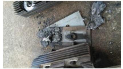
**30. Parts liberated** from failed fuses damaged the wheel itself
