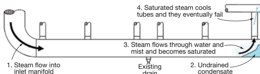
5. Root cause of the failures in Fig 4 was water collecting in the lower header at the end of the tube bundle
