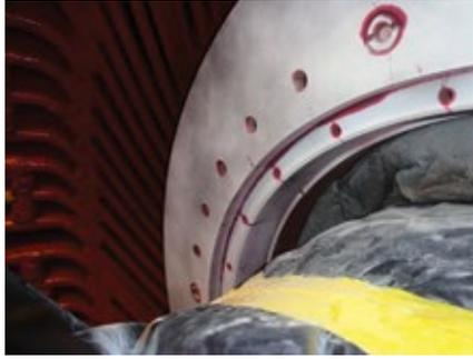
**37. Red-dye confirmation of cracks is shown at left and right**
