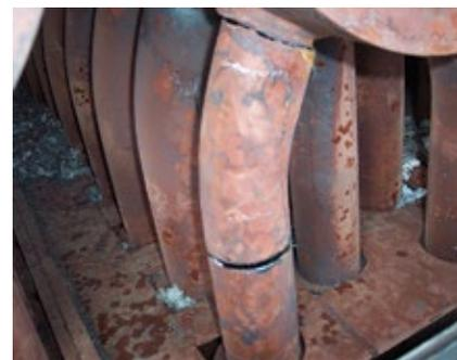
4. Several tubes failed in the HRSG reheater bundle next to the outer wall of the unit
