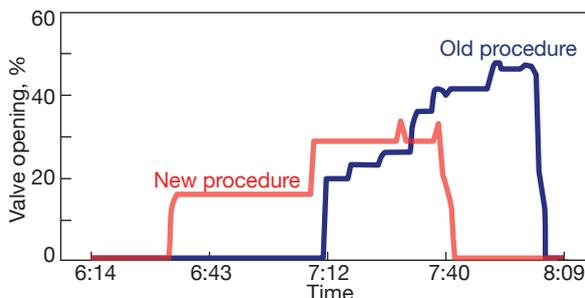
**2. Reduction in steam venting during startup saved a significant amount of water**
