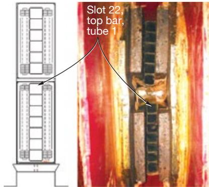
**1. Bar cross section** for this hydrogen-cooled generator is illustrated (left) and shown in the photo (right)
