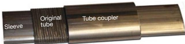
**8. Tube sleeve inserts** and outer couplers are one way to eliminate leaks (above)
