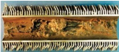
**23. Under-deposit corrosion leads to tube failures**
