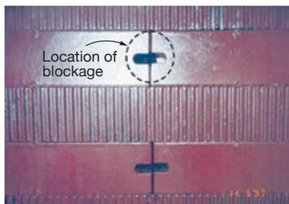
**42. Blocked ventilation passages** can contribute to rotor thermal sensitivity issues
