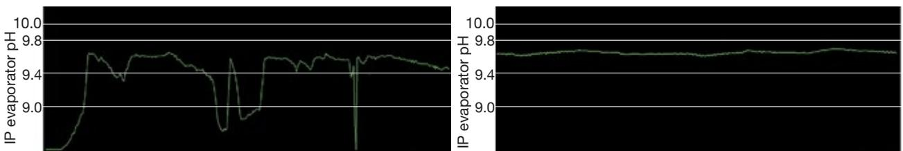
9, 10. IP evaporator (left) operated with unstable chemistry. Monitoring improvements led to stable chemistry (right)
