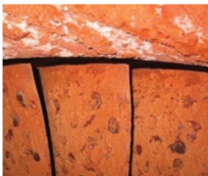
**24. Salt deposits in LP turbine attributed to a condenser tube leak (left)**
