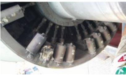
**29. Diode wheels** suffered significant damage. All fuses on the inboard wheel were open
