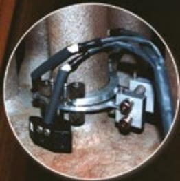
Claw Tool for Tube to Header Weld Cracking
