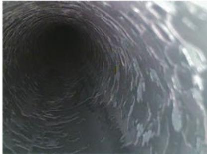
**6. Oxide exfoliation** of tube external surface is clearly visible at left, internal surface (via borescope exam) at right. Exfoliation is an indicator of overheating
