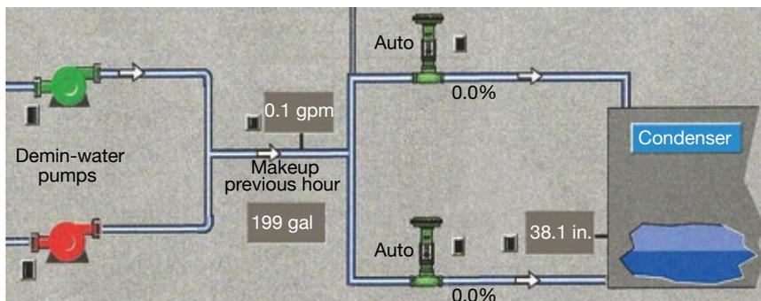
3. Monitoring of condenser makeup flow warns plant personnel of leaks
