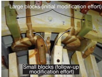
**28. Repaired joint** features added support stiffness to increase phase-bar natural frequency
