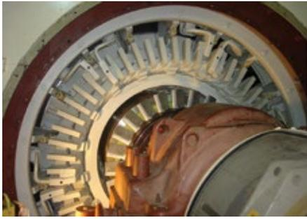
**25. Original end winding** showing phase-bar blocking design is at left; close-up at right. Supports use rope ties and conforming felt layer
