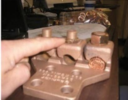
**33. Failed exciter lead connection** at left was corrected with an upgraded connector (right)
