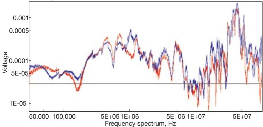
**5. Spectrum plot compares the same unit on dates two months apart.** Electrical activity increased between the first (red) and second (blue) scans
