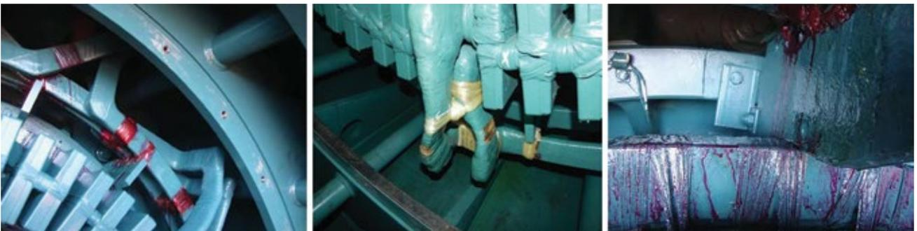
**35. Repairs to vibrating components** included replacement of connection-ring ties
