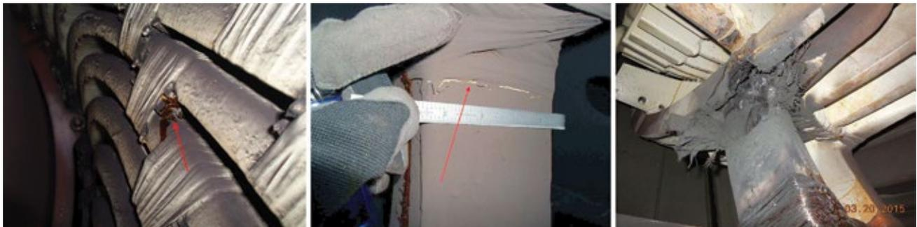
**11. Overheat damage** shown at left and in center led to the connection-ring failure at right
