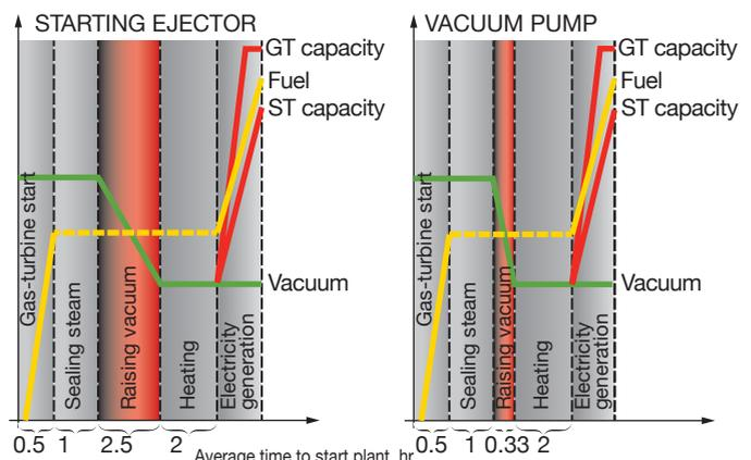
**3. Starting time with air ejector pulling vacuum (left)** required about six hours; with vacuum pump (right) about four hours
