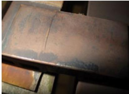
**21. Evolving crack in pole-to-pole connector**
