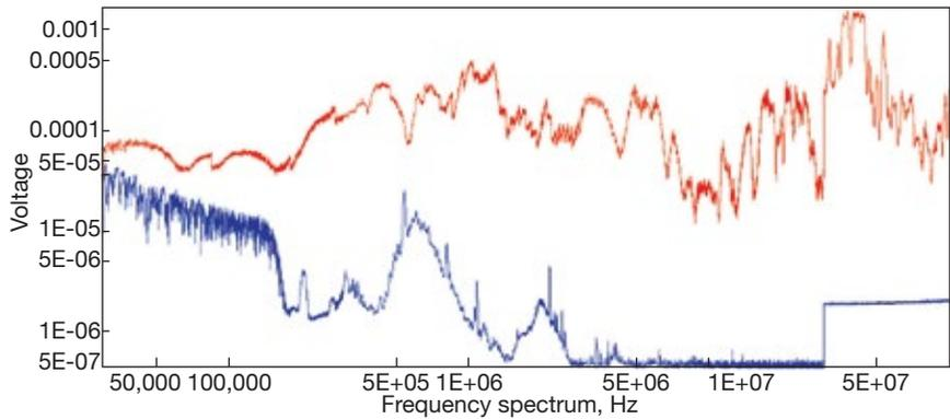
**4. Full-spectrum scans of sister units** are compared here. Red trace is of a unit that had significant vibration problems
