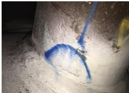
**11. Inspection identified cracking at the reheater header-to-manifold link**
