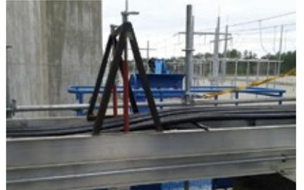
**2. Cable lifting rig** was designed and fabricated by plant personnel
