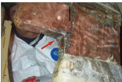
**6. Leak location** in connection-ring braze is identified by arrow
