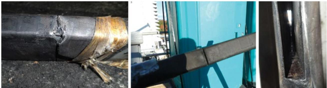
**10. Insulation was cut by inward migration** of the outside space block (left and center). Core damage at slot 1 is shown at right
