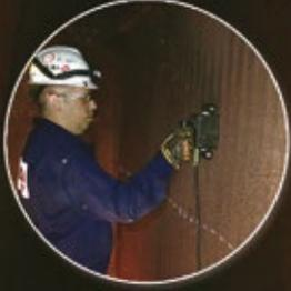
OD Scanning for Tube Wall Thickness
