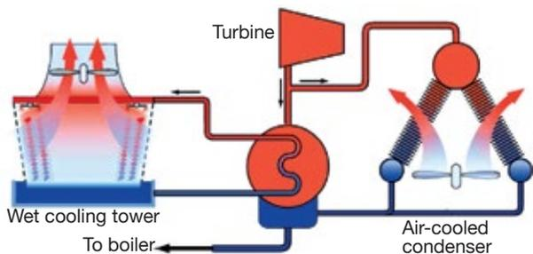
**3. Hybrid cooling** (wet and dry) is illustrated conceptually at the left, in service at right
