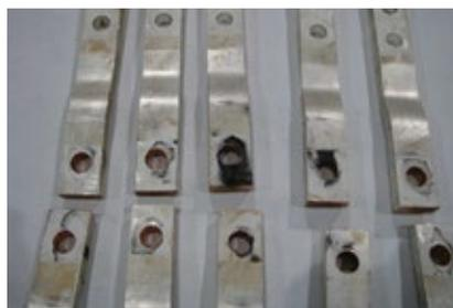
**7. Arc damage** on connection-ring flexible connectors is significant
