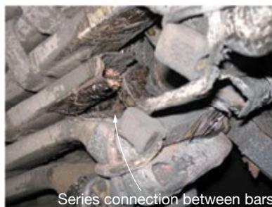
13. Failures resulting from endwinding vibration can cause considerable collateral damage
