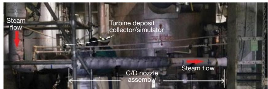
**1. Test loop** simulates LP-turbine expansion using a converging/diverging (C/D) nozzle (top). Results indicate filming amines and products can offer significant corrosion protection against contaminants as shown by the two sets of test strips (middle). Photo of the test setup is at the bottom
