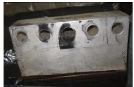
**8. Arc damage** on connection-ring tang is easy to identify
