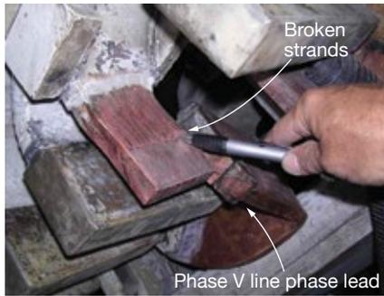
**27. Cracked strands** at the top of the pen at left are shown in detail at right
