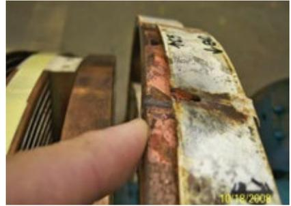
**32. Flux density test** revealed shorted turns in a large coil. Root cause was movement of turn insulation
