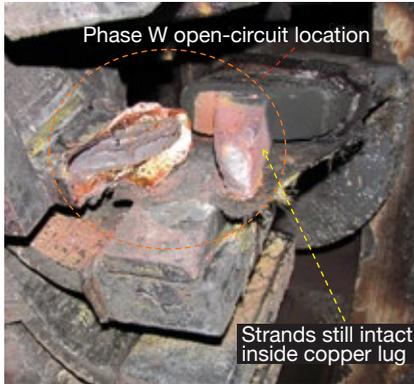
**26. Failed joint** reveals extensive burn damage
