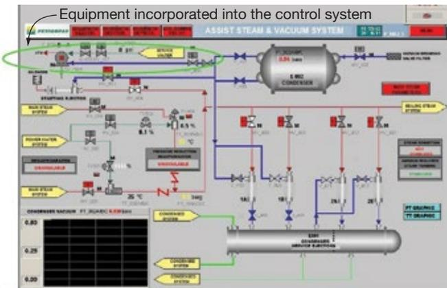
**2. Equipment incorporated into the DCS** to provide tight control over vacuum-raising is highlighted in the diagram
