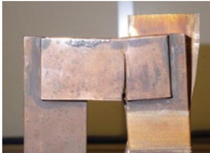
**22. Severe tear in pole-to-pole connector**
