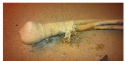
**18. Tape insulating** a connection joint wore away over the years and caused a hard ground
