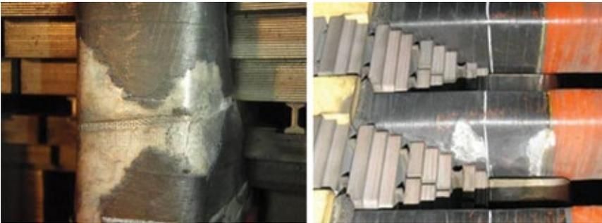
**16. OCP (outer corona protection) erosion** is shown on bars (left) and at core ends (right)
