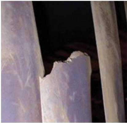
19. LP turbine L-0 blade failure
