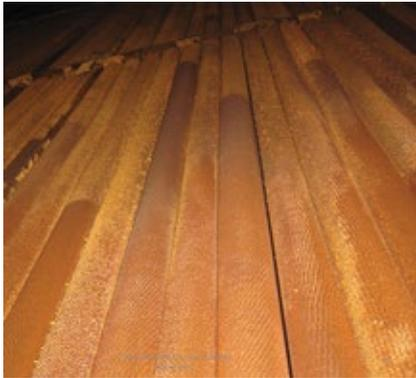
**2. Iron oxide (corrosion)** is a typical source of HRSG external tube fouling
