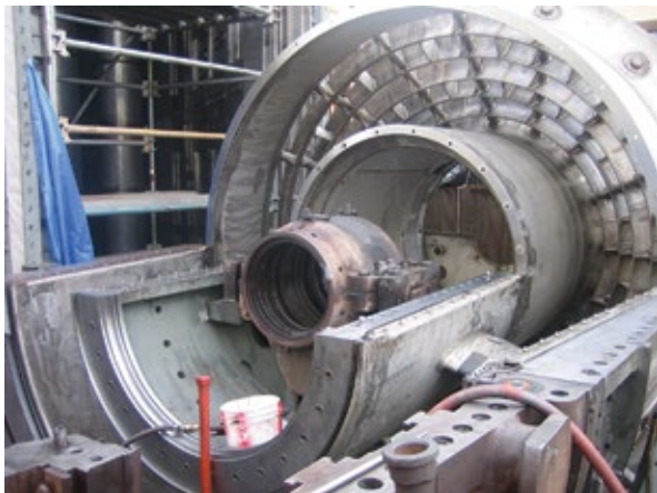
3. The exhaust section of a high-starts engine takes a beating over the years and typically is upgraded or replaced after about three decades of service
