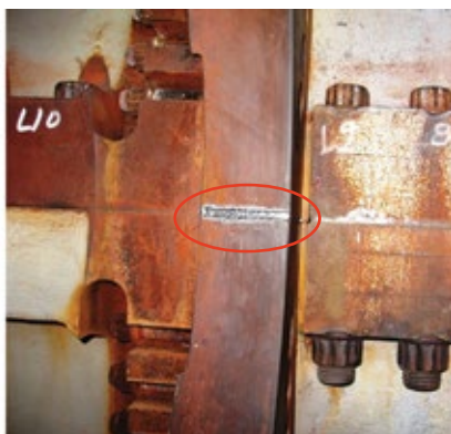
15. Peening is an alternative to welding for mitigating wrapper leaks
