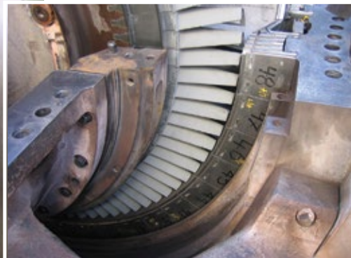
1, 2. Runout check (left) and replacement of first-stage buckets (above) typically are included in the refurbishment plan for a high-hours/high-starts 7B turbine rotor
