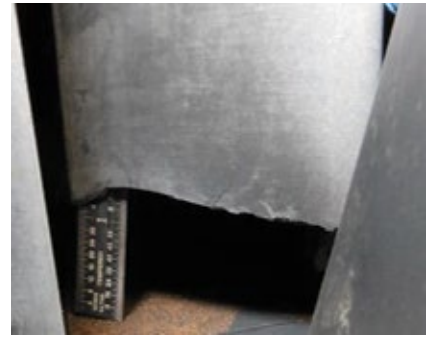
5. Tip was liberated from this S1 vane. Such potential damage is not addressed in either TIL 1884 or 1980
