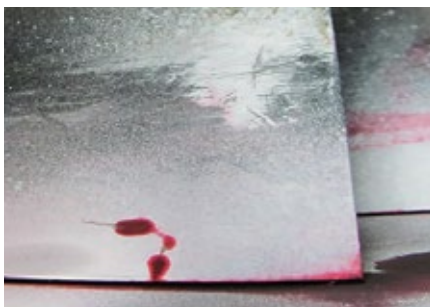
10. Rotor-blade radial tip crack like that at left can be removed in-situ (first and second stages) in one shift as shown in the center photo. Allowing the crack to propagate can lead to a tip liberation like that at right, with consequent downstream damage
