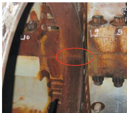
15. Peening is an alternative to welding for mitigating wrapper leaks
