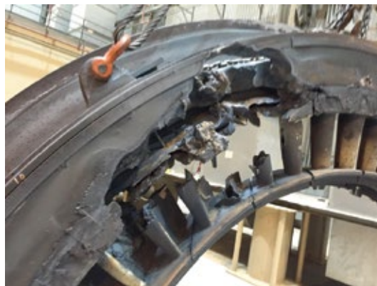
1. Blade ring was destroyed by hot gas following the liberation of ring segments
