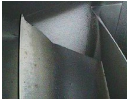
6, 7. Clashing damage experienced in the second (left) and third (right) stages remains unaddressed in a TIL
