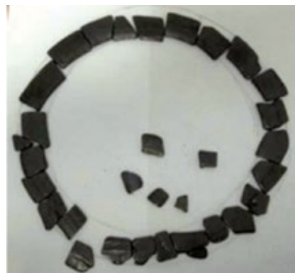
8. Hardfacing debris was removed from the strainer of a combined stop and control valve. Were the strainer to fail, as sometimes happens, this would wreak havoc in the steam turbine
