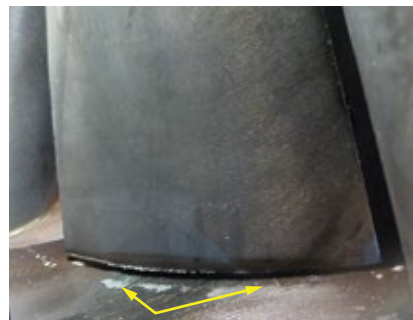
9. Rotor-blade tip distress is most commonly caused by rubs against the case during operation. Result may be discoloration or heat-affected zone at left or rolled metal at right
