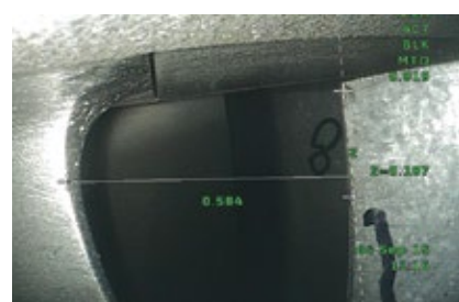
2. Precise measurements enable meaningful trending of damage progression year over year. Here, the distance between the trailing edge of the rotor-blade platform and the leading edge of the stator-vane tip is measured
