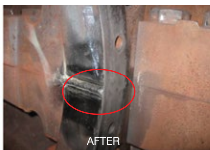
13. Welding of wrapper joints is an alternative leak-mitigation method. Here the inner split-line gap is in evidence (left) with Can 3 removed. After welding (right) the weld area must be machined even with the flange face
