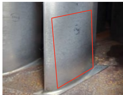
3. Area of interest is outlined on stator vane at left. Dye penetrant inspection identifies cracks in an S1 vane at right
