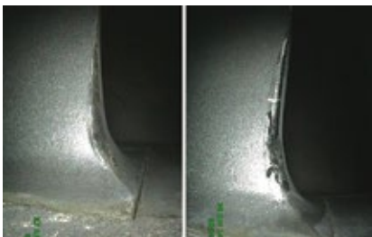
5. Clashing damage to the trailing edges of R1 rotor blades can range from rub marks shown at left to torn and displaced metal (right)
