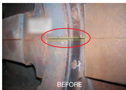
13. Welding of wrapper joints is an alternative leak-mitigation method. Here the inner split-line gap is in evidence (left) with Can 3 removed. After welding (right) the weld area must be machined even with the flange face
