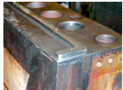
16. The OEM's "original" seal key modification was rated by users as time-consuming and costly to do and "unsuccessful"
