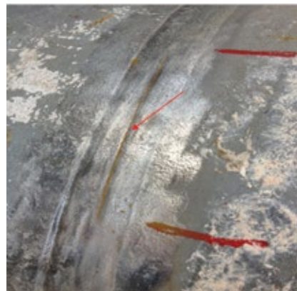
7. Mag-particle test reveals crack indication on the downstream weld of a tee
