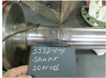
6. Damage to hard parts is caused by infrequent maintenance intervals and deterioration of soft parts
