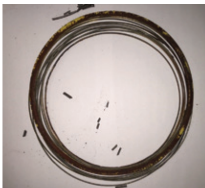
3. Flange, typical of those in ninth- and 13th-stage extraction lines (left), was broken to replace damaged gasket at right
