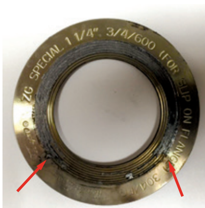
2. Technician points to the ring header-to-pigtail flange (left) where the gasket (right) was damaged and allowing leak-by
