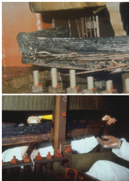
3. Saturation caused overheating in this transformer, irreparably damaging its winding
