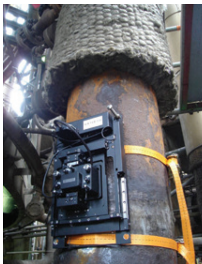
4. SFM in use on a P22 pipe at a refinery in Italy
