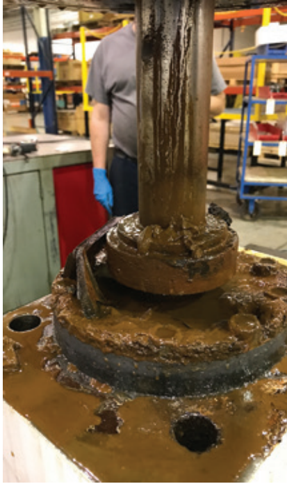
2. Steam leaks and moisture inside spring can contribute to rust and broken springs
