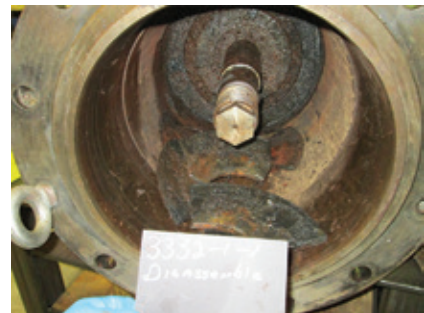
7, 8. Keeping moisture out of spring cans helps prevent broken springs and shaft damage
