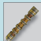
Varnish on valve spool
