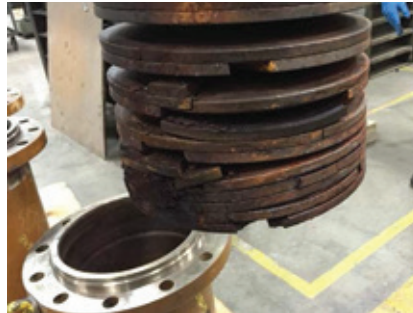
7, 8. Keeping moisture out of spring cans helps prevent broken springs and shaft damage
