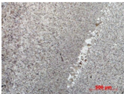
1. Ferrite phase found in fine-grained heat-affected zone/inter-critical HAZ in an aberrant P91 pipe
