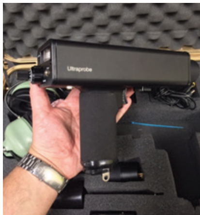
1. Ultrasonic leak detector is effective when the gas turbine is offline and in crank mode
