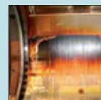
Varnish on journal bearing, gas turbine
