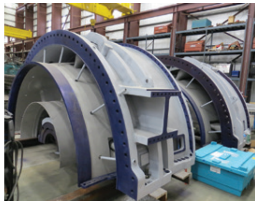
2. Repair/rebuild of exhaust sections is a significant part of DTS's 501F work today
