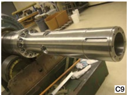
C7-C10. Collector failure and ground to the main shaft caused major arcing and heat damage to the end of the generator rotor forging, which could not continue in operation as found (Fig C7). The shaft was severed just outboard of the journal and bolt holes drilled and tapped for the new stub shaft (Fig C8). The assembled new shaft extension is in Fig C9 and the final assembly with fan and collector rings in Fig C10
