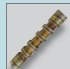
Varnish on valve spool
