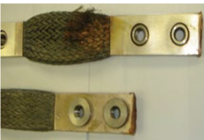
B31. Rubbing and/or abuse damaged these flex braids
