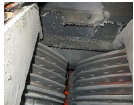
B26. Burning of gasket/sealing materials produced a heavy layer of soot
