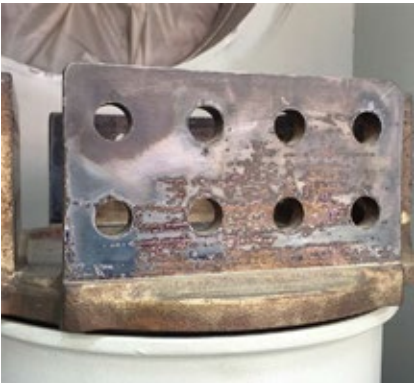
B29. Arc damage is revealed on a bolted joint's bus face
