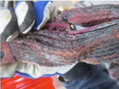
B28. Some flex links were found in a frayed/degraded condition
