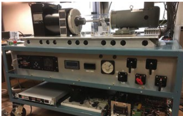
D1, D2. Mini turbine/generator model for training took two years to complete but was worth the wait
