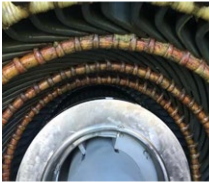
B11. Overall looseness in the endwinding structure is evident from the large amount of greasing
