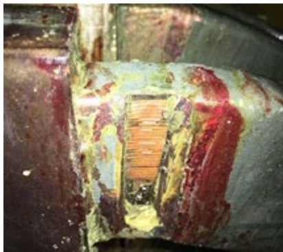
B15. Damage caused by excessive movement was corrected by reinsulating and securing with different material and methods than those used by the OEM
