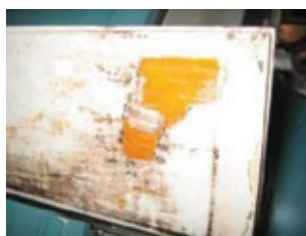
D18-D21. Impacts on rotors of cyclic duty include the failures shown in the photos above: slot-liner abrasion, insulation fracture, copper distortion, and blocked vent (left to right)
