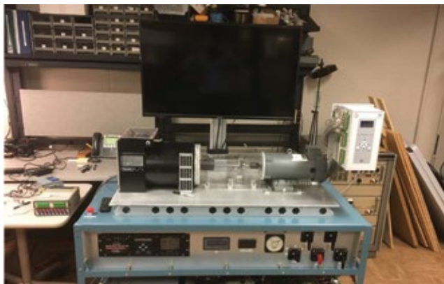
D1, D2. Mini turbine/generator model for training took two years to complete but was worth the wait
