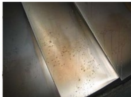
3. ODA treatment improved corrosion protection (condenser at left, last-stage turbine blades at right) during shutdown and had a positive effect on recommissioning at this steam plant
