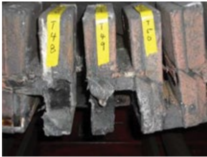
E3. Condensation on stator windings attributed to improper layup procedures caused unit to trip on restart after a planned outage
