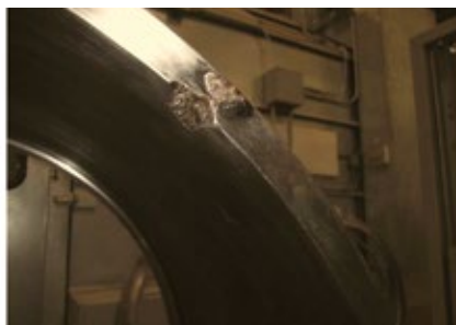
C1-C3. Negative sequence currents are a common and destructive phenomenon associated with generators. The result of these I_2 currents can be rotor body currents that can damage the rotor forging (left), retaining rings (center), and to a lesser degree, the field winding (right)
