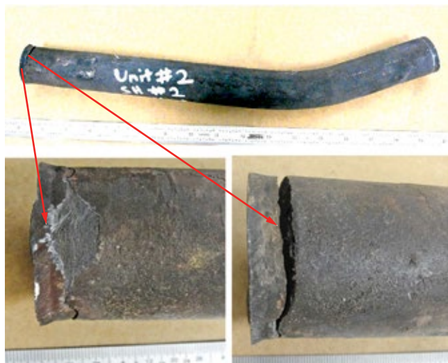
11. One of 73 failures in the upper header bent-tube rows experienced at an F-class plant
