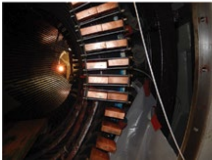
B5. Proper alignment of series connections were difficult to achieve because of bonding from the wet tie materials used
