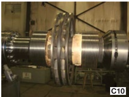
C7-C10. Collector failure and ground to the main shaft caused major arcing and heat damage to the end of the generator rotor forging, which could not continue in operation as found (Fig C7). The shaft was severed just outboard of the journal and bolt holes drilled and tapped for the new stub shaft (Fig C8). The assembled new shaft extension is in Fig C9 and the final assembly with fan and collector rings in Fig C10
