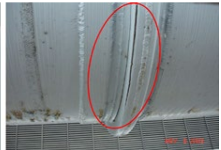
B33. Excessive movement of expansion bellows is conducive to cracking damage
