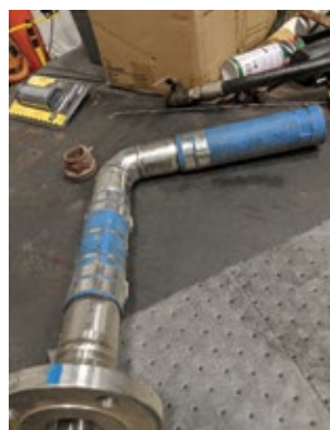
Original hose after failure is at the left, braided stainless-steel-reinforced replacement hose at right
