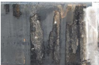
B3. Siemens Aeropac generator was rewound by Alstom because of the moderate-to-severe spark erosion in evidence
