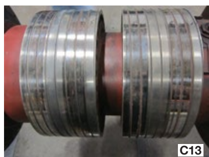
C11-C15. Typical conditions found during inspection of collector rings are threading (Fig C11), grooving (Fig C12), photographing (Fig C13), contamination (Fig C14), and heavy contamination (C15)
