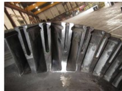
C4-C6. A double-ground fault caused severe arcing damage to the rotor, including melted material (refer back to Fig C1) and cracking on a tooth (left). The damaged portion of the tooth was removed (center) and replaced by weld build-up with appropriate heat treatment and re-machining of the tooth (right)
