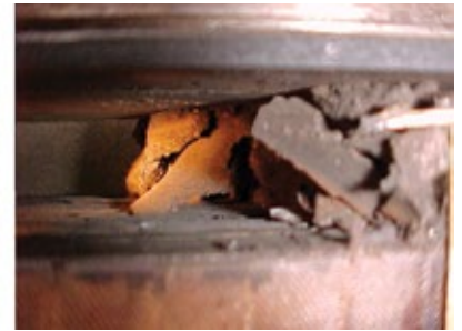
D8-D10. Rotor turn/coil shorts may not be a problem unless excessive; then they can be troublesome and destructive
