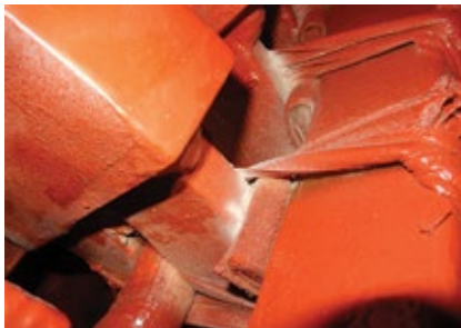
B8. Dusting is evidence of movement at the series connector interface with the outboard ring
