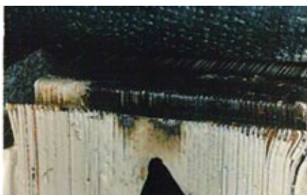
D3-D5. Causes of core failures include foreign object damage, lamination insulation failure (left), damage from repair work (center), and core looseness (right)
