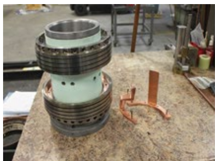
C20-C22. Major steps in replacing an old collector with a new one are shown left to right
