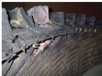
D14. Series connection braze failure caused a phase ground
