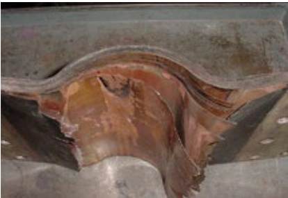
B30. Flexible connector's cracked laminations were caused by vibration or air flow
