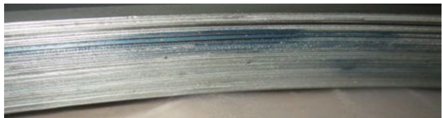
E8, E9. Rub marks are in evidence on air-side seals and shaft surfaces; plus, seals are out of round
