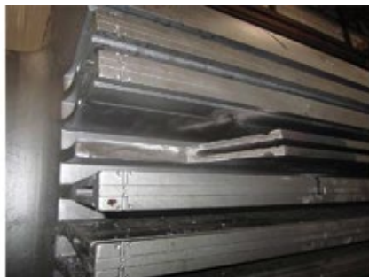
C4-C6. A double-ground fault caused severe arcing damage to the rotor, including melted material (refer back to Fig C1) and cracking on a tooth (left). The damaged portion of the tooth was removed (center) and replaced by weld build-up with appropriate heat treatment and re-machining of the tooth (right)
