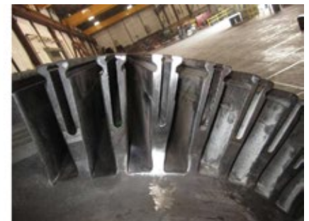
C4-C6. A double-ground fault caused severe arcing damage to the rotor, including melted material (refer back to Fig C1) and cracking on a tooth (left). The damaged portion of the tooth was removed (center) and replaced by weld build-up with appropriate heat treatment and re-machining of the tooth (right)
