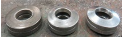
B27. The condition of Belleville washers used to secure phase links was called into question. Some had flattened out from repeated use, some had been installed upside down
