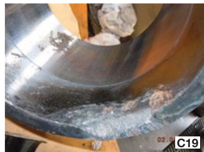
C16-C19. Problems resulting from collector-ring failure include burning caused by flashover to ground or severe arcing from poor maintenance (Figs C16 and C17 with brush holder removed), main-shaft damage caused by severe arcing to ground (Fig C18), and arcing damage to the ring ID (C19)
