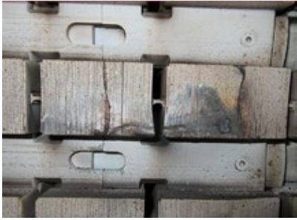
B19. Visual inspection of the stator identified several locations where overheating had occurred
