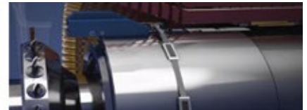
E6, E7. Retaining ring scanner at left and air-gap robot at right provide “eyes” to identify issues before they cause problems that can affect machine availability
