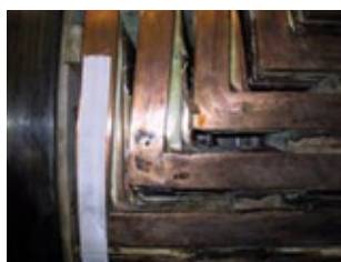
D18-D21. Impacts on rotors of cyclic duty include the failures shown in the photos above: slot-liner abrasion, insulation fracture, copper distortion, and blocked vent (left to right)
