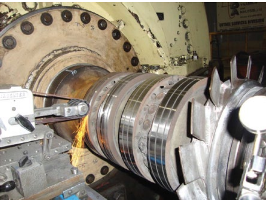
C23. Grinding operation for truing a worn, or new, collector ring
