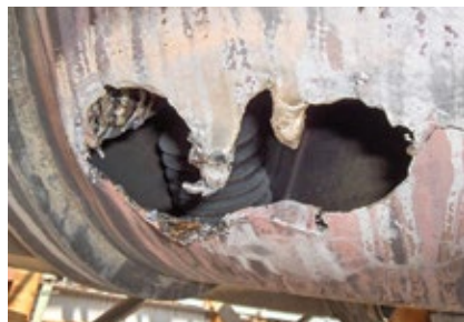
B35. Melting of the bus enclosure was caused by a line-to-ground fault
