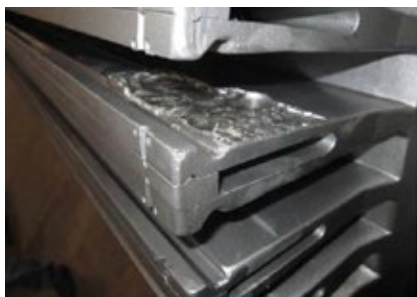
C1-C3. Negative sequence currents are a common and destructive phenomenon associated with generators. The result of these I_2 currents can be rotor body currents that can damage the rotor forging (left), retaining rings (center), and to a lesser degree, the field winding (right)
