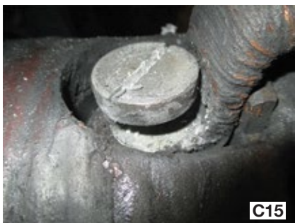
C11-C15. Typical conditions found during inspection of collector rings are threading (Fig C11), grooving (Fig C12), photographing (Fig C13), contamination (Fig C14), and heavy contamination (C15)
