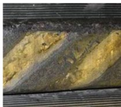
D15-D17. Failures in stator windings associated with cyclic duty include strand cracking and fracture (left), lead fracture and arc damage (center), and insulation abrasion (right)
