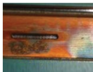
D18-D21. Impacts on rotors of cyclic duty include the failures shown in the photos above: slot-liner abrasion, insulation fracture, copper distortion, and blocked vent (left to right)
