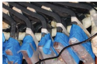
B4. Resin was injected into the dry tie material used in the rewind
