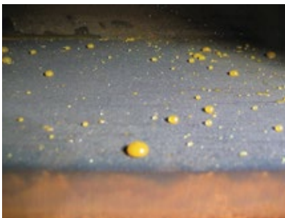
3. ODA treatment improved corrosion protection (condenser at left, last-stage turbine blades at right) during shutdown and had a positive effect on recommissioning at this steam plant
