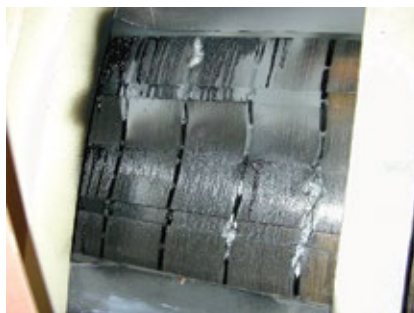
D6. Core over-fluxing in the extreme may cause total destruction of the core
