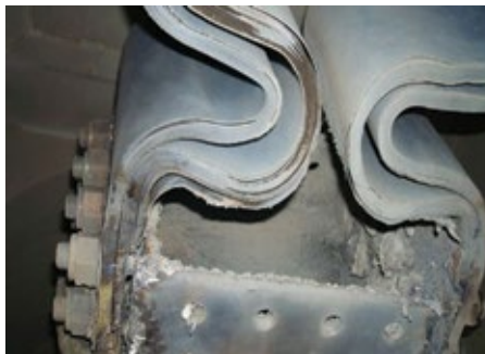
B32. Improper bolting and lack of maintenance are conducive to damaged contact surfaces at connection points
