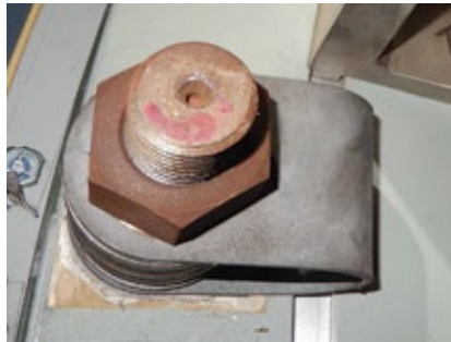
B6. Proper torqueing of keybars is critical in preventing their fracture
