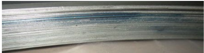
E8, E9. Rub marks are in evidence on air-side seals and shaft surfaces; plus, seals are out of round
