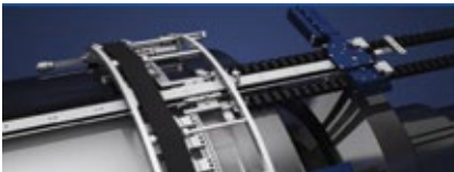
E6, E7. Retaining ring scanner at left and air-gap robot at right provide “eyes” to identify issues before they cause problems that can affect machine availability
