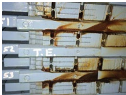
D13. Severe core and wedge looseness was found during the first major on a 7FH2 generator
