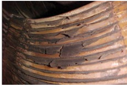
D8-D10. Rotor turn/coil shorts may not be a problem unless excessive; then they can be troublesome and destructive
