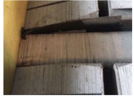
B21. Loose side packing found near the endwindings was migrating upwards into the air gap
