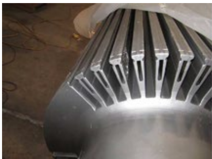
C4-C6. A double-ground fault caused severe arcing damage to the rotor, including melted material (refer back to Fig C1) and cracking on a tooth (left). The damaged portion of the tooth was removed (center) and replaced by weld build-up with appropriate heat treatment and re-machining of the tooth (right)
