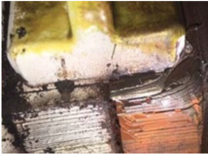
B22. Source of the foreign matter shown in Fig B20 was a very loose tooth package
