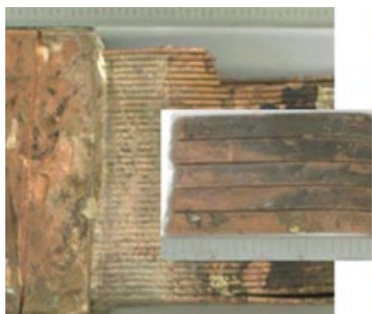
D15-D17. Failures in stator windings associated with cyclic duty include strand cracking and fracture (left), lead fracture and arc damage (center), and insulation abrasion (right)
