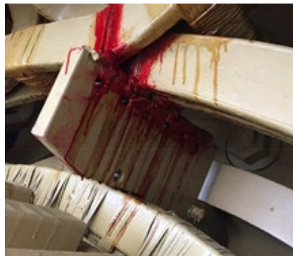
B9. Visual inspection reveals indications of two previous repairs using a weeping epoxy
