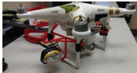
1. 3D-printed light attachment (left) and blade guard (right) are two improvements in drone technology developed by Xcel Energy's engineering team
