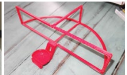
1. 3D-printed light attachment (left) and blade guard (right) are two improvements in drone technology developed by Xcel Energy's engineering team
