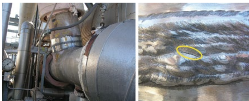
5. Crack in circumferential weld , visible at the time of discovery, became invisible to the naked eye when the pipe cooled
