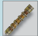
Varnish on valve spool
