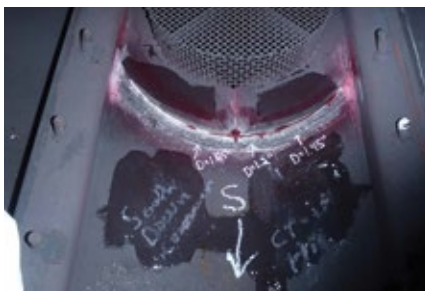
12. Stress analysis of steam-drum downcomer nozzle is at left; crack at downcomer is 1.65 in. deep in right photo
