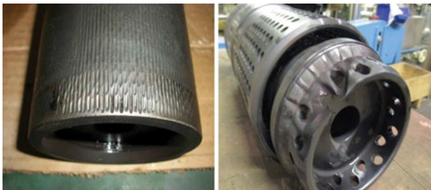
1. Erosion of HP-bypass pressure control valves is “not specific to any OEM, not a problem with most units, but a B/G problem with some,” according to one of the industry’s top HRSG consultants. At left, water and/or wet steam accessed the plug shown through perforations in the surrounding cage, creating an artistic-like erosion pattern. At right, the destructive effects of erosion are clearly visible at the bottom of the plug
