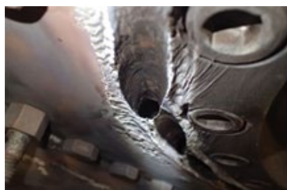
1-3. Erosion of critical steam-path parts caused by moisture and free water in steam affected the nozzle block (left), rotating blades (center), and reversing ring (right)
