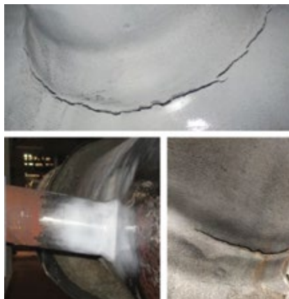
5. Excessive stresses in reheater outlet-header stubs are a direct result of cycling. Photos reveal cracked outlet branches and cracked and bent trunnions
