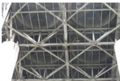
2. Air flow around the tubes usually is provided by large fans positioned below the tube bundles
