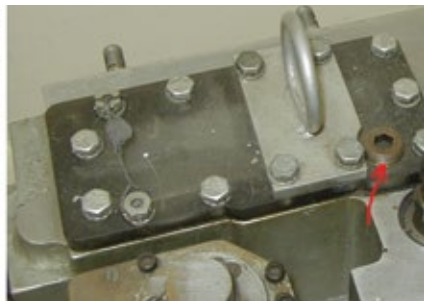
2. A typical fuel regulator by Young & Franklin is at left, the plug providing access for gag adjustment is highlighted at right
