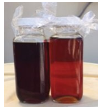
Varnish removal from GT1 oil was quick and dramatic using a portable bulk treatment conditioner. Note the color change after the first day when MPC was reduced from 50.5 to 28.3
