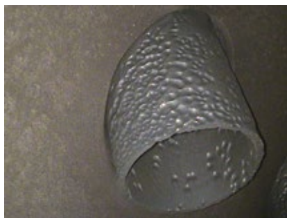
10. FAC on tube but not alloy header
