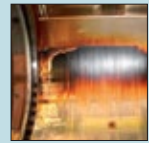
Varnish on journal bearing, gas turbine
