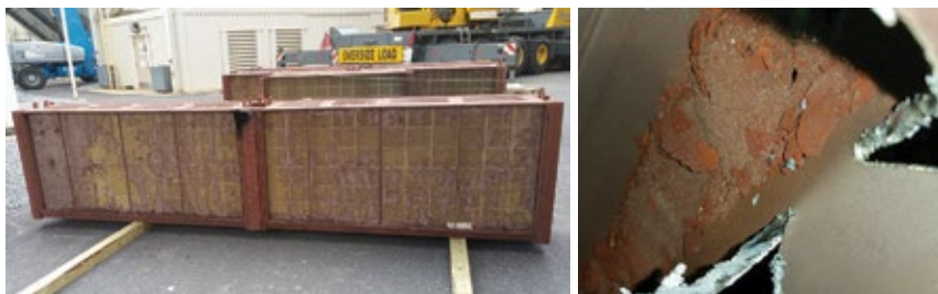
Regular inspection and maintenance can help prevent performance-robbing deterioration—such as the spent catalyst at the left and damaged ammonia injection lance at right
