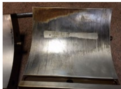
A gas-turbine journal-bearing pad exhibits a combination of wiping and varnish from frequent starts/stops and misalignment. Visit www.bearingsplus.com for a Bearing Damage Index
