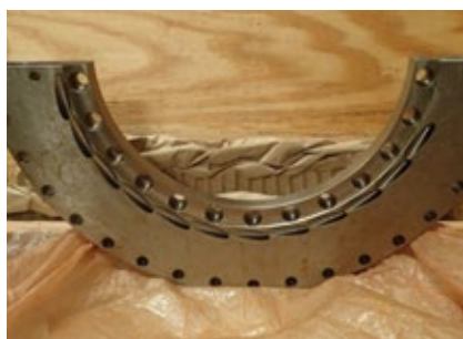
5-7. New components restored the machine to its original condition. At the left is the nozzle block, in the center the reversing-ring segment, and at right the rotating blades
