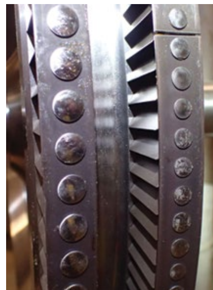
5-7. New components restored the machine to its original condition. At the left is the nozzle block, in the center the reversing-ring segment, and at right the rotating blades
