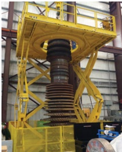
1. Rotor is prepared for a de-stack at Doosan's LaPorte (Tex) shop
