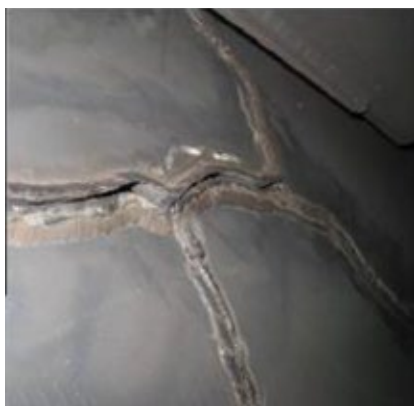
1. Crack repair attempts on exhaust cylinders are largely unsuccessful
