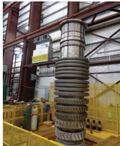
2. New air separator and torque tube are coupled to the compressor section
