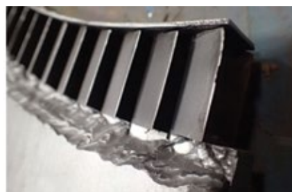
1-3. Erosion of critical steam-path parts caused by moisture and free water in steam affected the nozzle block (left), rotating blades (center), and reversing ring (right)
