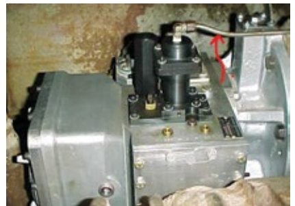
3. Air signal to the temperature bellows is increased via the tubing highlighted
