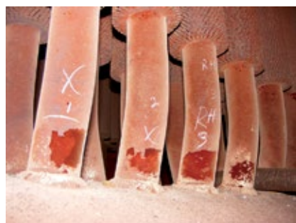
4. Exfoliation is an indicator of excessive stress
