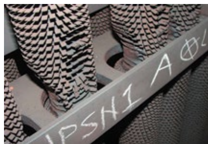
5. Fin and tube wear at tube-tie support
