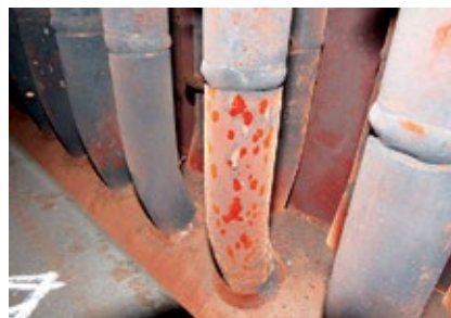
6. T22 tube should have been T91 material
