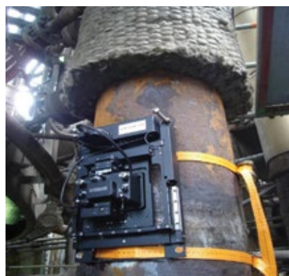
8. Portable scanning force microscope is in use on a vertical pipe
