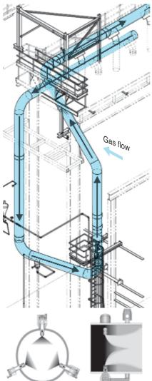
2. Redesign replaces the triple-wide spray valve design with one loop equipped with a ring-style injection nozzle without an integral valve
