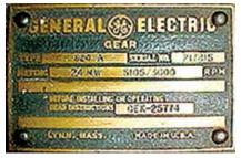
**5. Load-gear nameplate** indicates the proper GE document to access for information
