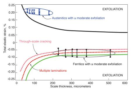
**1. Data points below the green line** in this graph (famous with OGE specialists) indicate a higher risk of exfoliation from ferritic steels typically used in the manufacture of superheater and reheater tubes. The original oxide failure map was developed by Armitt and others in 1978; Dooley and Patterson added exfoliation data in 2003
