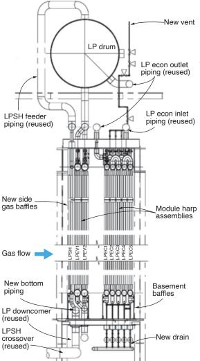
**3. New T11/P11 LP evaporator** and economizer modules are designed to handle cycling, and for ease of draining, venting, access, cleaning, and installation
