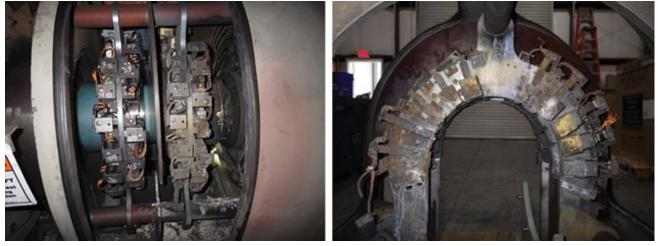
6. The outboard collector ring (at right in left photo) and associated brush-rigging components suffered severe arc damage. The outboard collector ring as viewed from the brush rigging is in the right-hand photo
