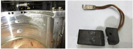
**5. Bearing electrolysis damage** and a broken shaft grounding brush were revealed during an inspection to determine the cause of high vibration
