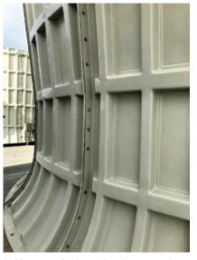
**2. New stacks** have hardware on the outside, making for easy maintenance access
