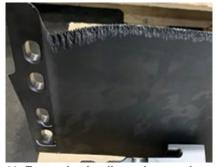
**11. Excessive leading-edge erosion** often is identified with 40-in. L-0 titanium blades installed in many steam turbines
