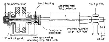
**3. Quill drop check** is a critical measurement in the alignment process. Note that "Y" on the generator coupling lines up with "Z" on the load-gear coupling
