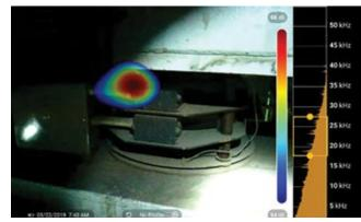
2. Small hydrogen leak from a generator bushing is identified here
