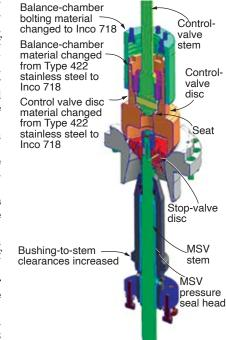
8. GE's digital valve upgrade was implemented to reduce stem erosion
