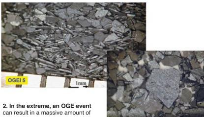
can result in a massive amount of material downstream, as this photo of a P91 superheater header shows
