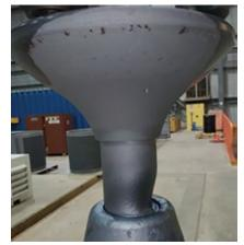
7. Main-stop-valve stem wear, attributed to solid-particle erosion, occurred over run of seven and a half years
