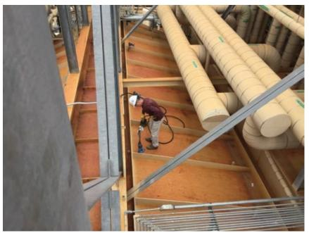
**3.** In the top-traverse test method, a weighted probe is lowed to desired locations in the inlet and outlet flow planes to measure  $NO_x$  and  $NH_3$ ; Gretta says it usually takes only three to four hours for adequate sampling in each plane
