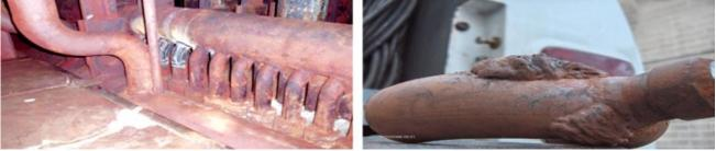
4. Six different weld-repair styles kicked off Bremco's tube-repair clinic, after the audience gasped at photos of the ugly, uglier (left), and ugliest (right) welds in service
