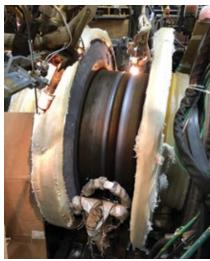
A 360-deg, deep rotor crack was excavated and weld-repaired allowing a return to service
