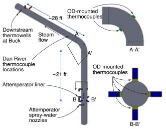
6. Attemperator effectiveness was analyzed using these arrangements of thermocouples mounted on the outer diameters of the 24-in. OD, Sch 80, Grade 22 reheater piping at Duke Energy's Buck and Dan River plants. T/c data have been collected in the DCS system since May 2018
