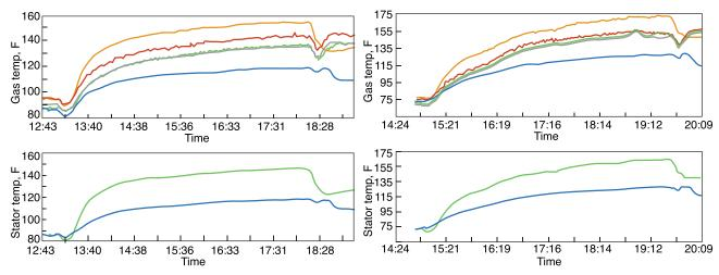
**Tests using hydrogen coolant** (left-hand charts) in August 2017 showed a maximum gas temperature of less than 155F and a maximum stator temperature of less than 150F. Temperatures using helium coolant in April 2018 tests (right-hand charts) were slightly higher with gas temperatures remaining below 175F and the maximum stator temperature also less than 175F
