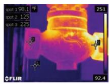
5. Thermal scans are valuable for identifying where performance-robbing leakage is occurring
