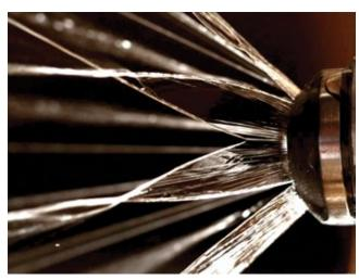
**5. Spray pattern** of a mechanically atomized fixed-orifice spray nozzle can be disrupted by inadequate water pressure, clogging, damage to the sharp edges required to produce droplets of uniform size, etc. Photo shows what happens when a springloaded nozzle operates below the minimum pressure required
