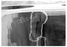
2. Cracks of significant length and depth at this turbine's HP inlet were ground out and weld-repaired
