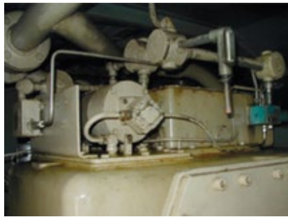
1. Hydraulic ratchet assembly sits on top of the Frame 5L's accessory gearbox
