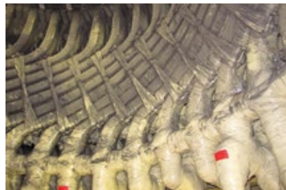
4. What remains of a failed connection is at the left, melted copper from this failure is in the center, resulting contamination to the stator winding is at the right
