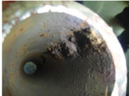
3. Inappropriate cycle chemistry caused waterwall and superheater-tube failures
