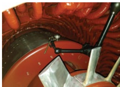
2. Radial runouts on retaining rings were checked following unit trip on high vibration
