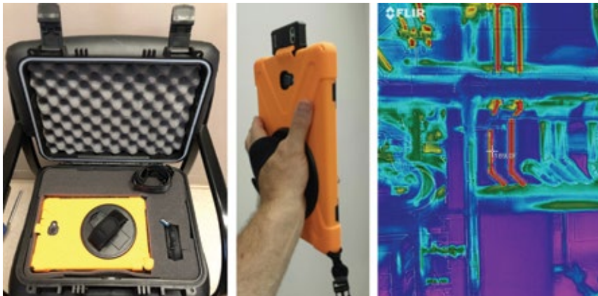
Thermal imaging camera tablet, tablet case, and protective storage box are shown in the left and center photos with an example of an image provided by the camera at the right
