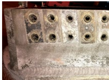
2. Arcing damage to flexible-lead contact surface is shown at left, to bus-connection surface at right
