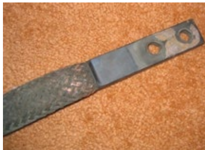
2. Arcing damage to flexible-lead contact surface is shown at left, to bus-connection surface at right
