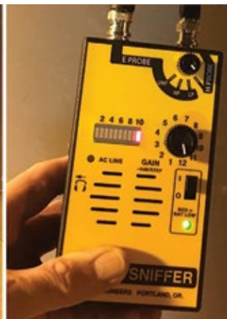
5. Instrument for locating partial discharge and EMI
