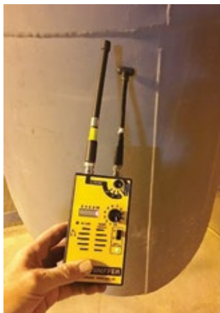
5. Instrument for locating partial discharge and EMI
