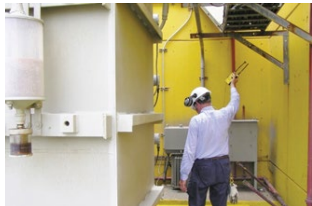
6. Plant is surveyed for electromagnetic radiation using Model 246A instrument from Radar Engineers
