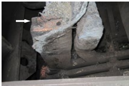
4. What remains of a failed connection is at the left, melted copper from this failure is in the center, resulting contamination to the stator winding is at the right
