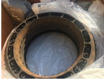
1. Combustor replaced during Spring 2018 overhaul
