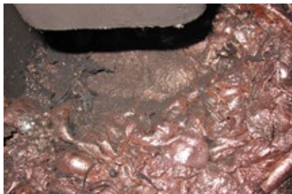
4. What remains of a failed connection is at the left, melted copper from this failure is in the center, resulting contamination to the stator winding is at the right
