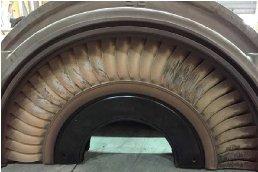
4. Steam turbine experienced deposits, pitting, and cracking
