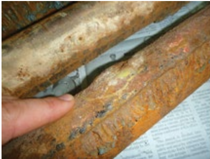
3. Inappropriate cycle chemistry caused waterwall and superheater-tube failures
