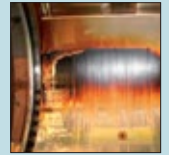
Varnish on journal bearing, gas turbine
