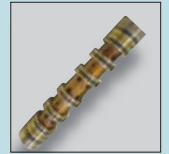
Varnish on valve spool
