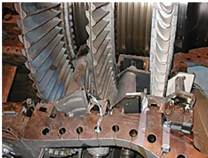
3. Turbine section of a Frame 6 illustrates three-stage arrangement (left). Arrow in photo of first stage at right points to where firing temperature is calculated (not measured)
