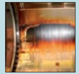
Varnish on journal bearing, gas turbine
