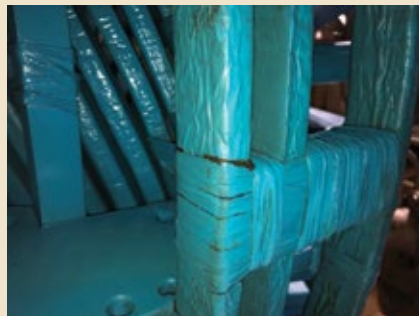
1, 2. Inspections in the early 2000s found problems primarily on the stators—such as connection-ring vibration (left) and stator bar vibration (right)
