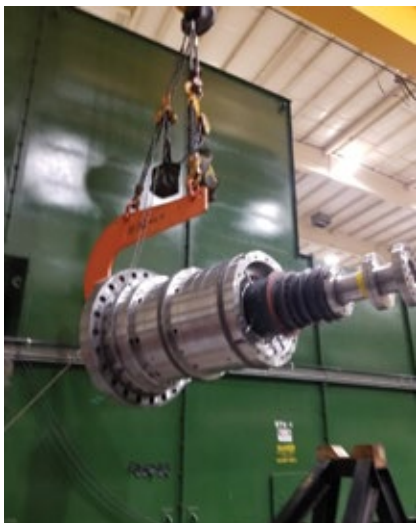
5, 6. New HP steam turbine rotor and barrel assembly is at left, new LP section at right
