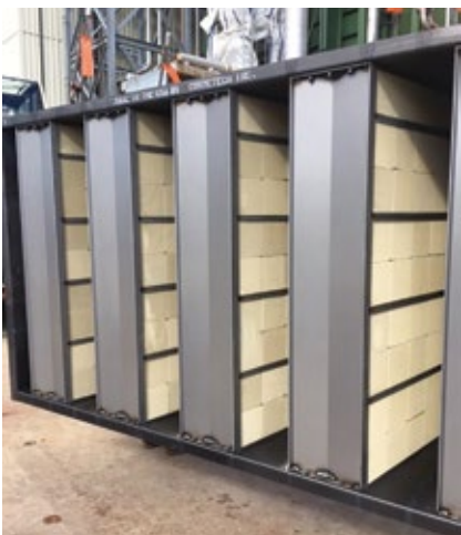
4. New catalyst controls emissions of multiple pollutants simultaneously
