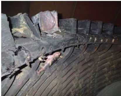
6-8. Inspection results: Field pole crossover cracking (left), phase-to-phase failure (center), bottom-bar insulation damage
