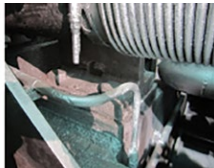
9-2. Vertical bolting and dowel hold the support leg in place
