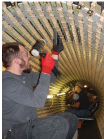
7, 8. Piggyback wedge system for medium- to large-size machines being installed (left) has a history of proven performance and often is used as an upgrade solution (right)
