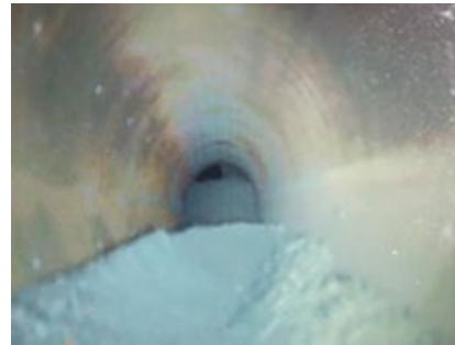
10. Debris buildup inside duct-burner elements can be evaluated using a borescope
