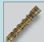
Varnish on valve spool
