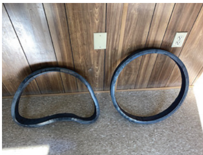
2. Strange things can happen to equipment in severe service. Welds joining the valve seats to their bodies were found broken and one of the seats badly deformed
