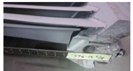
8. A thermal mismatch across the upper and lower halves of a diaphragm can create bending forces strong enough to crack (left) and liberate (right) nozzles
