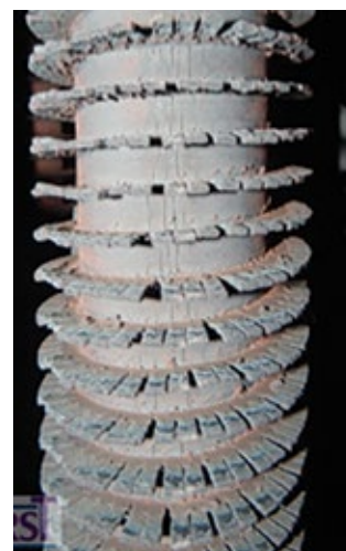
2. Reheater tube reveals long-term overheating damage
