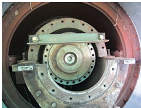
9-9. Rotor locking plate prevents axial shift
