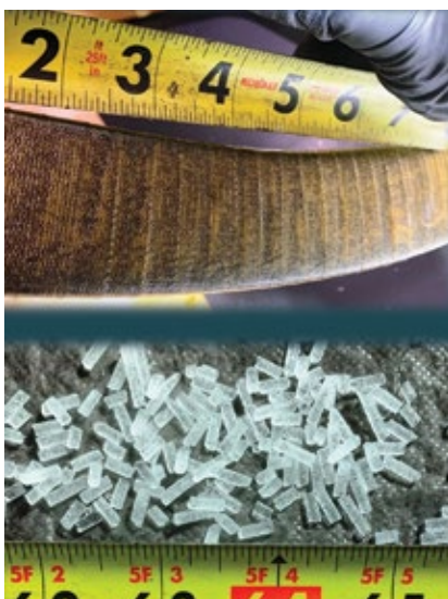
3. Electric Machinery's rice-like CO 2 pellets (bottom) were effective in cleaning insulation (top). Tight process control is necessary to prevent unintended damage to insulation
