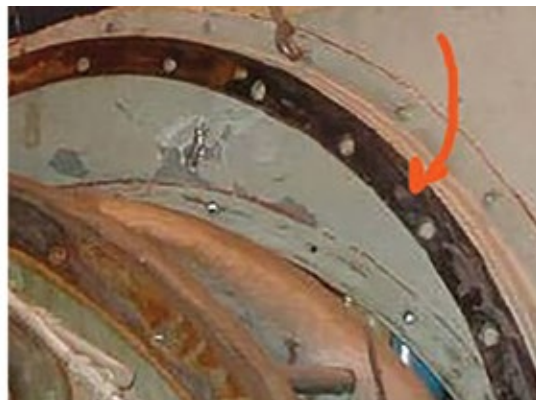
9-5. Bolts around the engine circumference hold exhaust seals in place
