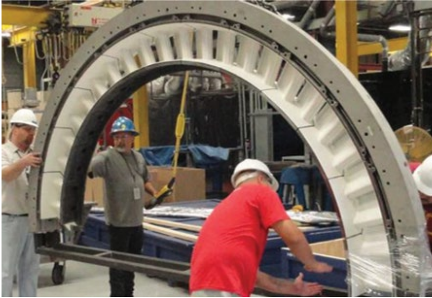
5, 6. MD&A's TBC coat for F-class first-stage nozzles (left) is said to offer superior oxidation resistance. Repairs to F-class second-stage blades make these parts better than when they were new (right)
