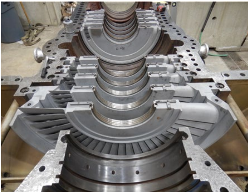
1. Upper-half casing of an impulse steam turbine, flipped over, shows the top halves of diaphragms fully assembled in their proper locations
