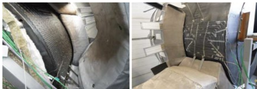
7. ARNOLD Group believes the "heater on metal-mesh baffle" (left) is the optimal configuration for turbine upper casings, offering easy removal, good contact; "heater on surface body" for lower casings (right), provides good contact and heat transfer
