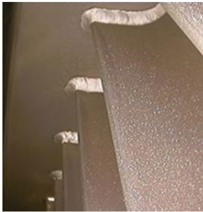
5. Full-perimeter fillet weld tie each blade into the inner and outer rings
