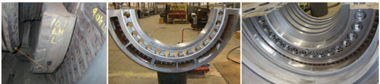
3, 4. Steampath failures , such as the diaphragm at left, typically require re-engineering and parts of new manufacture, as illustrated by the upper-half nozzle plate before (center) and after (right) installation
