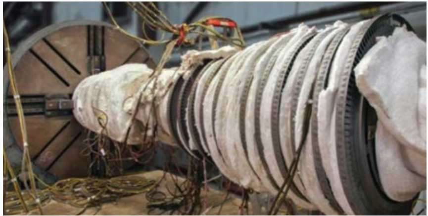
2. One rotor-straightening option includes thermal stress relief to relax internal residual stresses
