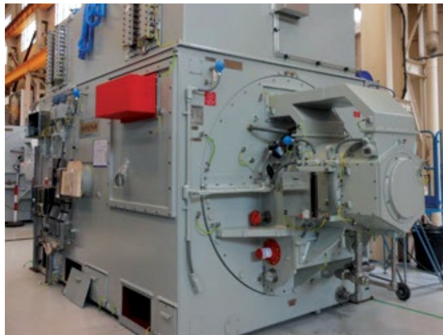
2. Brush 2-pole, 13.8-kV generator is designed for operation in hazardous areas
