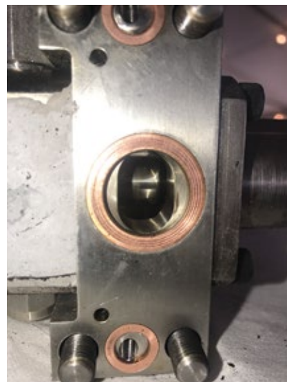
5. Copper crush gaskets provide more reliable long-term sealing than Viton O-rings in high-temperature applications. Photo shows these gaskets in a water-cooled three-way check valve that bolts to the fuel-nozzle distribution valve by way of an intermediate flange. Because check valves sometimes must be removed to facilitate maintenance, use of the multiple-use copper crush gasket speeds reinstallation, thereby enabling a quick return to service
