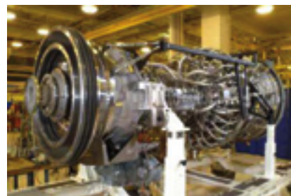
3, 4. LMS100 combines proven components from the OEM's aero and frame product lines. Photo is of the engine's supercore
