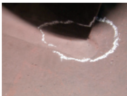
8. LP baffle reveals protective oxide coating and no signs of FAC or oxygen pitting
