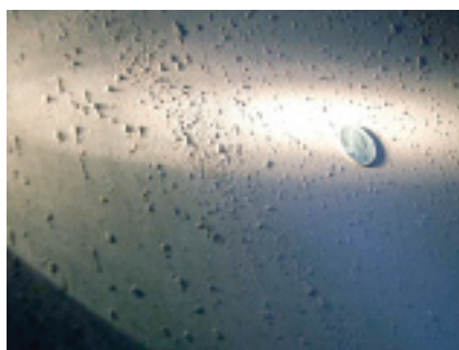
6. Oxygen pitting in HP steam drum found during inspection in 2005
