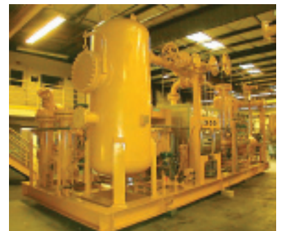
Screw fuel gas boosting compressor used with aeroderivative gas turbine (output: 50 MW)
