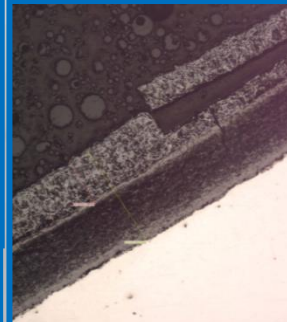
Steamside spalling and implications for downstream components.
