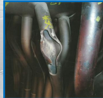
Detrimental impact of transient thermal excursions on component integrity.
