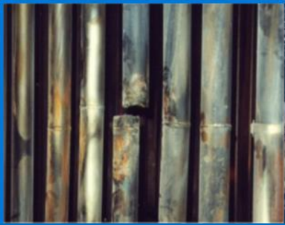
Rogue PWHT leading to SCC failure within 48 hours.
