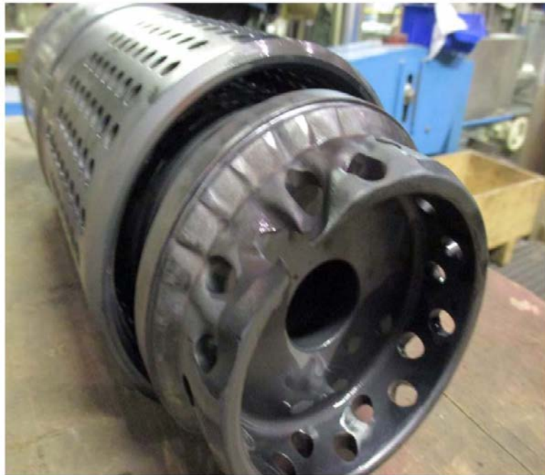
Figure 14 – Abnormal PCV plug and cage wear after only a few start/stops
