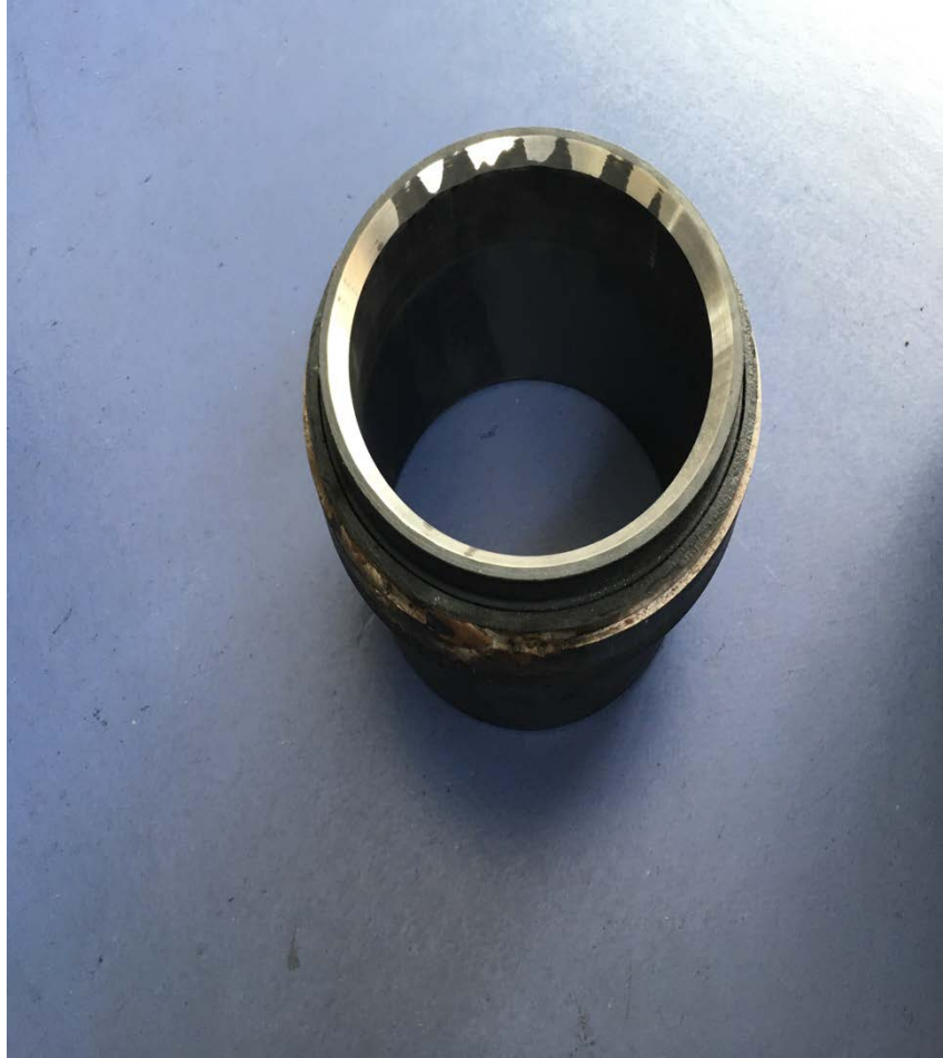
Figure 13 – Normal PCV seat wear after 5 years of cycling service
