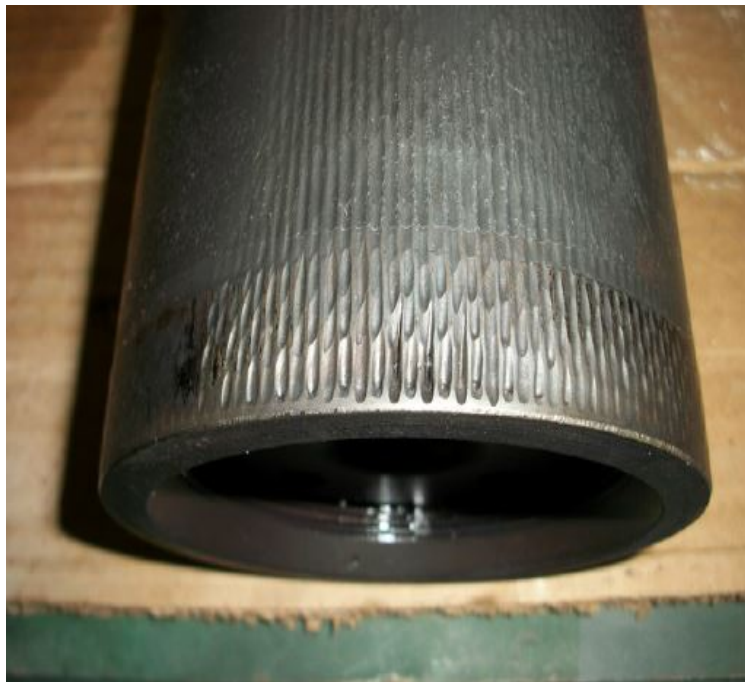
Figure 15 – Abnormal PCV plug and cage wear after about one year of service
