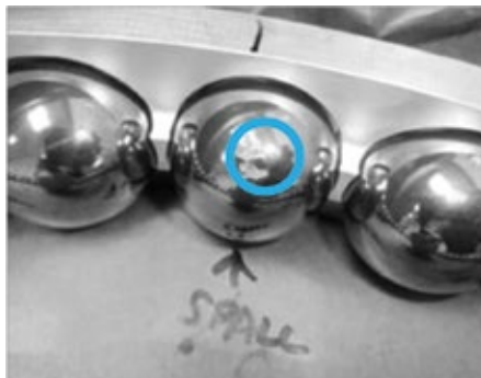
GasTOPS. Bearings and gears are damaged in service because of stress concentrations that arise from misalignment, mishandling, misassembly, corrosion, and contaminants in lube oil
