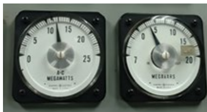
4. Power output (left) and reactive power output (right) for the Frame 5L described in the article
