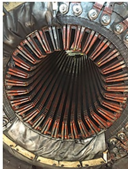
1. Dry-ice cleaning of a generator core (before at left; after at right) facilitates inspection and repairs
