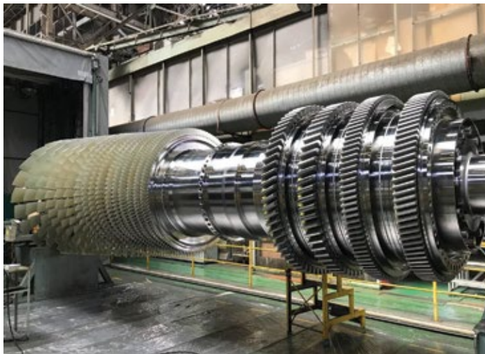
Mitsubishi Power's first new-manufactured, upgraded W501F rotor is at left, details on the thick torque tube and bolted air separator to correct long-standing issues with the original design are shown at right
