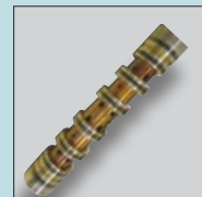
Varnish on valve spool
