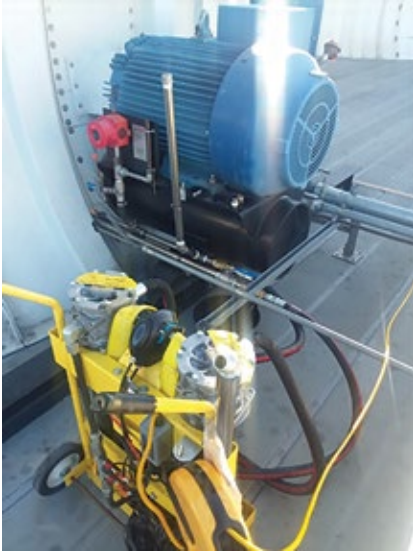
3. Filtration cart is small enough for one technician to perform the tasks required
