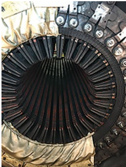
1. Dry-ice cleaning of a generator core (before at left; after at right) facilitates inspection and repairs
