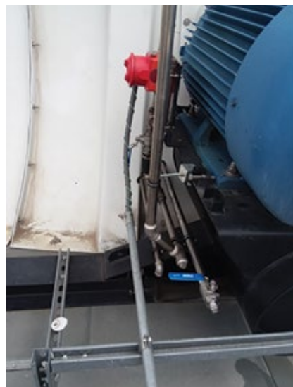
2. Service lines terminate outside the shroud, facilitating hook-up to the filtration cart
