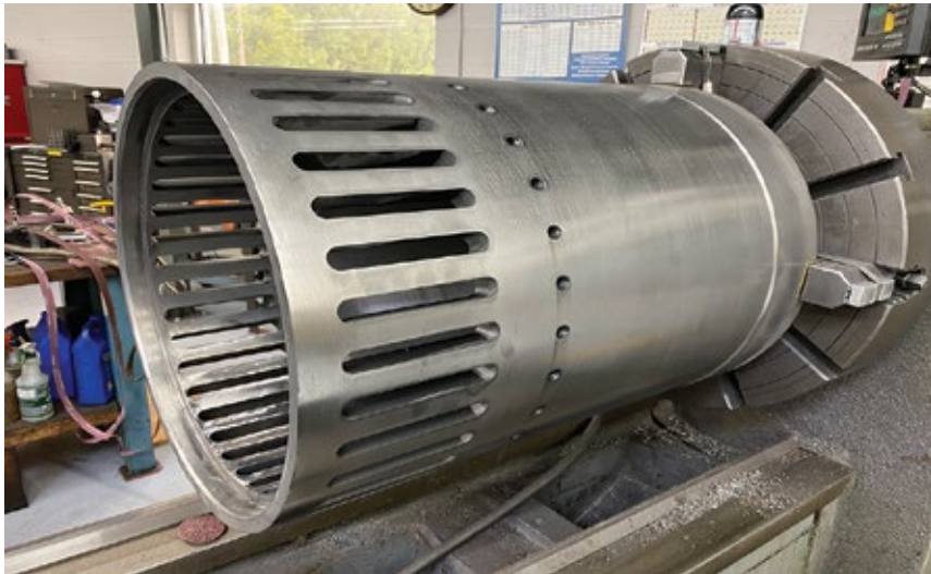
3. Final machining of a large valve cage is done by lathe
