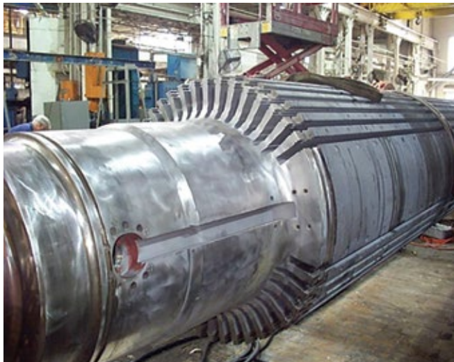
National Electric Coil. Rotor forging was machined from a single piece of NiCrMoV steel to withstand torsional, lateral bending, vibratory, and rotational stresses
