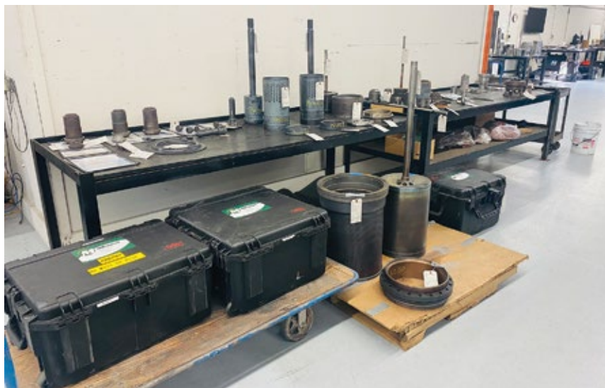
2. Outage complete , trim kits and reusable parts are returned to the Millennium shop for restocking and repair
