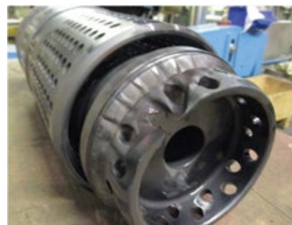
4. Typical HP pressure-control-valve erosion
