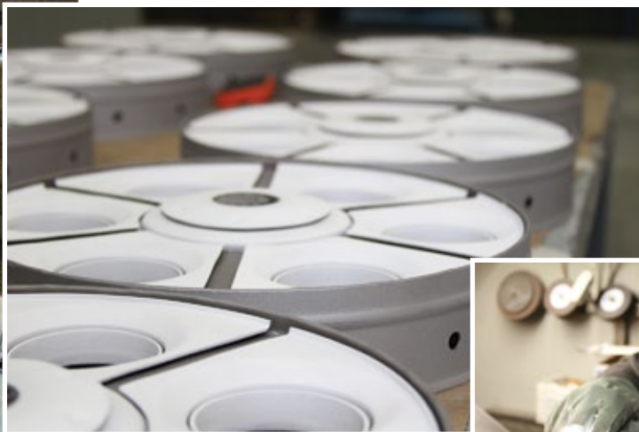
2. Re-coated combustion covers
