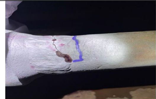
WELD 6 INITIAL PT LINEAR INDICATION NOTED
