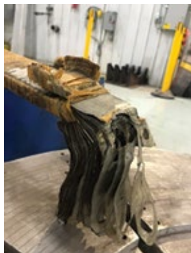
2. Three examples of main-lead J-strap overheating and arcing, an electrical failure
