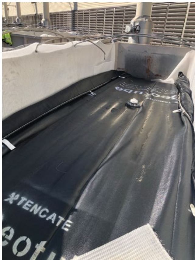
1, 2. Semi-solid waste material is pumped from the chlorine contact chamber (left) to geotubes (right) by an engine-driven pump
