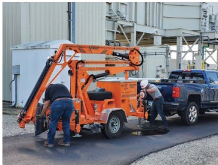
3, 4. Mobile tie-off system in travel mode at left, ready for work at right.
