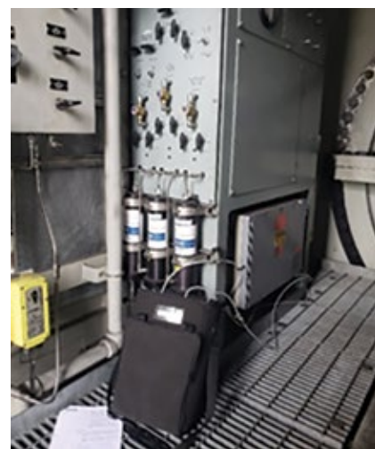
4. Portable calibration-gas kit in service illustrates the ease of use
