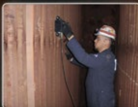
OD Scanning for Tube Wall Thickness
