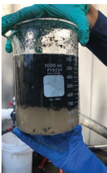
4, 5. About 4 ft of semi-solid waste material was removed from the chlorine contact chamber to maintain proper system performance (left). Flocculant testing of the semi-liquid waste material is at right
