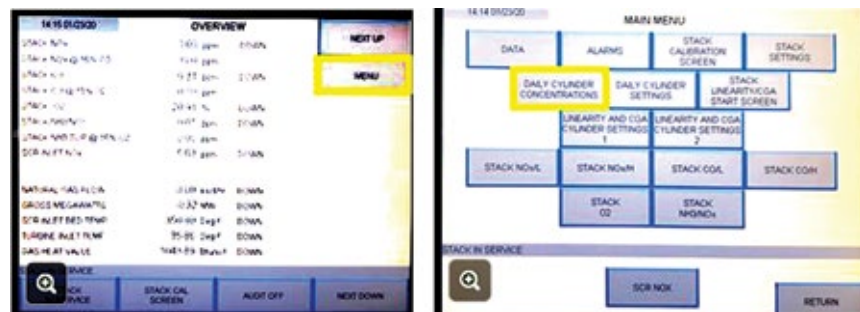
3. CEMS panel on the operator interface terminal. On the overview screen at left, tapping “main menu” button brings up the screen at the right. Tapping its “daily cylinder concentration” provides guidance on when cylinder replacement is necessary
