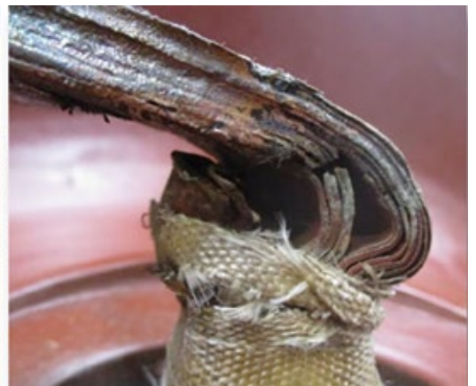
1. Main lead rotational and radial failure manifests as compressed and twisted leaf copper (left) and broken leaf copper (right)
