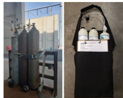
3. Original arrangement of calibration-gas cylinders is at left, new portable kit at right
