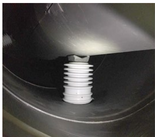
10. Insulator tracking was found in Phase A of the steam turbine/generator
