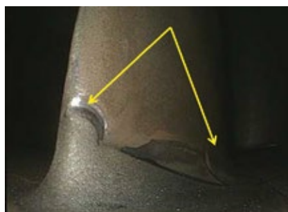
5. Stator was damaged by liberated shim
