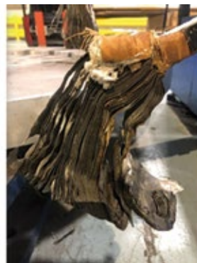
2. Three examples of main-lead J-strap overheating and arcing, an electrical failure
