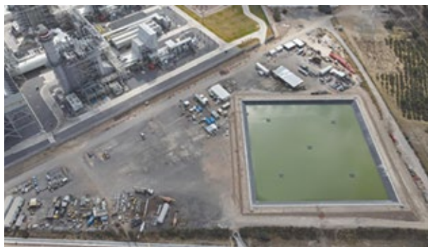
1. New pond under construction is at left. One mechanical evaporator was installed in each of the 200-ft-diam pond sections outlined above
