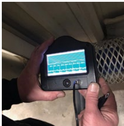
1. Technician checks steam trap for proper operation at left, views results above
