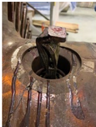
1. Main lead rotational and radial failure manifests as compressed and twisted leaf copper (left) and broken leaf copper (right)
