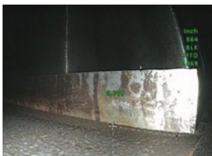
4. Failure of retention hook allows shim to protrude from the compressor
