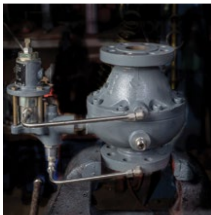
1, 2. Pilot-operated, high-pressure regulator, Type 310A, is used where high capacity and accurate control are essential. Pilot assembly (Type 32A) is for pressure-reducing or wide-open monitoring applications
