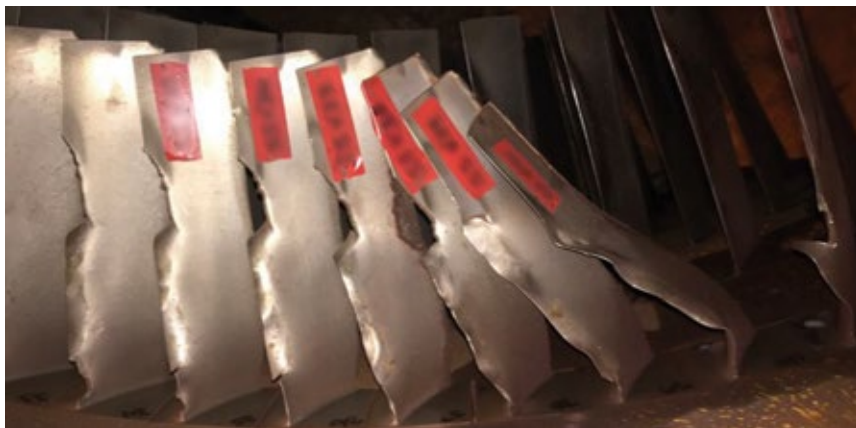
3. Significant damage was found in Row 5 of the 7F compressor; vane damage is shown here
