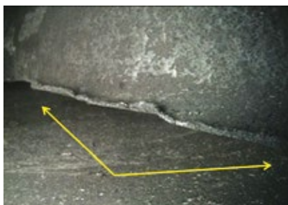
1. Rotor-blade tip distress is most commonly caused by contact with the case during operation
