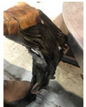
2. Three examples of main-lead J-strap overheating and arcing, an electrical failure
