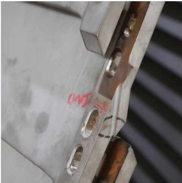
1. A- \frac{3}{8} -in. crack was found on the tip of an L-0 blade in the LP
