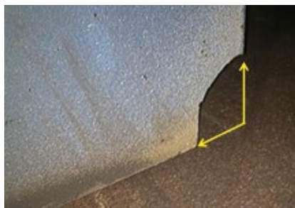
2. Eddy-current inspection detect radial tip cracking shown prior to tip liberation
