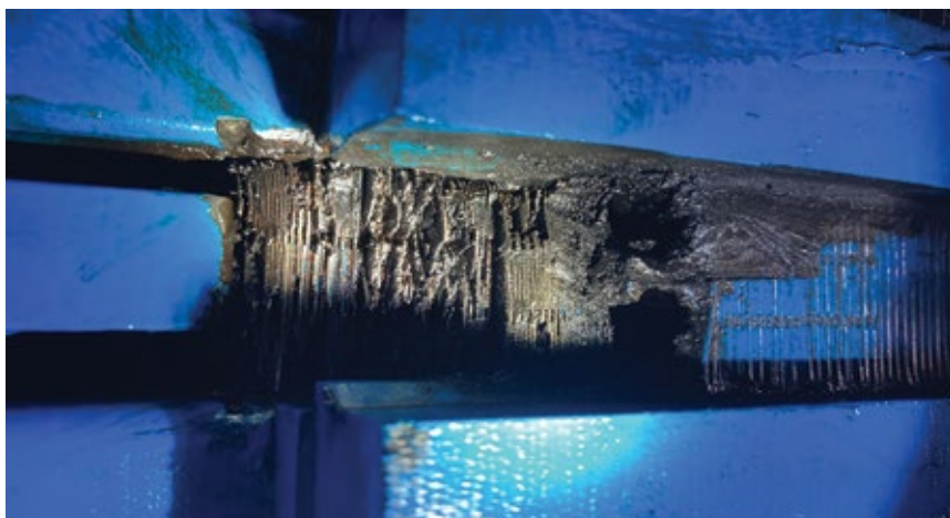
4. Damage to core iron was significant
