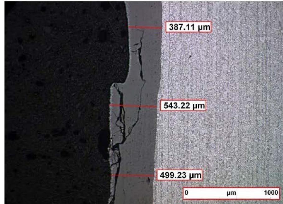
Oxides Much Thicker Than Near Failure Zone
