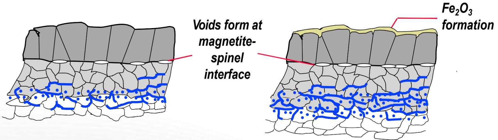
3. As oxidation rate slows, Cr-rich oxide precipitates start to form semi-continuous layers along alloy grain boundaries
