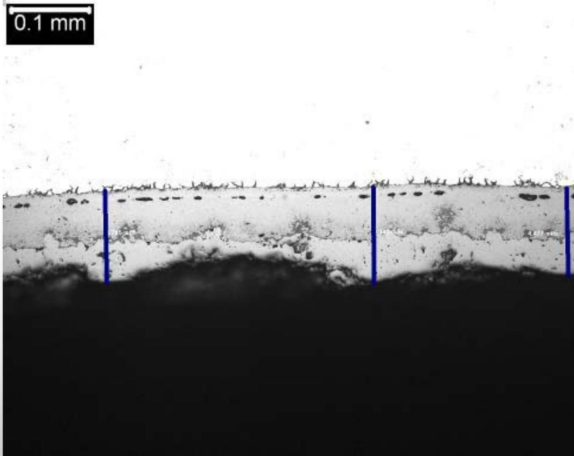
But at some stage it starts to form a new duplex pair (laminated) at the tube/oxide interface
