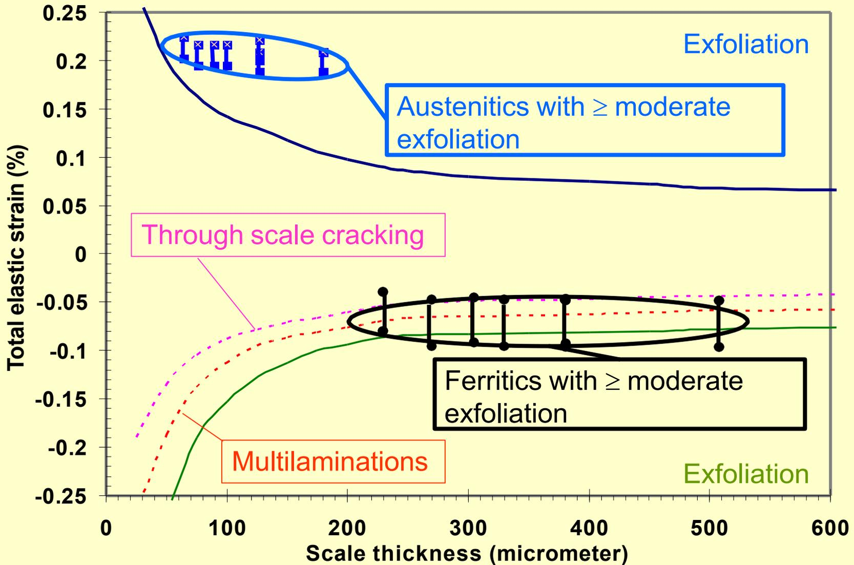
Original Oxide Failure Map: Armitt et al 1978
