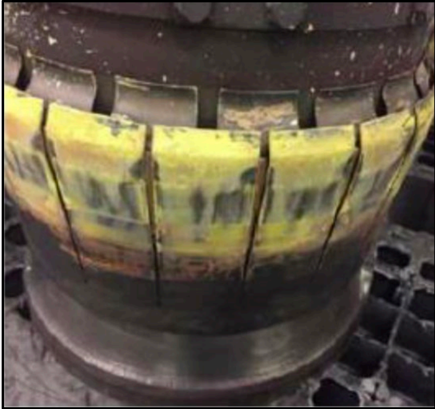
GT Combustor Basket Spring Clips
