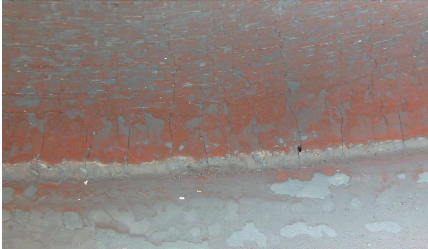
Root of downstream steam pipe weld from the inside bottom
