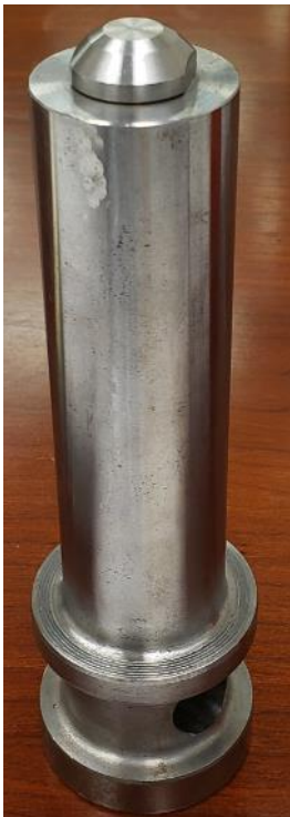
Original nozzle and sleeve to be replaced
