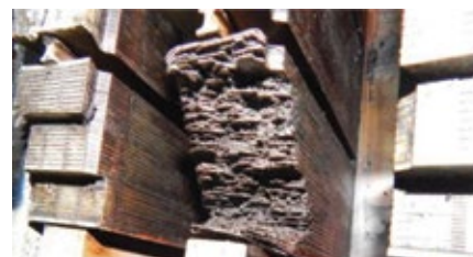
7. Core looseness can lead to outside space block (OSSB) migration on large generators (left). Tooth loss on 7FH2 generators (right) most often is associated with units made by Mitsubishi Power
