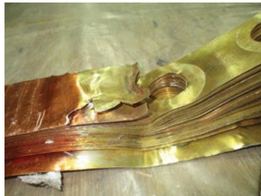
6. Main-lead mechanical and electrical failures included broken J-strap leaves at left and J-strap overheating/arcing at right
