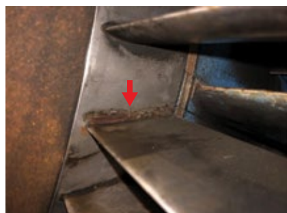
2. Inlet guide vanes , pressure side shown, were liberated from the tip shroud (arrow)
