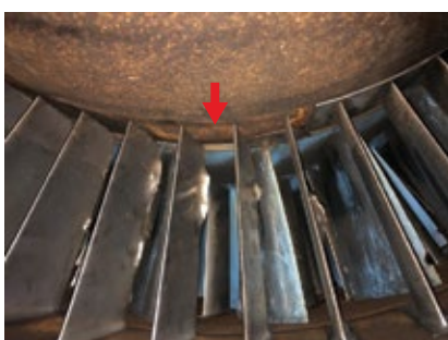
3. A section of the inner shroud is missing (arrow). Note the impact damage to the trailing edges of the inlet guide vanes (suction side)
