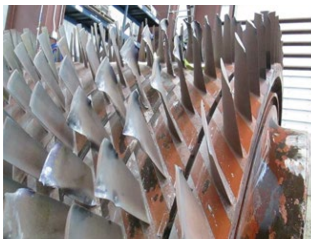
2. Compressor damage as-found is at left. Repaired, stacked, stretched compressor rotor is married to the repaired turbine rotor at right. A unit rotor balance was done before progressive blade/balancing of the turbine section
