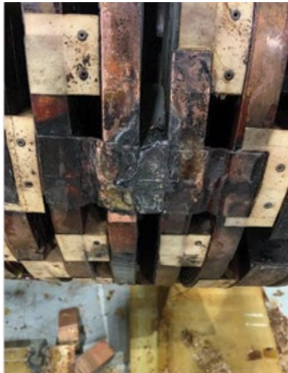
10. Nomex tab rivet failures were in evidence after retaining rings were removed to inspect endwindings. Photo shows jumper condition with melted blocking
