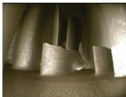
4. Two S0 vanes liberated at the 6 o'clock position
