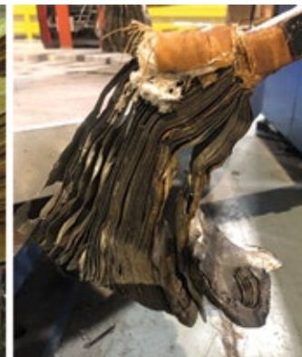
6. Main-lead mechanical and electrical failures included broken J-strap leaves at left and J-strap overheating/arcing at right
