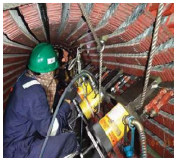
12. Repairs are made in photo at left to correct a stator failure (T6 neutral phase ring at flex leads). Rewind complete, the phase ring is prepared for bump testing at right
