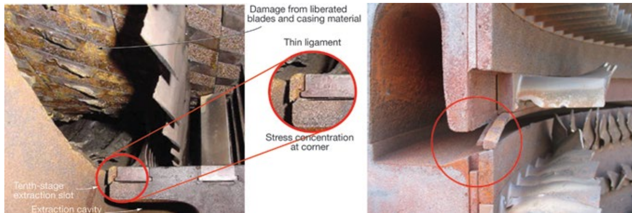
1. The thin ligament at the 10th-stage extraction slot may be weakest point in the Frame 5 compressor (left). It is susceptible to cracking, which can cause major damage if it occurs. Photo at right shows how: The hook portion of the casing simply “peels” away, allowing vanes to work free and go downstream
