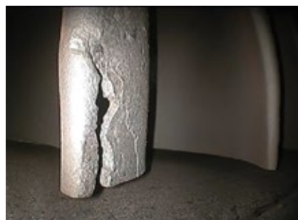
7. Impact damage and material loss was found on several first-stage buckets in the turbine section
