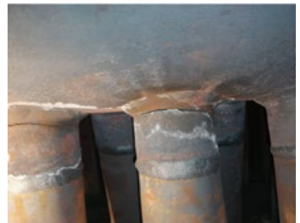
6. P91 reheater failure was caused by cycling-induced thermal-mechanical fatigue and condensate quenching
