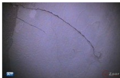
3. HP attemperator liner cracks are in evidence from borescope inspection
