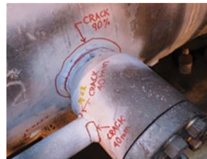
3. Cracks in the HRH bypass dump arrangement were discovered at the nozzle housing (upper area) and at the water manifold (lower area)
