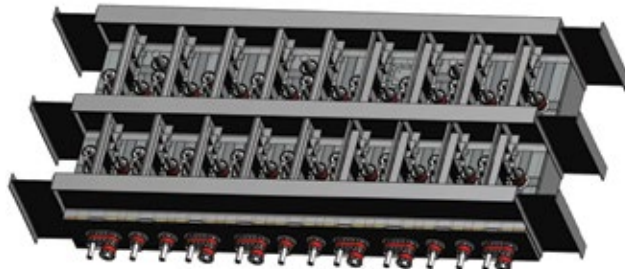
11. Complete roof module features upgraded cold casing and penetration seals
