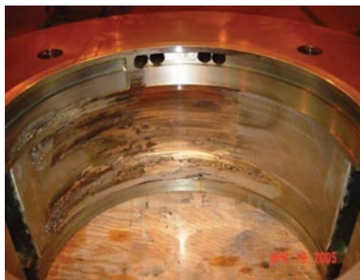
9. Unintended magnetism can cause problems such as eddy current damage to bearing journal at left and housing damage to turbine bearing at right
