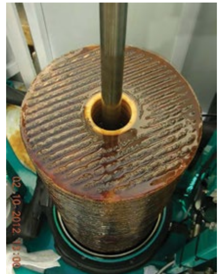
2. Filter disks are effective in removing varnish
