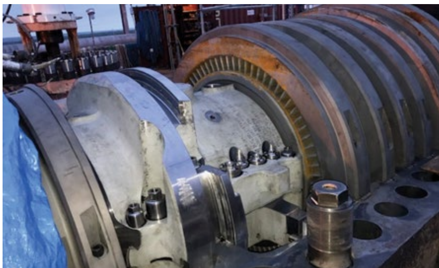
2. Upgraded N2 packing can help maximize the value and extend the life of your steam turbine
