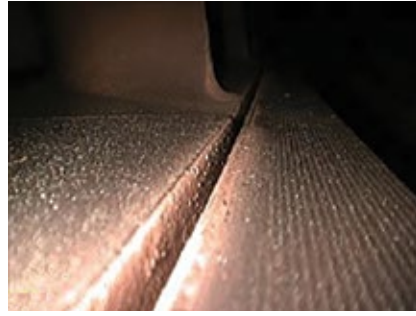
9. Stator-vane hook-fit separation in the ninth stage ranged from 32 to 68 mils between the case material and vanes
