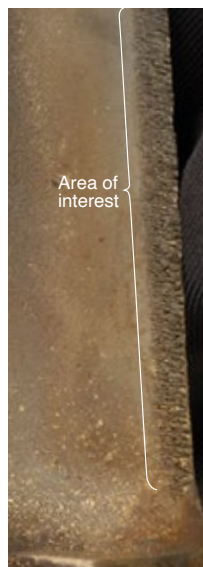
1. Trailing edge erosion, associated with moisture-droplet impacts on some L-0 blades, can lead to crack initiation and possibly airfoil liberation
