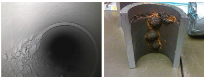
2. Cleaning to remove corrosion cells (right) is more involved than a cleaning to remove high levels of iron-only UDC (left)
