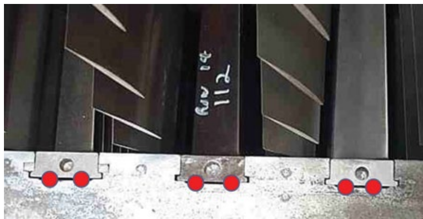
1. Loose ring segments in compressor stages S17, EGV1, and EGV2 are secured as shown using spring pin dampeners
