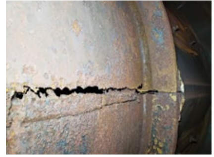
10. Corrosion and material loss in the exhaust section was significant
