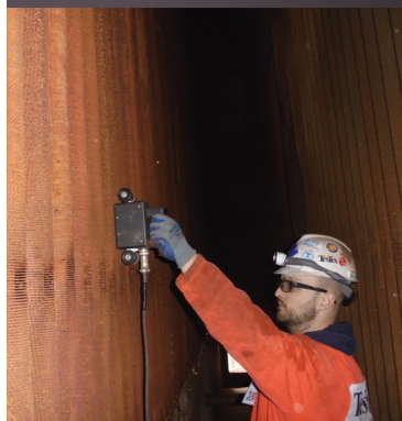
Through Fin Tube Scanning for Wall Thinning
