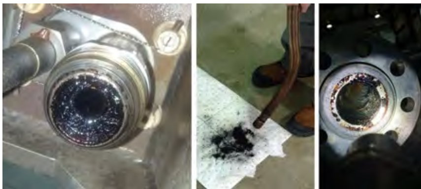
1. Coking in fuel nozzles, gas supply header, and hoses impeded transferring back to gas fuel after operating on distillate oil
