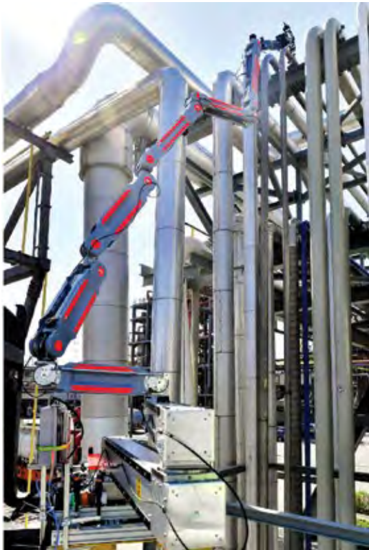
8. Float-arm application example: Here the arm is passing through narrow gaps between pipes to reach challenging locations
