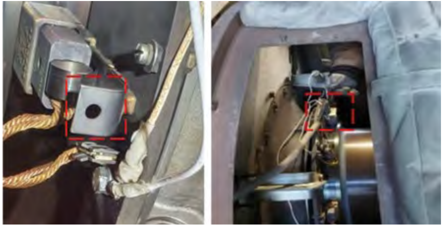
3. Brush-holder lock is of the spring type (left); strong air currents are caused by the moving rotor (right)
