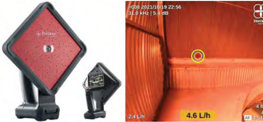
5. The Distran Ultra Pro (left) makes image-based results available for air leakage detection (right)
