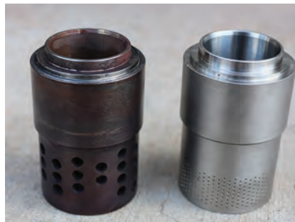
1. Original control-valve trim is at left, IMI CCI's retrofit trim is at right
