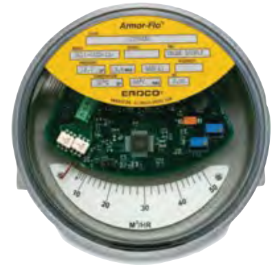
6. ERDCO's Armor-Flo device links to the plant DCS
