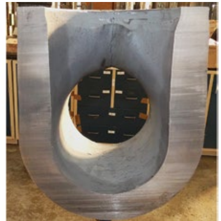
6. Tee suffered a through-wall crack at the crotch position on one side and another partially through-wall crack on the other
