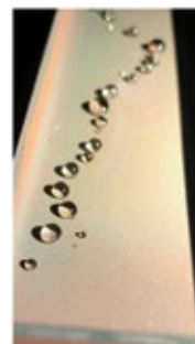
1. Background on FFA chemical structure. Hydrophobic film has been thought to "protect" the steel by decreasing contact between water and metal
