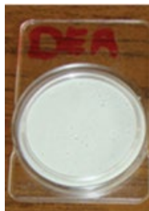
4. Snow-white Millipore filter confirms optimized corrosion rate
