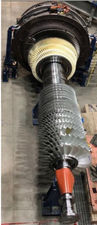
Hybrid rotor increases the shaft limit for the 501F to 227 MW
