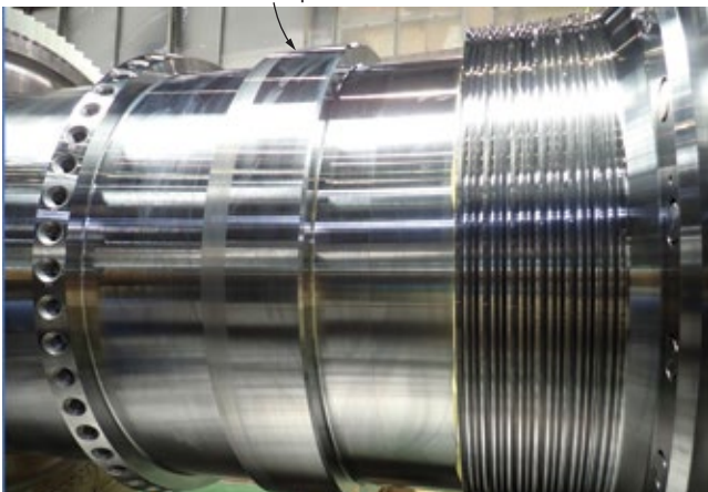
Mitsubishi Power's upgraded 501F rotor features a thick torque tube as a reliability improvement
