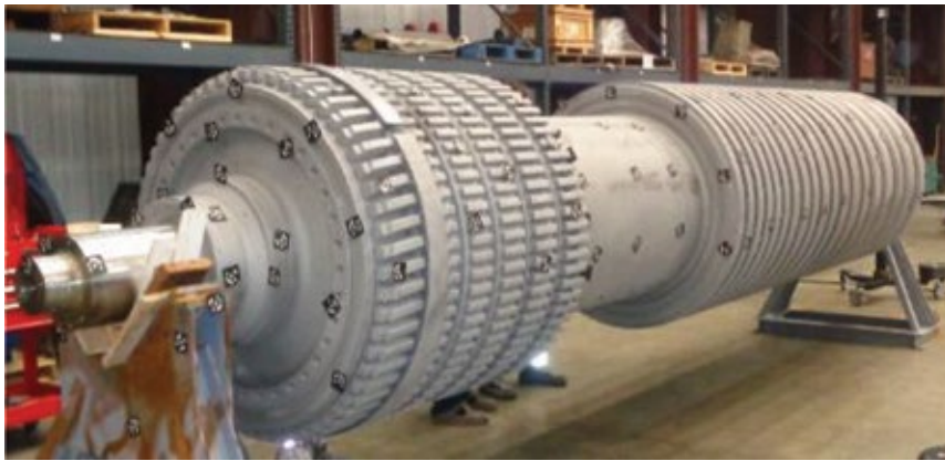
15. Doosan Turbomachinery Services’ reverse engineering involves internal and external characterization and metallurgical evaluation
