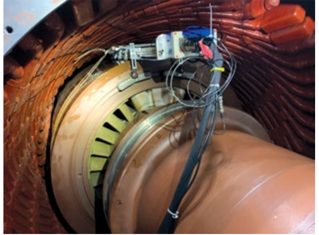
Generator retaining rings should undergo nondestructive examination at least once a decade, according to the OEM
