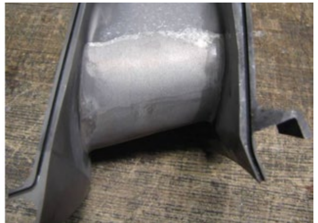
10. Impact damage to nozzle guide vane is heavy on leading edge; some trailing-edge damage as well. Otherwise, however, part is in good shape with low hours (left). At right, repair success using Liburdi Powdered Metallurgy: Part was returned to service for a 24,000-hr interval. Post service inspection found no indications or material loss
