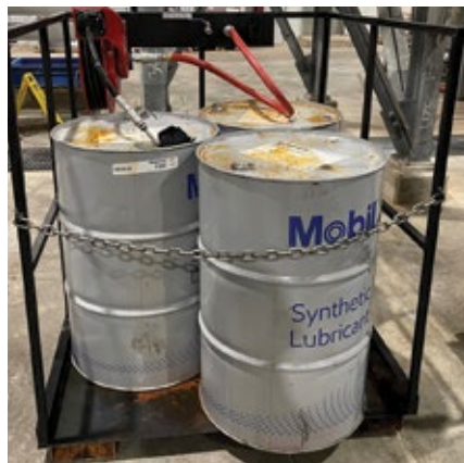
1. Identical totes are used for handling DTE (left) and SHC (right) oils separately
