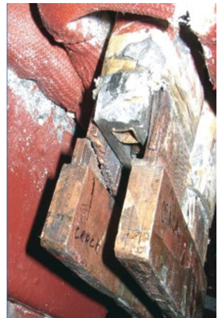
16. Stator and field are impacted by mechanical and thermal forces. Broken strands are one possible result
