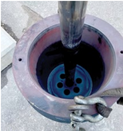
3. Plug and cage are stuck in position
