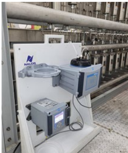
5. Iron concentration is measured with an online laser nephelometer
