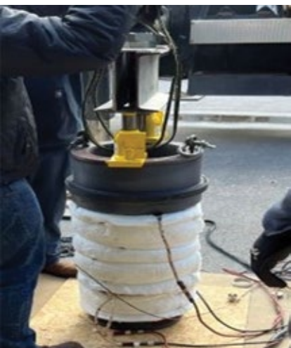
4. Separator rig relies on heat and jacks to separate the parts
