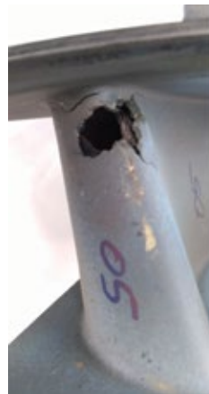
10. Impact damage to nozzle guide vane is heavy on leading edge; some trailing-edge damage as well. Otherwise, however, part is in good shape with low hours (left). At right, repair success using Liburdi Powdered Metallurgy: Part was returned to service for a 24,000-hr interval. Post service inspection found no indications or material loss
