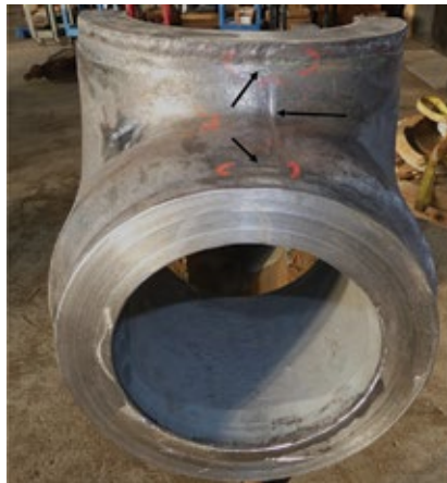
6. Tee suffered a through-wall crack at the crotch position on one side and another partially through-wall crack on the other
