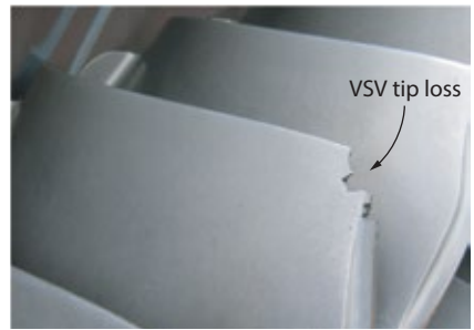
Borescope inspection for VSV tip loss
