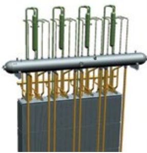
Secondary steam separation in bottles outside drum
