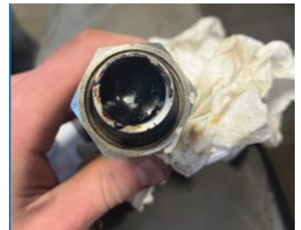
Coke prevents fuel flow after burning diesel oil
