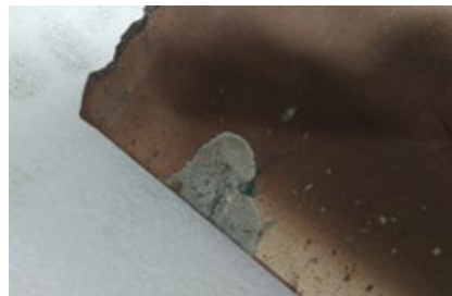
Impact damage/cracking to turbine S2B airfoils
