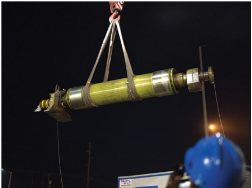
7. 7A6 generator field on its way to MD&A St. Louis for a full rewind
