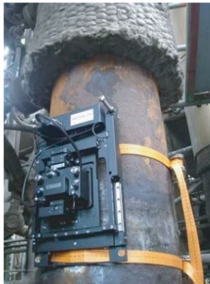
3. Portable scanning force microscope on vertical pipe
