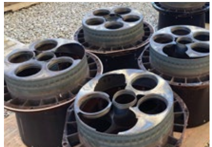
Failed combustor end caps
