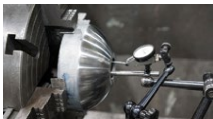
6. Main steam valves for the A10 steam turbine were inspected and repaired in MD&A's St. Louis facility
