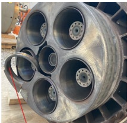
Damage caused by acoustic dynamics
