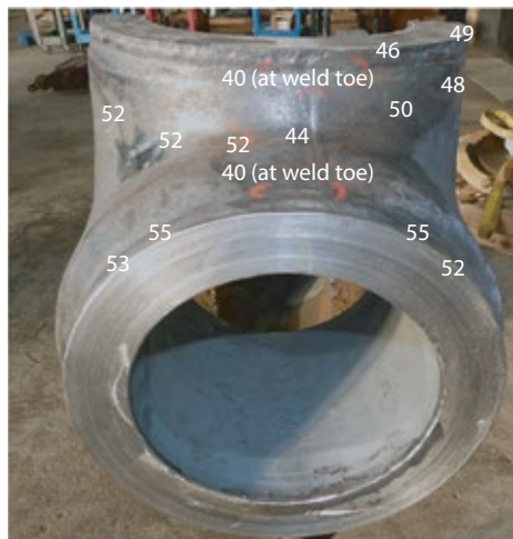
3. As produced tee wall thicknesses are in millimeters. Note the short leg lengths for both the run and branch
