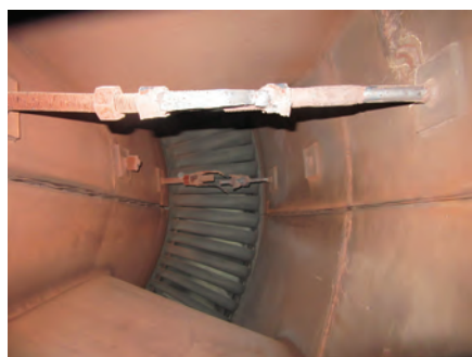
1. Inspections are critical to managing exhaust-frame health. Examples of findings: Parting-joint separation and cracked shop welds are in evidence at left, along with turnbuckles remaining from a previous outage; borescope image in center reveals cracked airfoil internals; cracked shop welds and previous repair are at right
