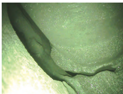
1. Inspections are critical to managing exhaust-frame health. Examples of findings: Parting-joint separation and cracked shop welds are in evidence at left, along with turnbuckles remaining from a previous outage; borescope image in center reveals cracked airfoil internals; cracked shop welds and previous repair are at right
