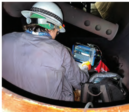
GS5. PAUT is performed to size the cracks and determine the depth
