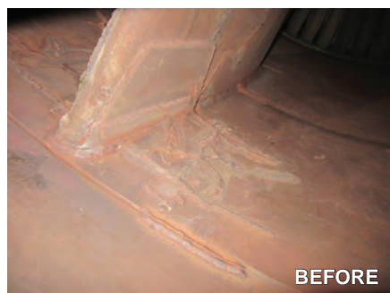
1. Inspections are critical to managing exhaust-frame health. Examples of findings: Parting-joint separation and cracked shop welds are in evidence at left, along with turnbuckles remaining from a previous outage; borescope image in center reveals cracked airfoil internals; cracked shop welds and previous repair are at right
