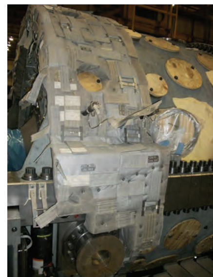
4. Arnold insulation system enables 60–80% of blankets to remain in place during outages, cutting reinstallation time and cost while allowing rapid turbine access by removing only essential sections like split lines, bolts, flanges, and jack rings
