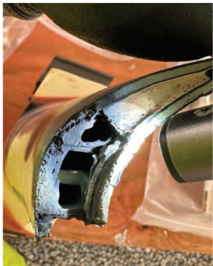
Leading-edge burnup on S1B air-foils prompted a change in the tip-cap replacement process and follow-on inspection
