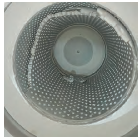
11. HP bypass valve damage due to water impingement
