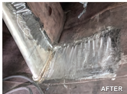
2. An advantage of partial, targeted repairs is the ability to get your plant back in service quickly. Photos stacked at left show an airfoil crack and past repair at the top and IPS upgraded repair at the bottom. An airfoil internal crack is at the top right and IPS internal repair below
