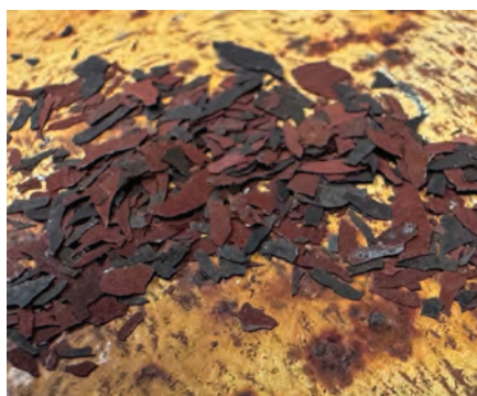
5. Iron-oxide debris causes severe damage to blades and vanes, resulting in clogged cooling paths, erosion of coatings, and costly off-cycle replacements
