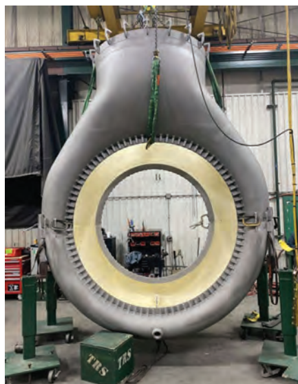
7. Hot gas casing by refurbished by TRS in partnership with HTS
