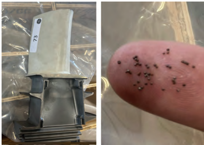
New first-stage blades were delivered with shot-peening grit inside cooling channels. Air flush was ineffective
