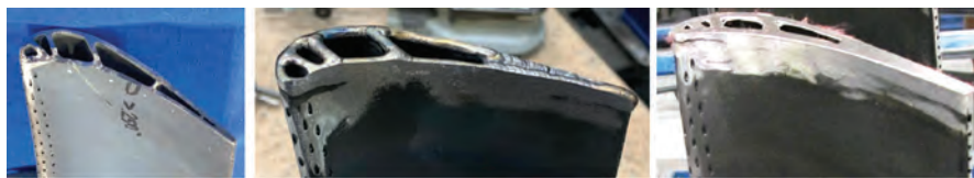
MD&A: Blade tip rejuvenation of 7FA.04 first-stage blades involves removing cracks and damage, welding with Rene N4 material, and machining to prepare for new tip cap installation—restoring structural integrity and extending service life
