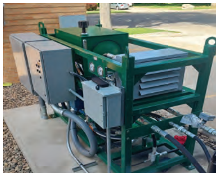
2. Hydraulic motor starter package, comprising an electric motor and variable displacement piston pump, replaced an aged diesel-based skid, for which parts and services were unavailable
