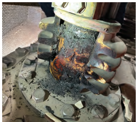
Responding to a low casing-pressure alarm on a hydrogen-cooled generator, plant personnel increased gas pressure. Hydrogen consumption increased dramatically over the next few weeks. Cause was a failed bushing
