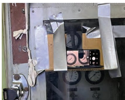
3. Graph of exhaust temperature and speed was created by converting iPhone recordings of analog readouts into troubleshooting data
