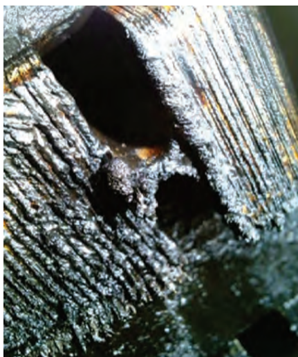
MD&A: Greasing, contamination, and step iron damage was discovered after a challenging in-situ robotic inspection of an early vintage 7FH2 generator
