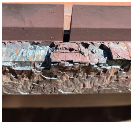
Debris from oxidation flaking of the inner support ring for the first-stage nozzles ends up downstream
