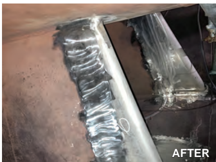
2. An advantage of partial, targeted repairs is the ability to get your plant back in service quickly. Photos stacked at left show an airfoil crack and past repair at the top and IPS upgraded repair at the bottom. An airfoil internal crack is at the top right and IPS internal repair below
