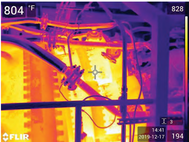
Elevated compartment temperature issue (left) attributed to loose DLN 2.6+ combustion-can bolts (right) was resolved by replacing carbon-steel washers with ones of higher yield strength and increased temperature resistance (TIL-2484)
