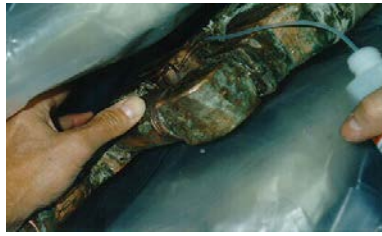
Figure 7-34. Testing for Water Leak using Bubble Solution
