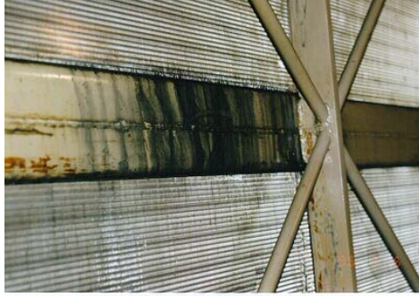
Figure 6-36. Wear Products from Vibration of Cooler Components
