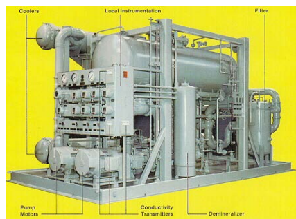
Figure 6-71. Typical Large External Pumping Unit for Liquid Cooled Generator (Westinghouse)
