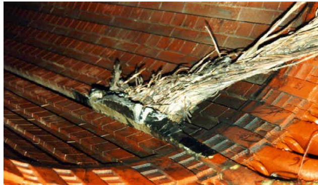
Figure 2-13. Stator Bar Thrown from Slot by Sudden Short Circuit Force
