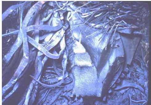
Figure 2-32. Results of Field Forging Fracture
