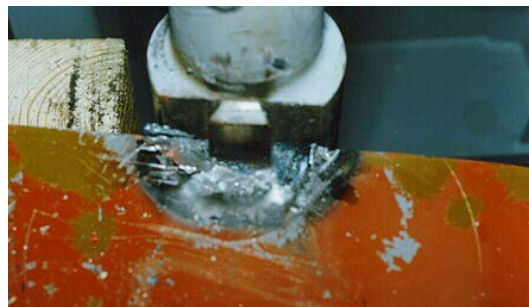
Figure 6-33. Keybar Burning Due to Over-flux Incident
