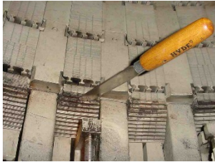
Figure 4-47. Knife check of local core looseness
