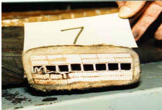
Figure 2-14. Stator Bar Ventilation Ducts Collapsed by Armature Current Forces of a Sudden Short Circuit
