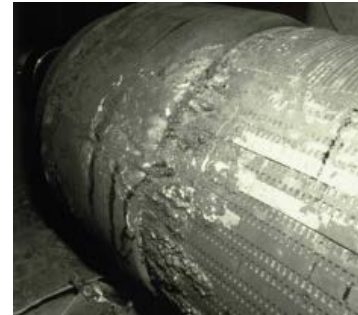
Figure 4-61. Melted field and retaining ring forgings
