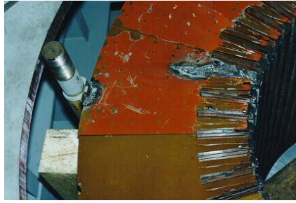
Figure 6-34. Melted Keybar and Tooth Areas Due to Over-flux Incident
