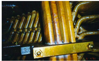
Figure 6-19. Dust Generation from Connection Ring Vibration
