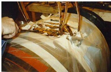
Figure 8-48. Partial Rewind of Field Winding
