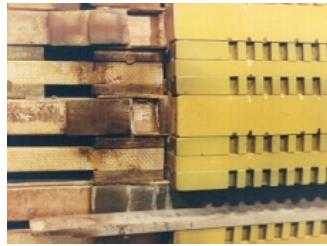
Figure 4-57. Cracked top turn. Root cause: Non-body-mounted retaining ring.
