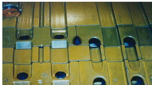
Figure 6-51. Field Ventilation Holes, Direct Cooled
