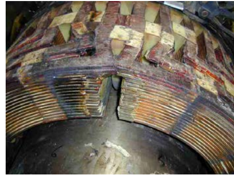
Photo 30. Badly over-temperature and distorted endwinding.
