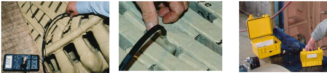
Figure 7-37a,b&c. Capacitance and Wet Insulation Testing (WID) Testing for Wet Insulation
