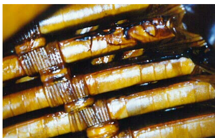
Figure 6-22. Deposit Resulting from Partial discharge Field Acting on Lubrication Oil Vapor
