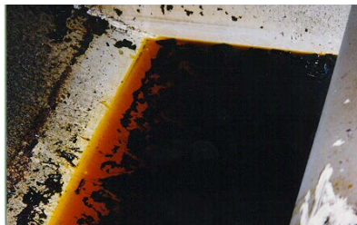
Figure 6-35. Oil Accumulation in Stator Frame
