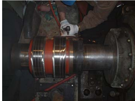
Figure 8-46. Re-grooving collector rings. (Cutsworth Products/Services)
