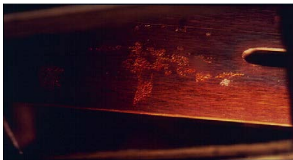
Figure 6-52. Copper Dust Generation Site on Field Turn
