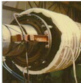
Figure 8-35 & Figure 8-36. Retaining Ring Removal Equipment, Induction and Gas Ring Heating
