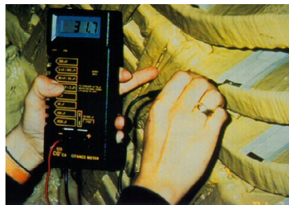
Figure 7-32. Bar Insulation Capacitance Testing
