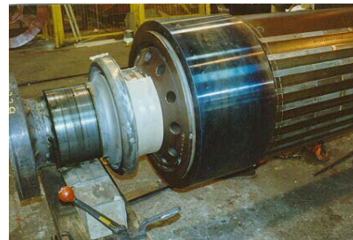
Figure 8-37 & Figure 8-38. Retaining Rings Showing Normal Heating (Left) and Overheating Pattern (Right)
