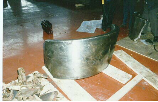
Figure 4-20. Section of Retaining Ring which Failed in Service Due to Stress Corrosion Cracking
