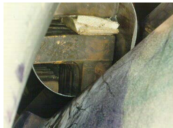
Figure 6-12. & Figure 6-13. Field Winding Inspection with Mirror and Direct View
