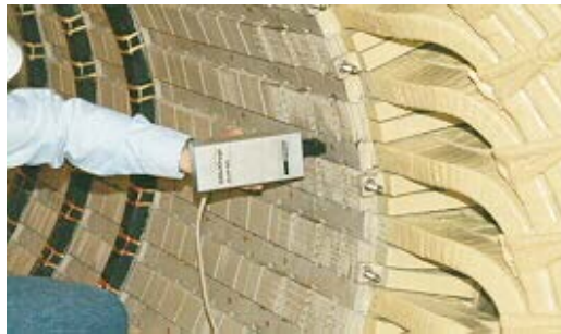
Figure 7-12. Hand-held Stator Wedge Mechanical Wedge Tapper
