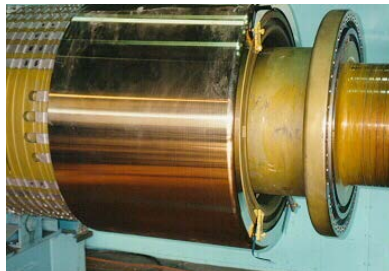
Figure 8-37 & Figure 8-38. Retaining Rings Showing Normal Heating (Left) and Overheating Pattern (Right)
