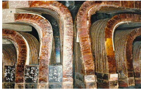
Figure 4-15. Field Winding Turn Distortion
