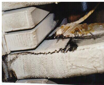
Figure 8-26 & Figure 8-27. High Potential Test Partial discharge Damage to Stator End Winding
