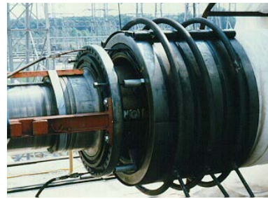
Figure 8-35 & Figure 8-36. Retaining Ring Removal Equipment, Induction and Gas Ring Heating
