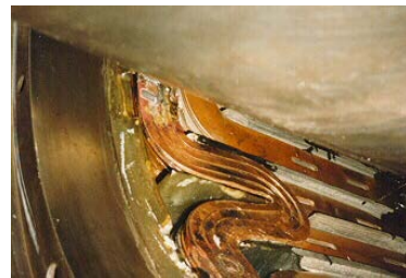
Figure 6-12. & Figure 6-13. Field Winding Inspection with Mirror and Direct View
