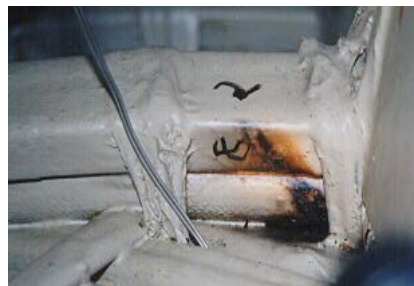
Figure 8-26 & Figure 8-27. High Potential Test Partial discharge Damage to Stator End Winding
