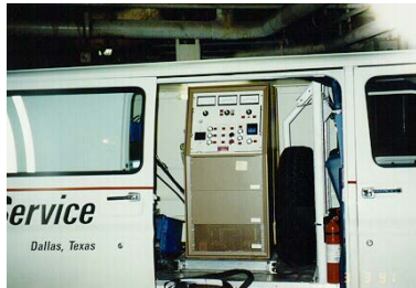
Figure 7-4. Van Mounted 0.1Hz High Potential Test Equipment
