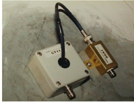
Figure 5-17. Radio Frequency Current Transformer on Lead from Adwel 1000 pF Line Pickup (ABB)
