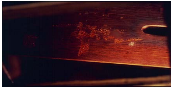
Figure 2-39. Site of Abrasion of Copper Conductor Resulting in “Copper Dust”
