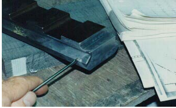
Figure 2-34. Wedge Body Burn Resulting from Rotor Body Current
