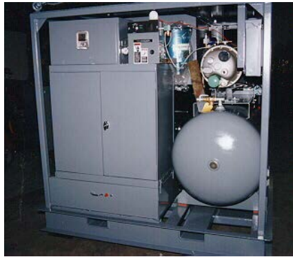
Figure 7-29. Test Skid for Removing and Drying Water from Stator Windings (General Electric)
