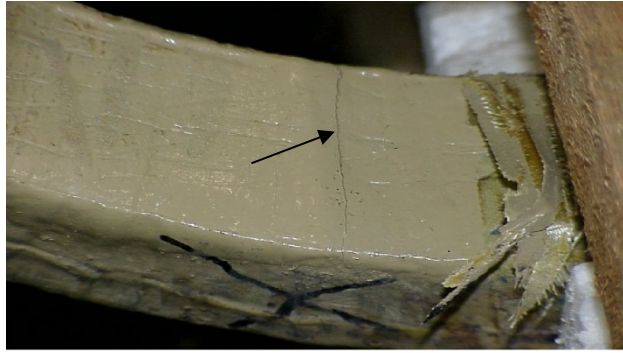
Figure 2-22. Severe crack in stator bar groundwall insulation.
