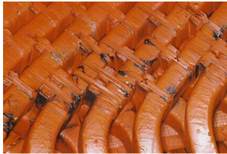
Figure 4-1. Stator End Winding Vibration
