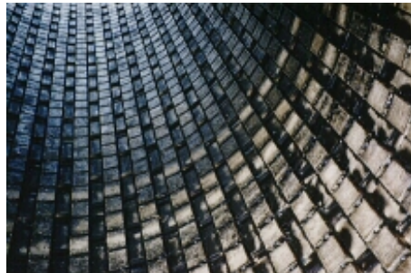
Figure 4-46. Heavily contaminated stator
