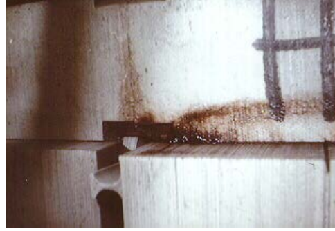
Figure 6-8 & Figure 6-9. Robot Camera View of Stator Bar Vibration and Core
