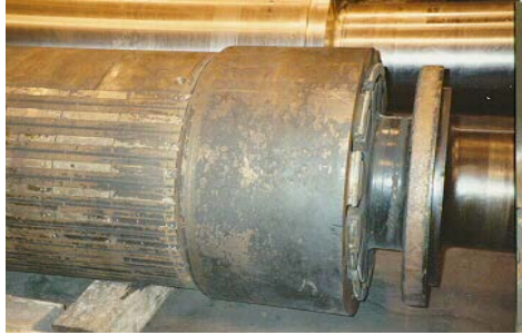
Figure 6-60. Heavily Contaminated and Rusted Field
