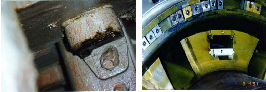
Figure 6-38 & Figure 6-39. Fretting Winding Support and Field Balance Weight Locks
