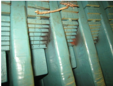
Figure 2-7. Deposit likely due to side vibration of the bar in the slot
