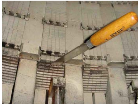
Figure 6-31. Use of Knife to Evaluate Core Looseness
