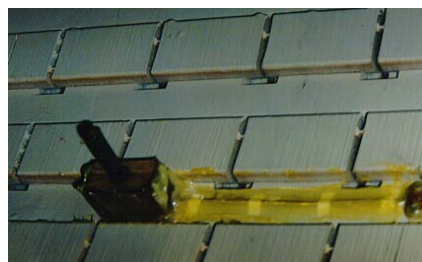
Figure 7-21. Assembled Field Turn Short Flux Probe
