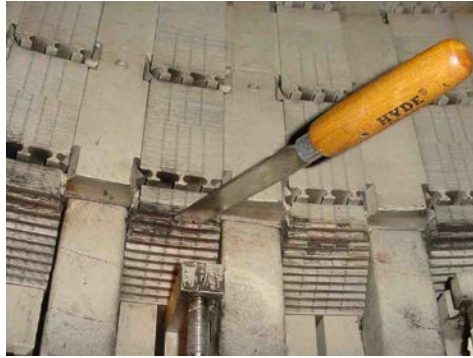
Figure 4-23. Similar loose core laminations.
