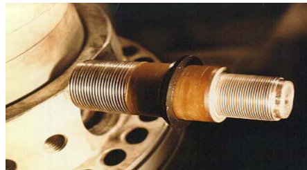
Figure 8-43. Stud Removed from Collector Connections
