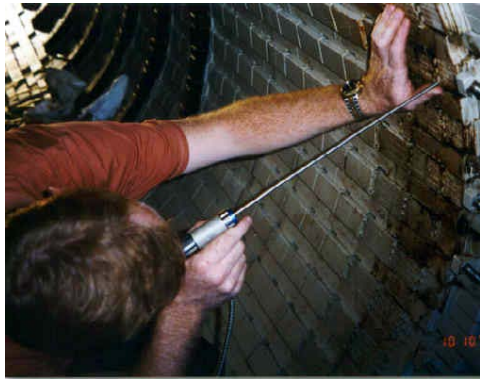
Figure 6-17 & Figure 6-18. Inspection for Stator Bar Slot Vibration by Borescope and Flashlight
