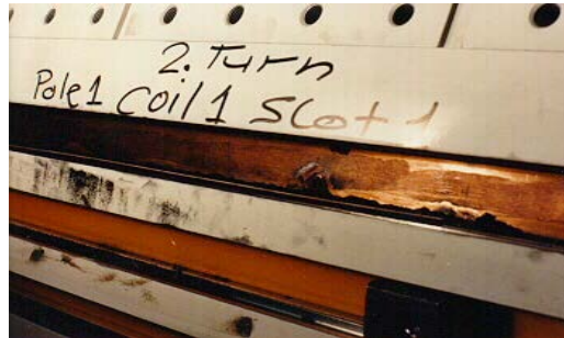
Figure 4-14. Ground Current Damage to Copper Turn and Field Forging from Broken Top Turn
