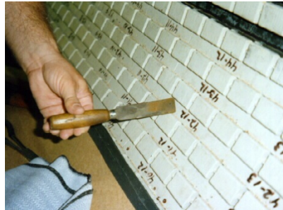
Figure 7-27. Knife Test of Core Tightness
