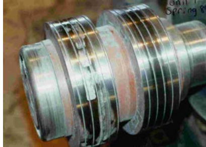
Figure 2-47. Patterning of brush wear on collector.
