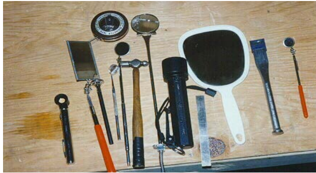
Figure 6-3. Typical Hand Tools for Generator Inspection, Courtesy Enoch Silva, ES Consulting
