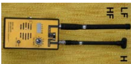
Figure 5-22. Hand-held PD search instrument.
