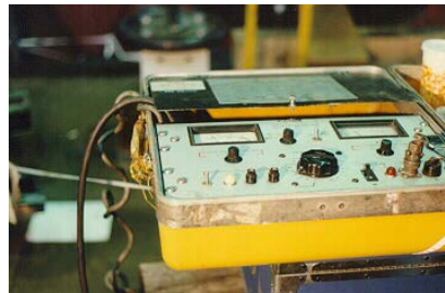
Figure 7-5. DC High potential Equipment
