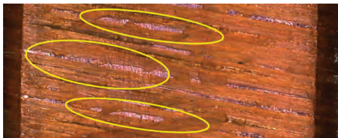
14. Original magnified stator bar strand, left, pinpoints weaknesses compared to upgraded replacement
