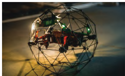
4. Flyability Elios 2 is equipped with an advanced onboard lighting system and 4K cameras
