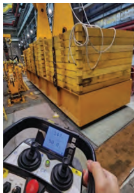
2. Trial lifts of critical components (GT rotor at left; exhaust casing at right) are an important part of pre-outage training
