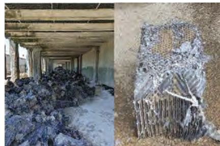
3. Deposition of calcium silicate inside the media dramatically degraded cooling-tower performance
