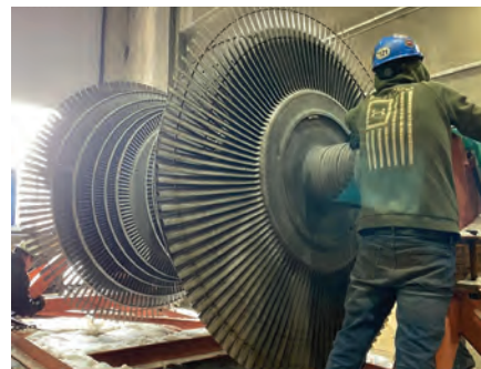
8. Salvageable D5 LP rotor was found by combing through a list of units affected by a TIL issued in 1981. Rotor was then repaired and refurbished and installed in a 1961-vintage D5 ST/G which suffered a significant crack of the L-0 wheel at the fillet transition from shaft to rotor hub
