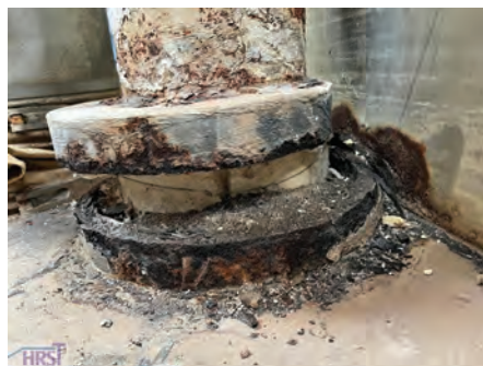
5. Corrosion under insulation (CUI), which has forced many plants into an outage, is getting more attention with CCGT units over 20 years old
