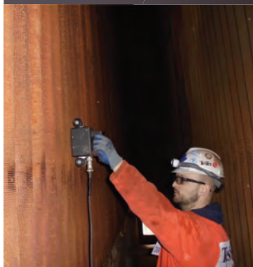
Through Fin Tube Scanning for Wall Thinning
