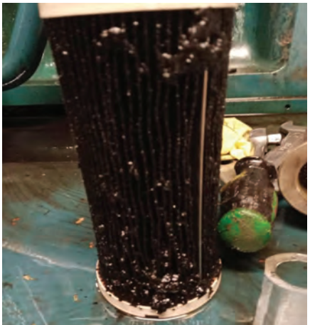
4. Fouled fuel filters adversely affect plant availability and engine reliability while adding to the time, effort, and cost of operation and maintenance
