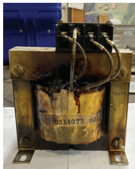
A1T instrument transformer suffered damage shortly after unit restart
