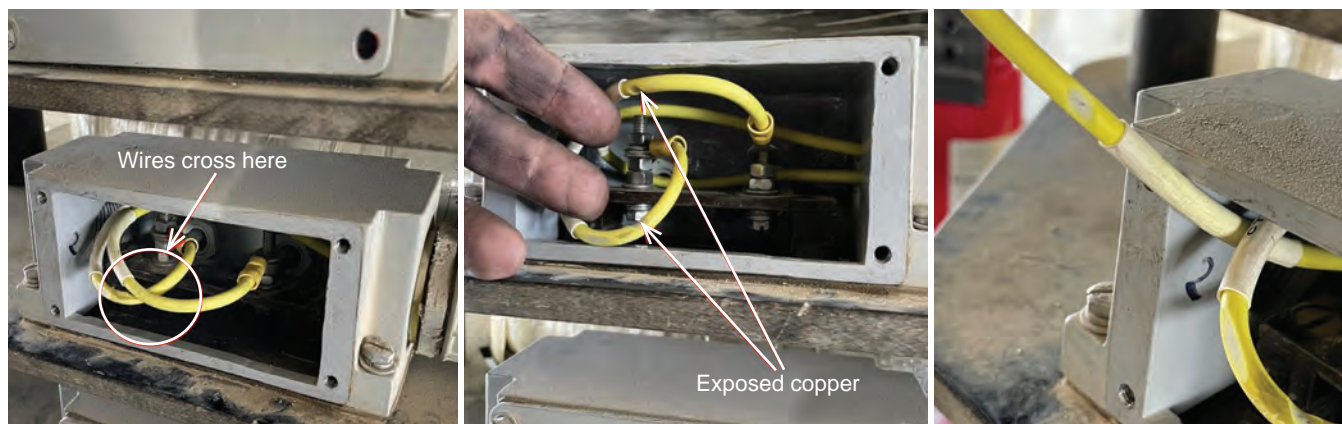
11. Ground fault and worn insulation were found where two CT wires crossed and touched (left and middle). A similar situation was found in another unit (right)
