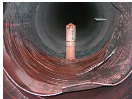
1. Thermal liner damage from leaking spray water
