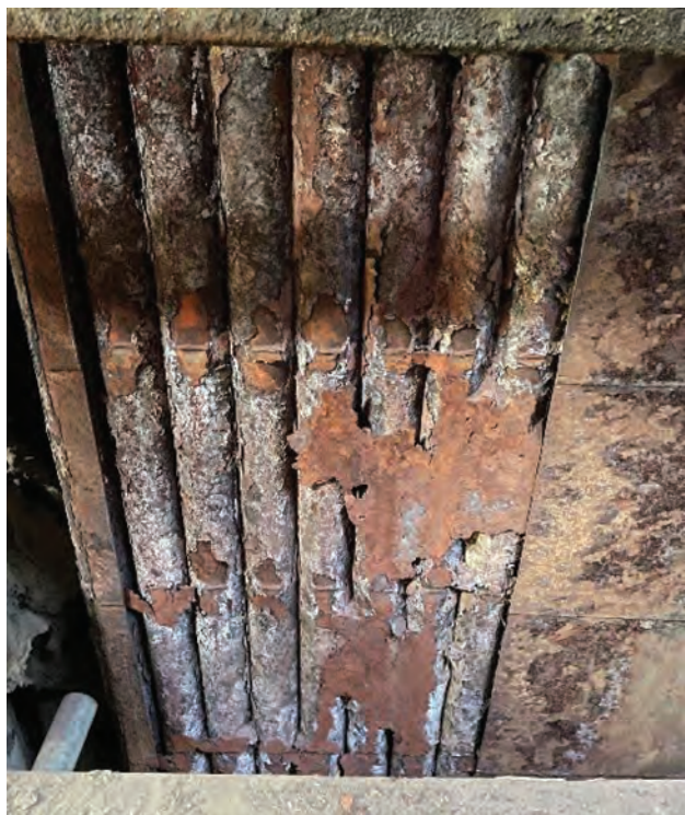
6. As-found tube corrosion condition after casing removal
