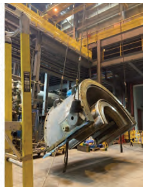
2. Trial lifts of critical components (GT rotor at left; exhaust casing at right) are an important part of pre-outage training
