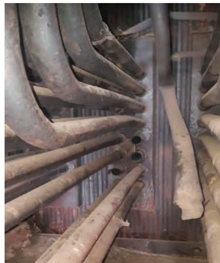
5. Tube failure at seal box around boiler wall penetration
