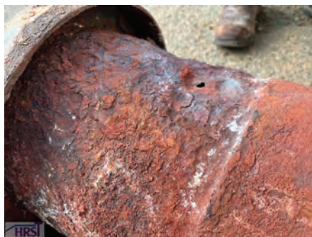
5. Corrosion under insulation (CUI), which has forced many plants into an outage, is getting more attention with CCGT units over 20 years old
