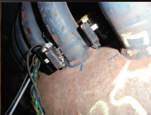
Tube to Header Weld Examination for Cracking
